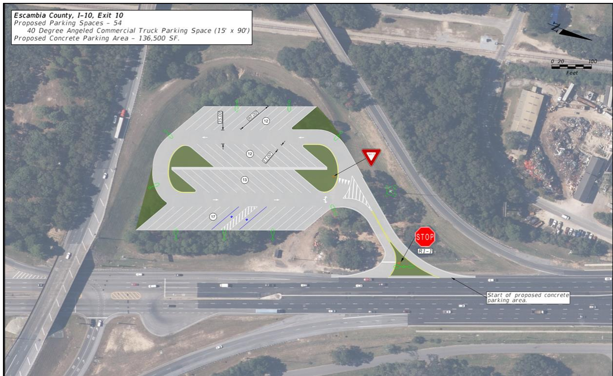
Figure 22: Escambia County Exit 10 Interchange Infield Concept Design
