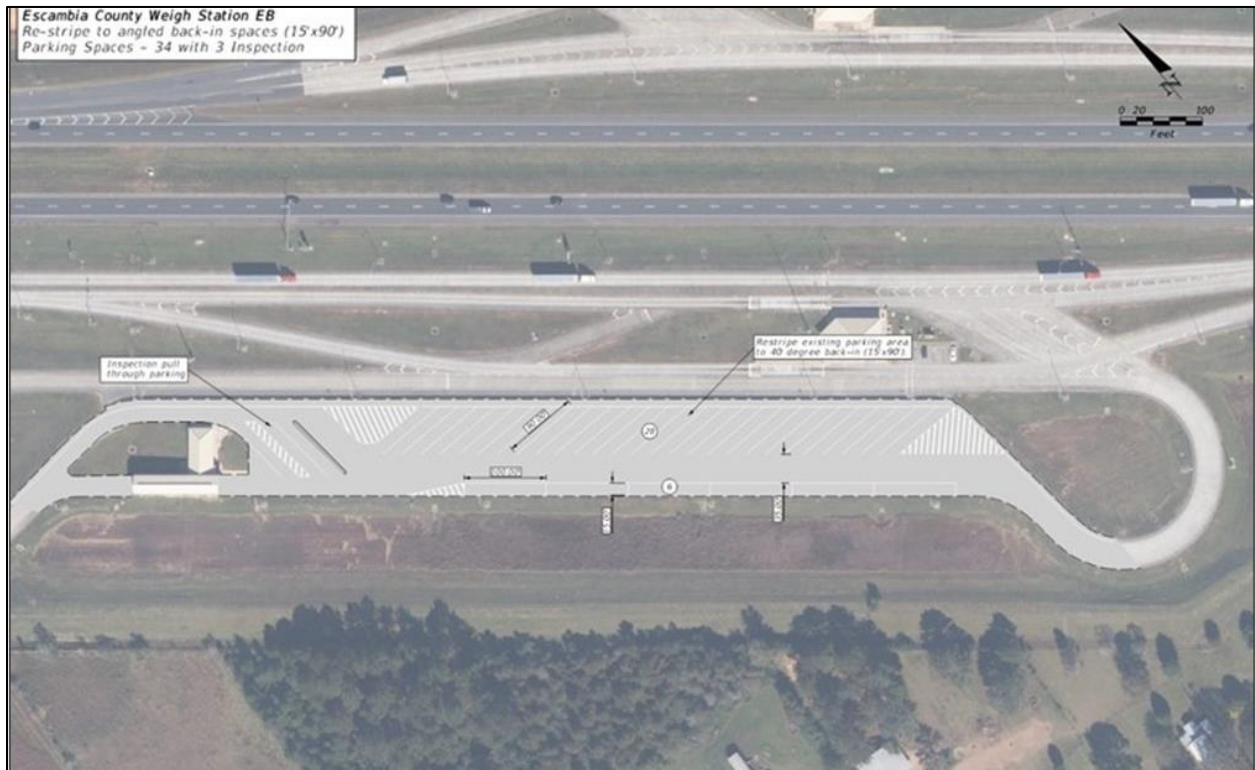
Figure 19: Escambia County Westbound Weigh Station Concept Design
