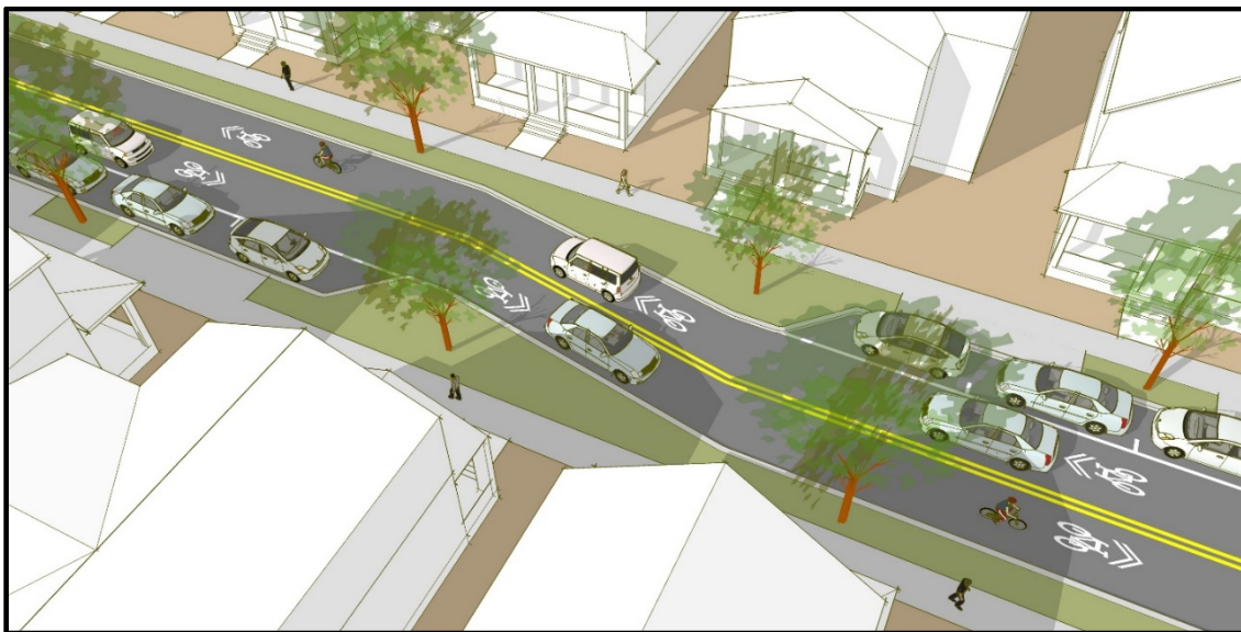
Figure 202.3.1 Concept Sketch - Midblock Chicane
