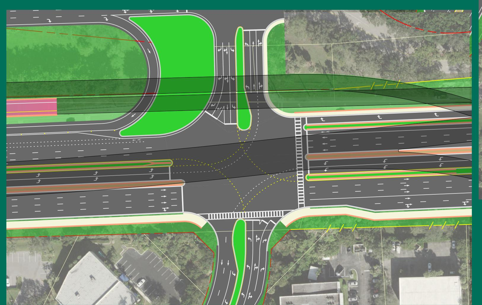
Note: Non-restrictive Intersection Option provides poorer signal operation than the restictive intersction shown.
