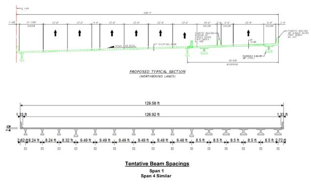
Figure 3-6 Widening / Rehabilitation – Tentative Beam Spacings
