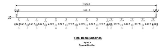
Figure 3-7 Widening / Rehabilitation – Final Beam Spacings
