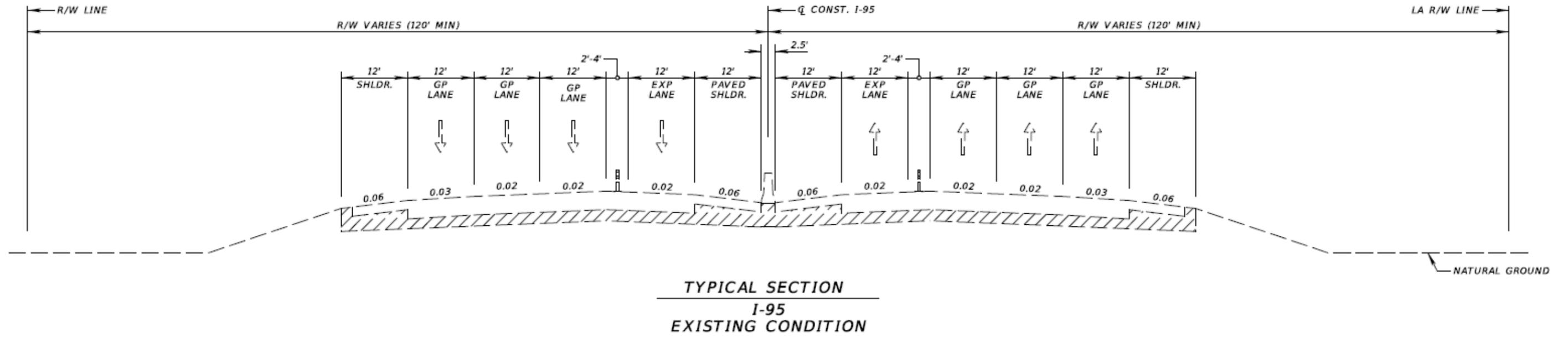
Figure 2-2 Existing Typical Section – I-95
