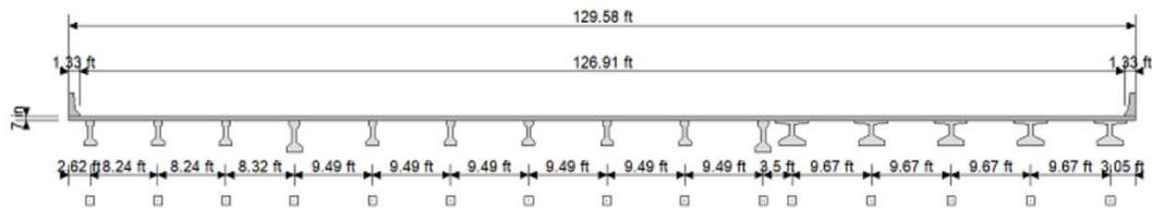
Figure 3-7 Widening / Rehabilitation – Final Beam Spacings
