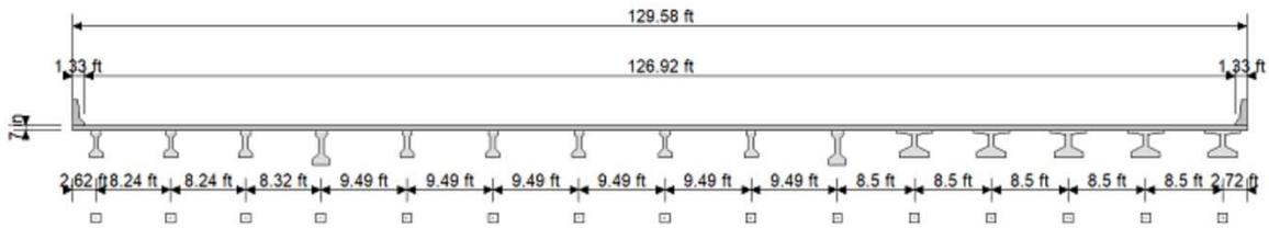
Figure 3-6 Widening / Rehabilitation – Tentative Beam Spacings
