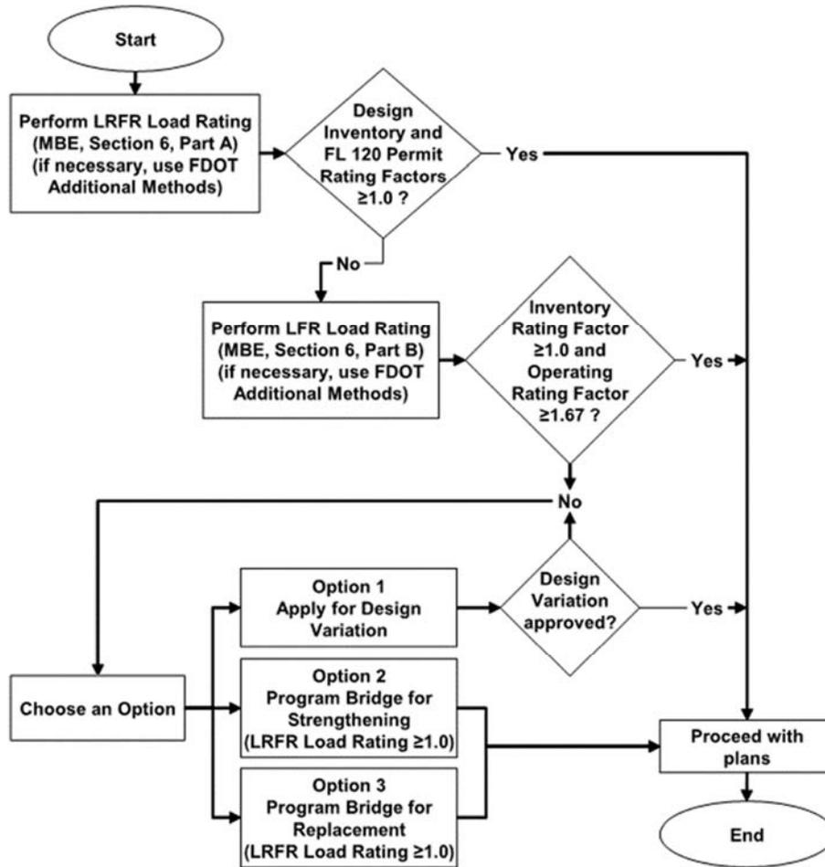
Figure 3-5 Widening / Rehabilitation Load Rating Flow Chart
