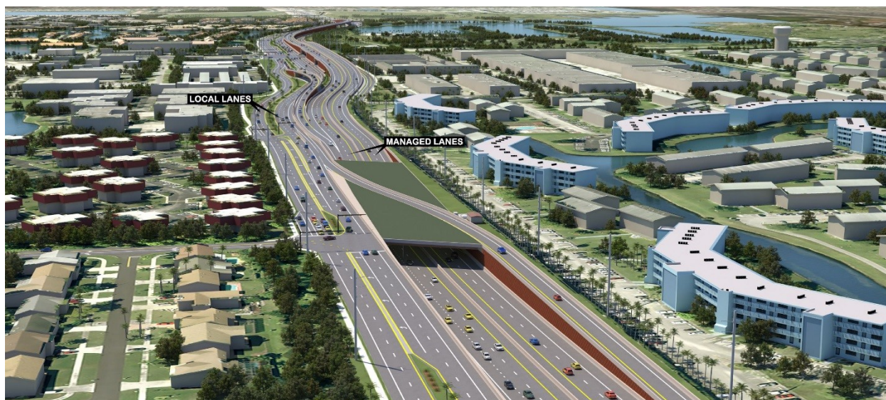
Figure 4.1.6: Partial Depressed – Depressed Eastbound & Westbound Managed Lanes Alternative
