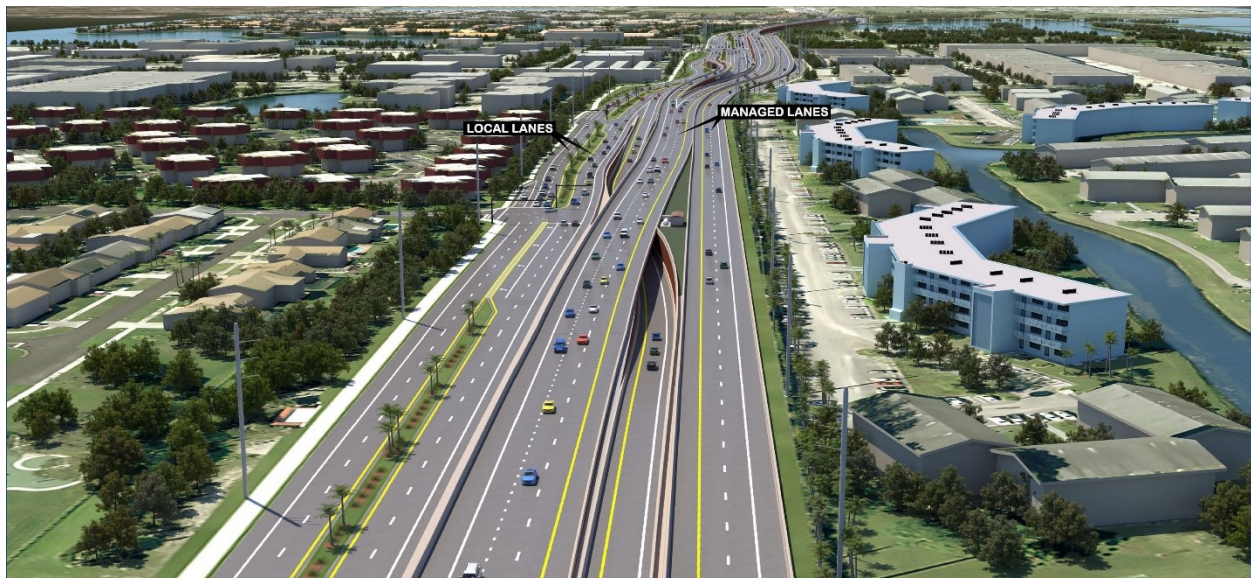
Figure 4.1.4: Partial Depressed – Depressed Westbound Exit Ramp Alternative
