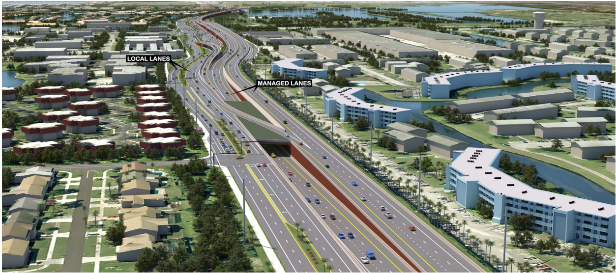
Figure 4.6.19: Depressed Eastbound Managed Lanes Looking West
