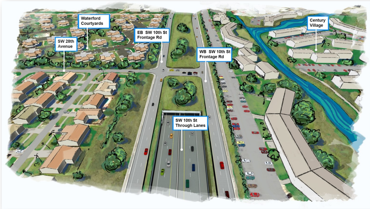
Figure 4.1.6: Conceptual Depressed Section from Broward MPO COAT Study
