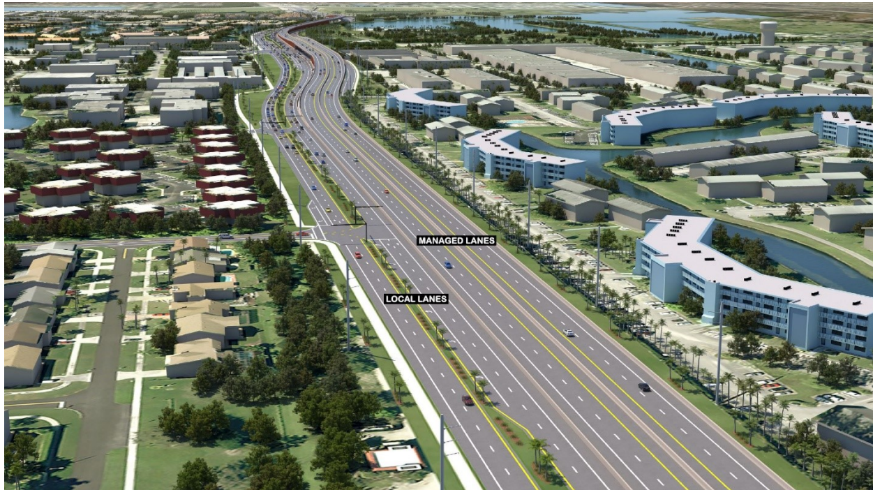
Figure 1.4.7: Non-Depressed/No Managed Lane Access Alternative
