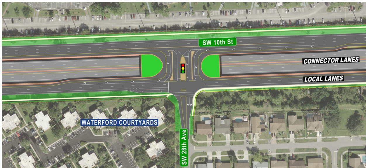
Figure 4.5.7: SW 28 th Avenue Intersection with Center Alternative
