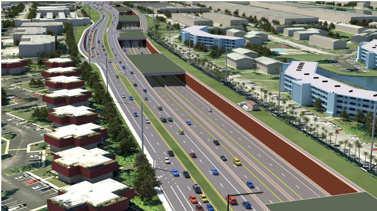
Figure 1.4.3: Full Depressed Alternative
