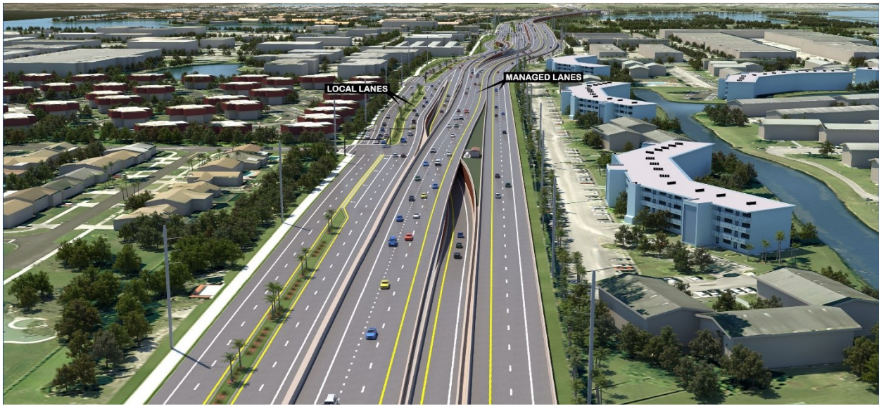
Figure 1.4.4: Partial Depressed – Depressed Westbound Exit Ramp Alternative
