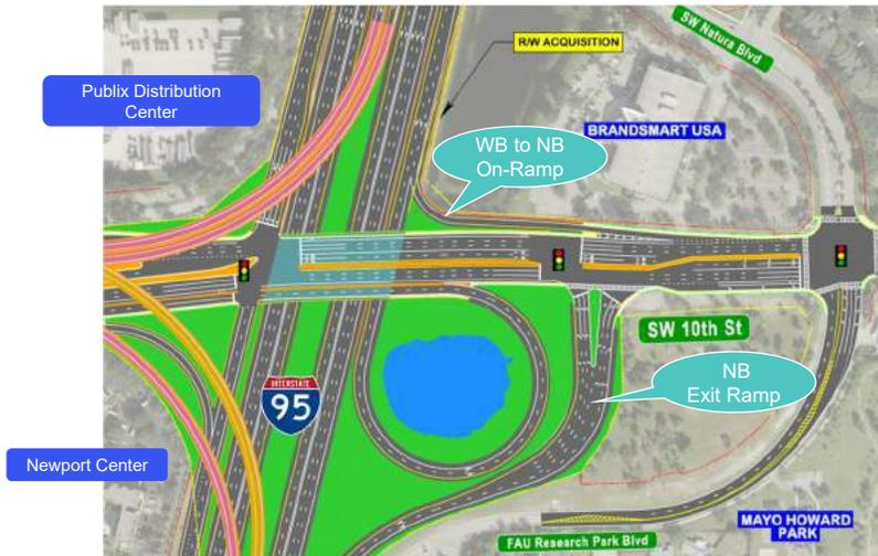
Intersection improvements at the SW 10<sup>th</sup> Street interchange include expanding the NB exit ramp to accommodate triple left and triple right turns and providing a free-flow right turn for the WB SW 10<sup>th</sup> Street to NB I-95 entrance ramp.
