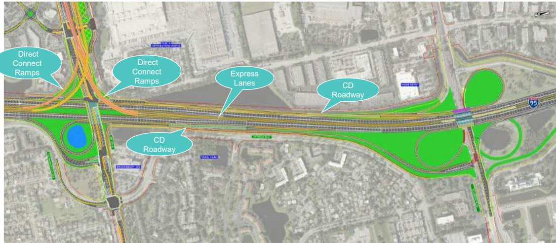
The improvements being considered along I-95 include direct connections from the SW 10<sup>th</sup> Street managed lanes to I-95 SB and NB express lanes. Will be adding 1 EL in each direction and a NB separate parallel roadway called a collector distributor or CD roadway combining both of the on-ramps and separating the traffic entering I-95 from the traffic exiting at Hillsboro Blvd. A similar CD roadway is also proposed for the SB traffic.
