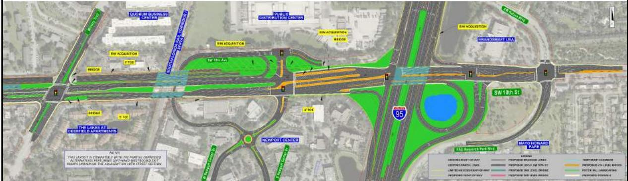
Improvements along local SW 10<sup>th</sup> Street include sidewalks and 7 foot buffered bike lanes on both sides. A roundabout is being evaluated at the intersection of east and west Newport Drive.
