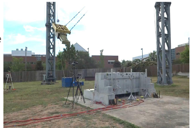
An impactor has been raised to 15-foot drop height prior to release.
