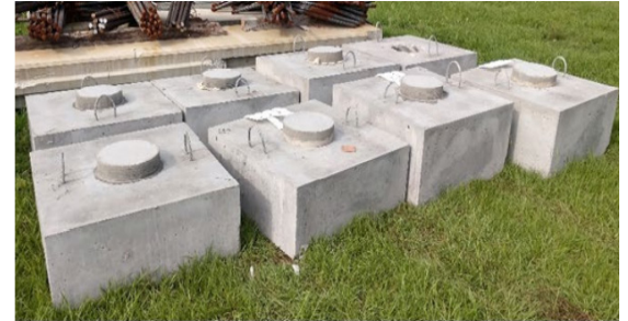
Florida International University researchers used these specimens to test shear friction capacity for precast pile caps and precast piles that do not have steel crossing the interface.
