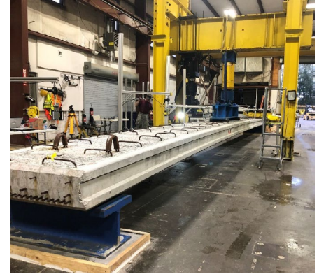
Figure 1. Slab with higher camber than expected.
