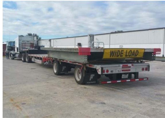
Figure 23 – Completed Deck Unit Shipping
