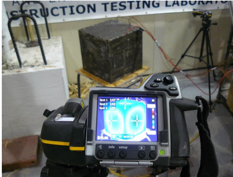
Figure A-15: Camera 2 simultaneously monitored three surface of the specimen
