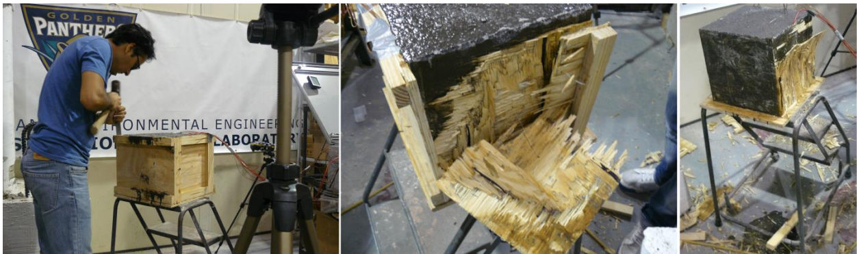
Figure A-10: Formwork removal
