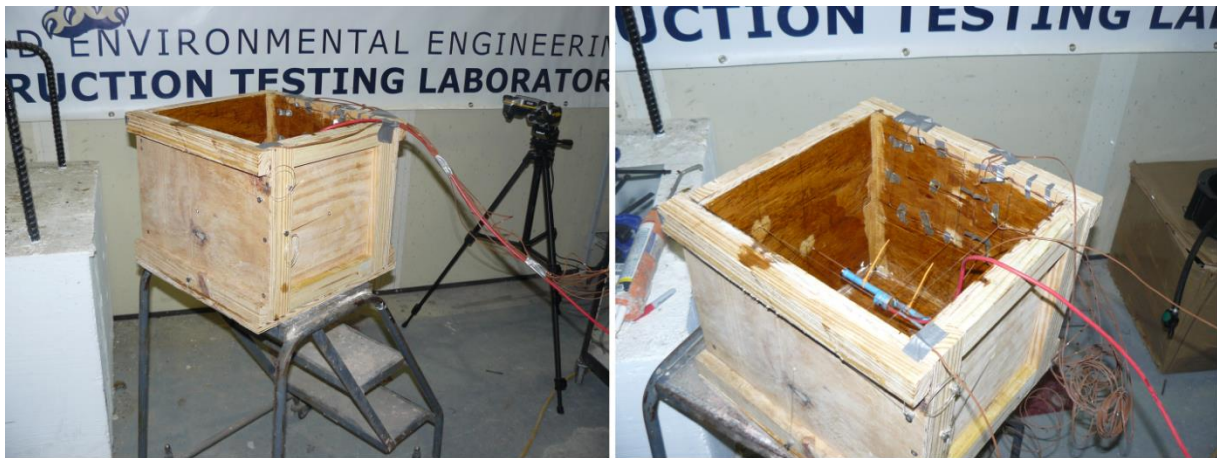
Figure A-3: Six thermocouple sensors were embedded in the neighborhood of the surface shot by the thermography Camera 1
