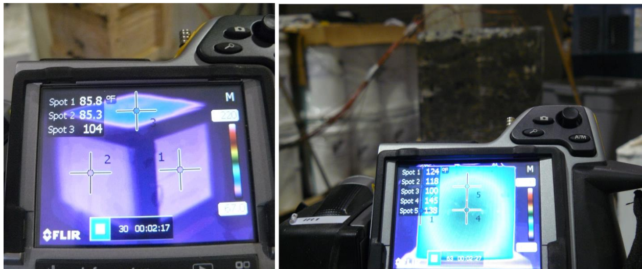
Figure A-16: Three spot-meters set for Camera 2 (left), and five spot-meters for Camera 1 (right)
