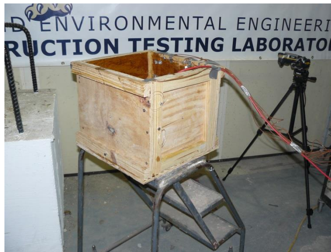
Figure A-1: Formwork for E3HP epoxy grout system
