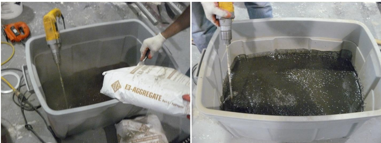
Figure A-8: The part C (aggregate) added and mixed for 5 minutes until the aggregate was completely wetted out
