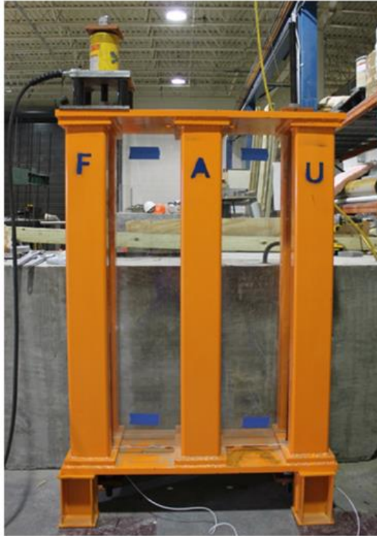
Figure 4.19 Two CFCC Tendons Positioned in the Test Frame for Application of Tension
