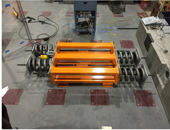
Figure 4.31 Loaded Creep Rupture Testing Frame
