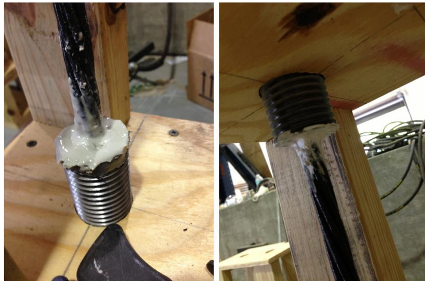
Figure 4.5 Epoxy Filler in Curing Process
