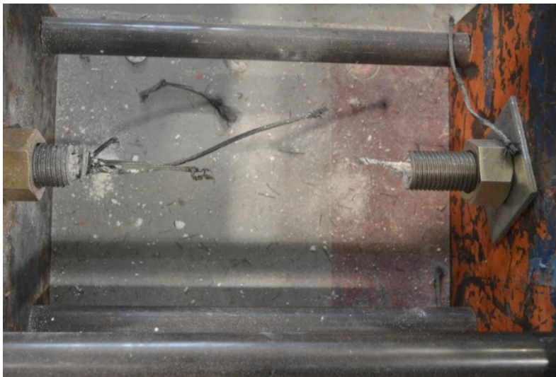
Figure 4.12 Fragments of the Ruptured CFCC Tendons after Failure
