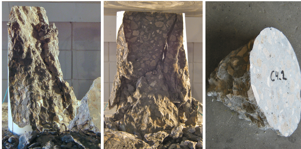
(a) Cone on top end (b) Cone on both ends (c) Preserved surface
