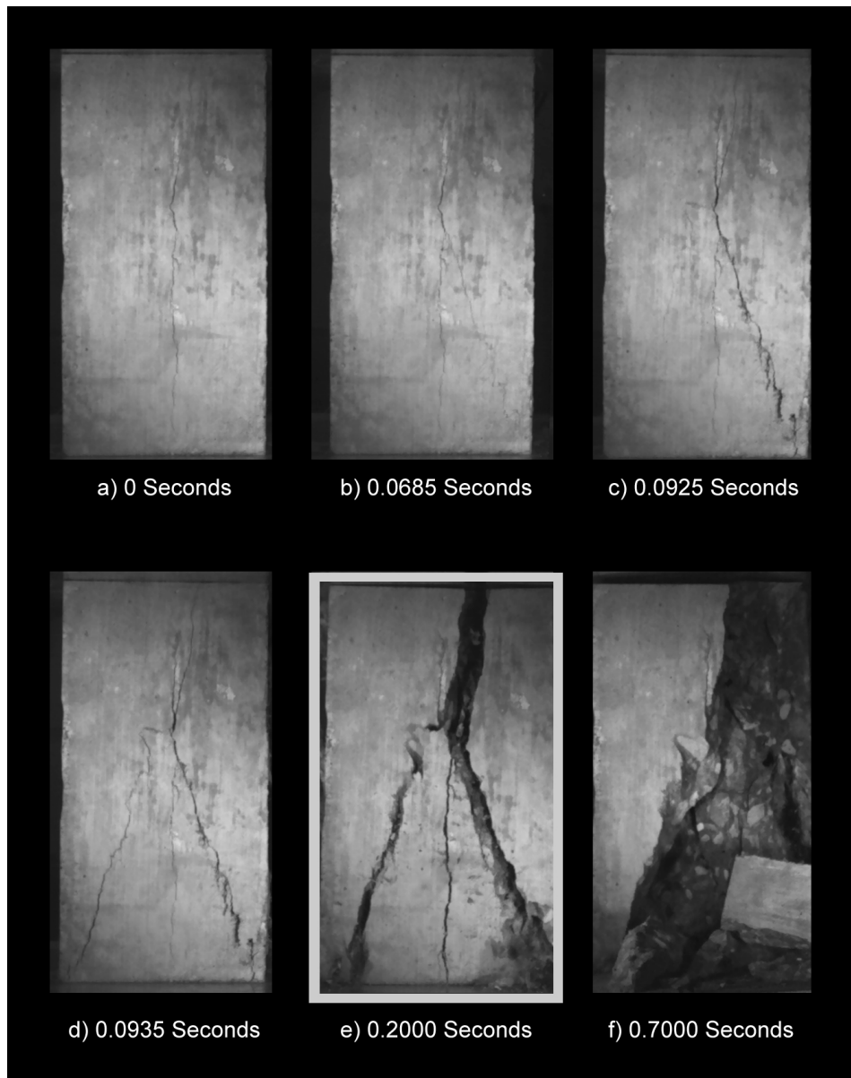
Figure 4.15: Column failure under regular friction
