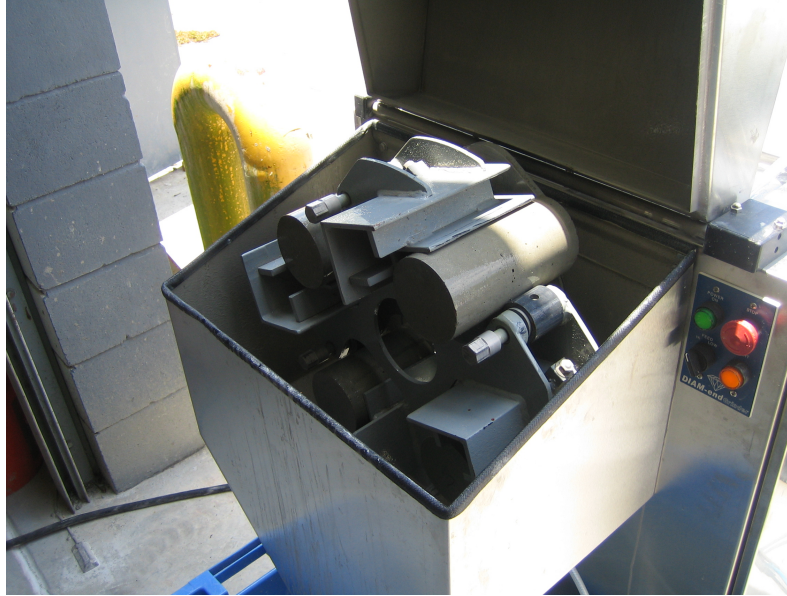
Figure 3.6: End grinder for concrete cylinder
