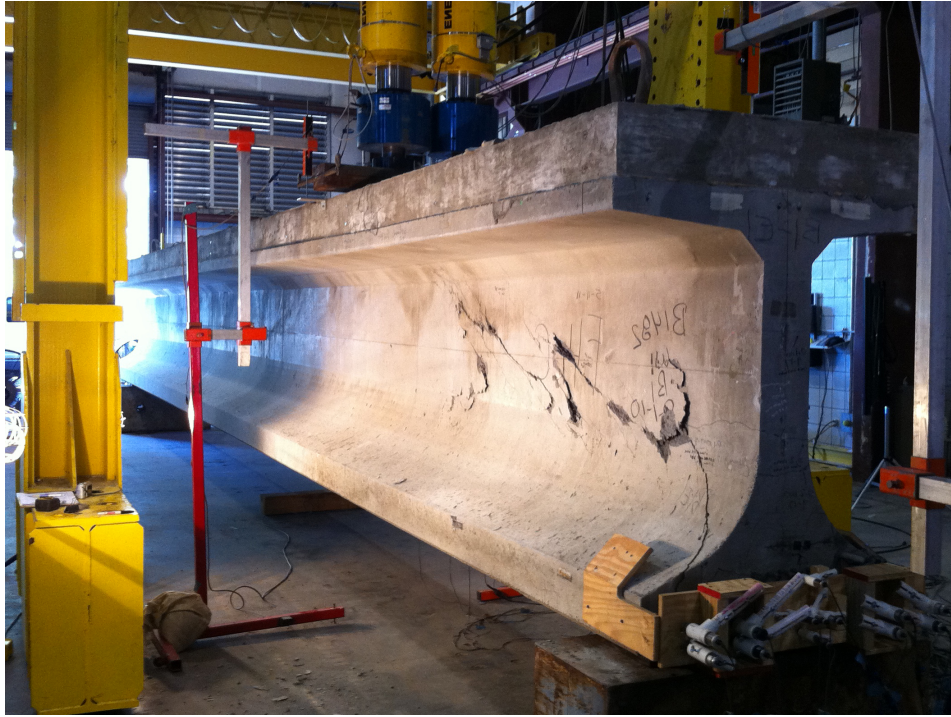
Figure 1.2: Concrete failure in structural testing
