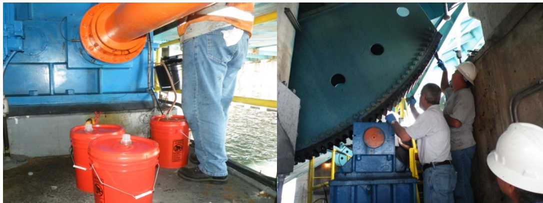
Figure 3: Damage tests (mechanical): removal of gearbox oil (left) and removal of the open gear grease (right)
