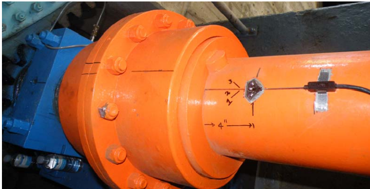
Figure 25: Strain rosette on the drive shaft
