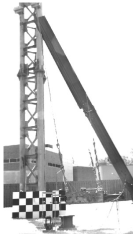
Figure 10-21. Oblique impact from high-speed camera (where t = 0 \text{ sec.} indicates contact between post and pendulum) for experiment T-25-2
