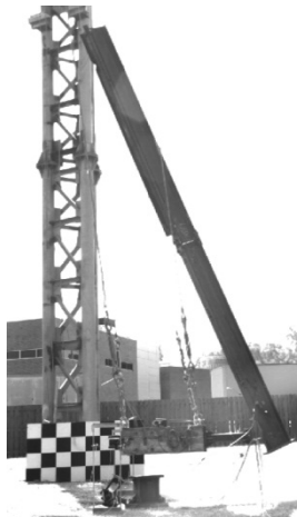
Figure 10-21. Oblique impact from high-speed camera (where t = 0 \text{ sec.} indicates contact between post and pendulum) for experiment T-25-2
