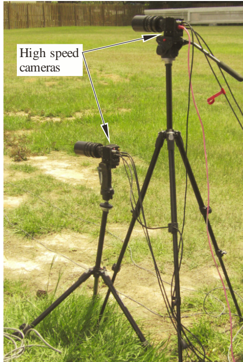
Figure 10-15. High-speed digital video cameras
