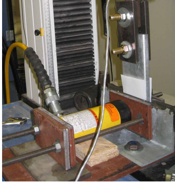
Figure 5-5. Experimental setup with Teflon sheets installed
