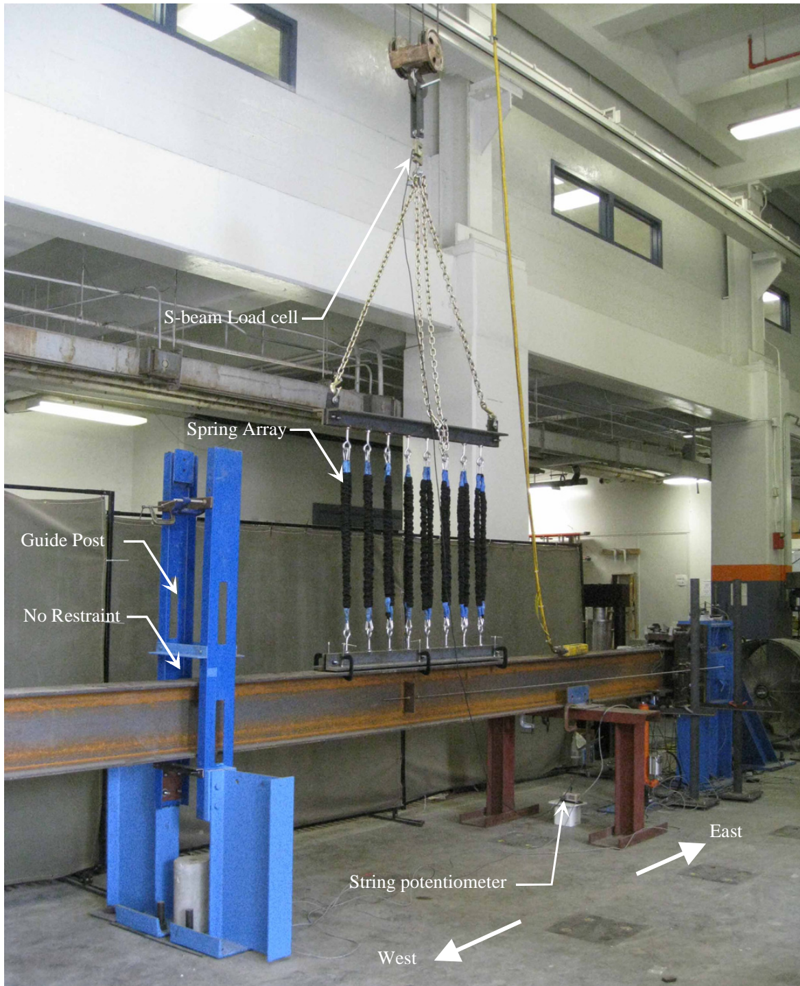
Figure 7-6. View from west side of the static test setup
