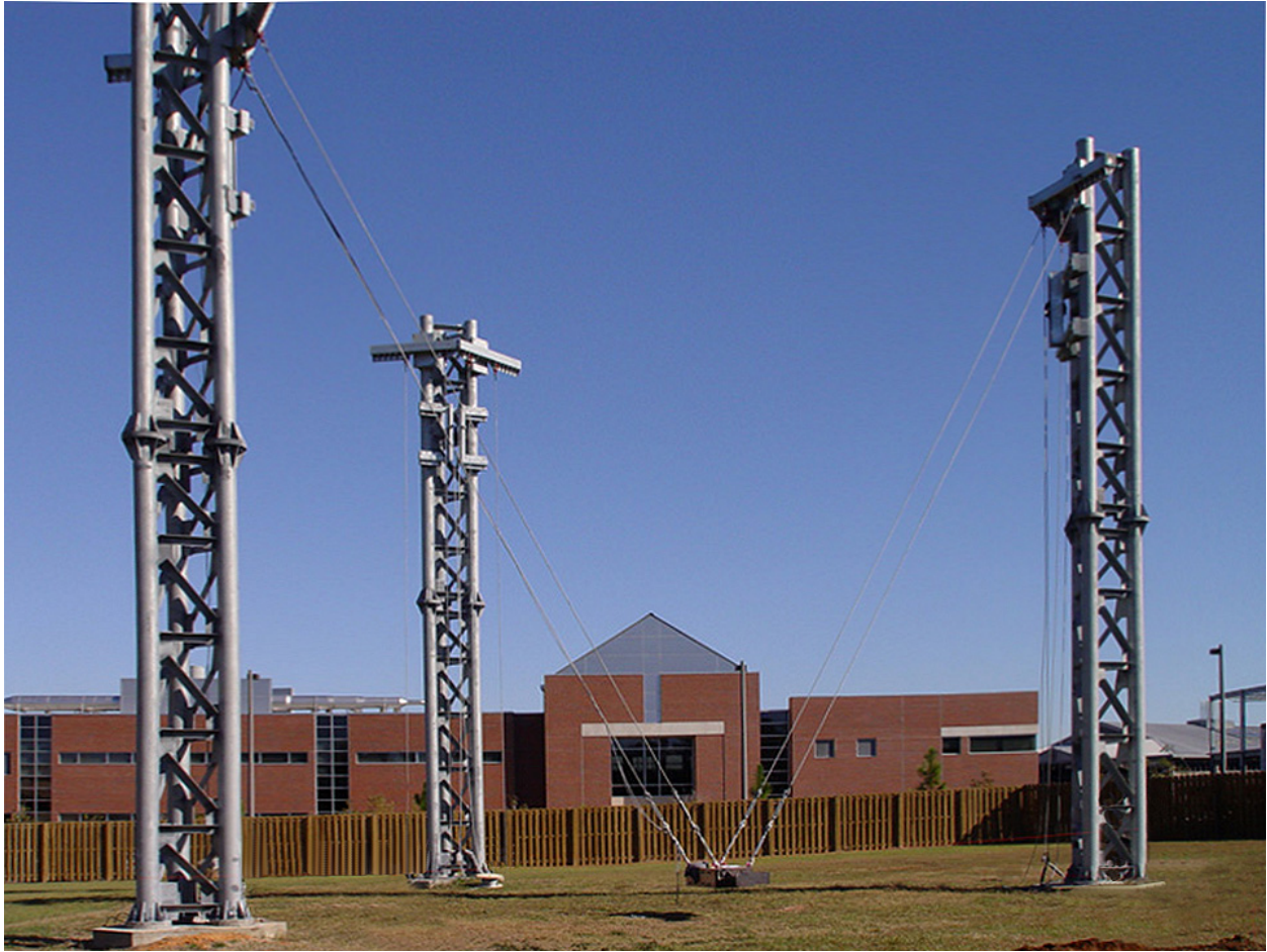
Figure 4-15. Completed pendulum impact test facility at the FDOT Structures Research Center
