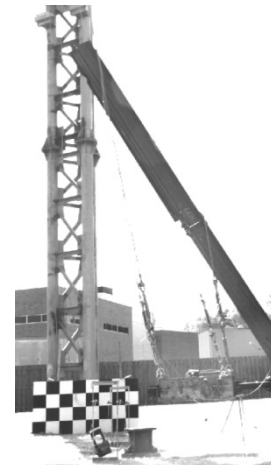
Figure 10-21. Oblique impact from high-speed camera (where t = 0 \text{ sec.} indicates contact between post and pendulum) for experiment T-25-2
