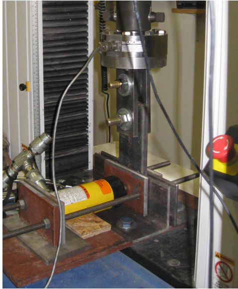
Figure 5-2. Experimental setup used to quantify static friction coefficients
