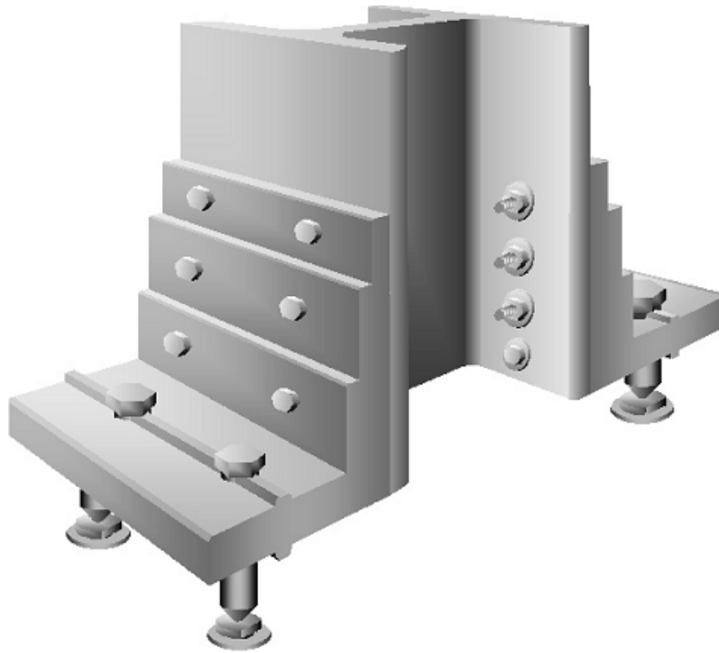
Figure 2-7. Multidirectional coupler (Transpo Industries, Inc.)
