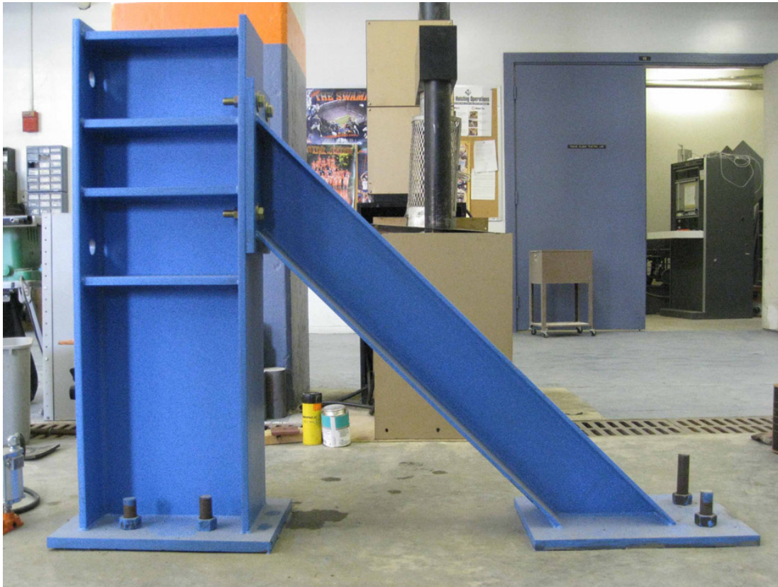
Figure 7-4. Steel support fixture in the UF Civil Eng. Structures Lab.
