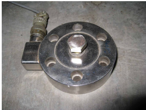
Figure 7-14. 5-kip pancake load cell
