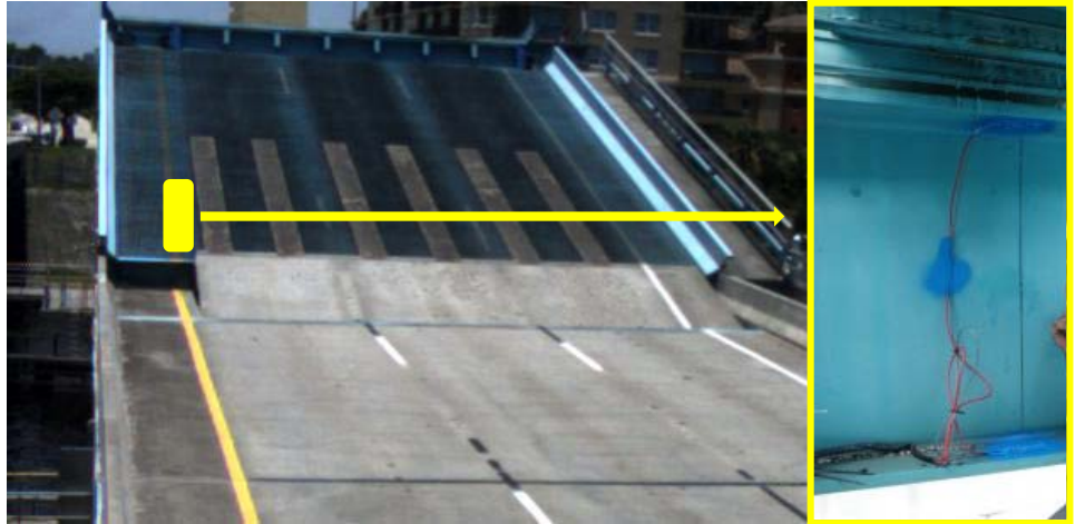
Figure 70: East South Main Girder Live Load Shoe Strain Gage Location
