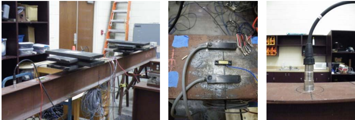
Figure 40: Loading Plates (Left), Installed Strain Gages (Center) and Accelerometer (Right)
