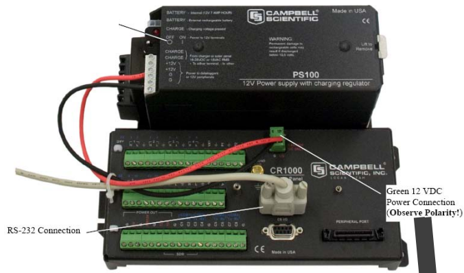
Figure 21: Power and Wiring Panel of CR1000 ( http://www.campbellsci.com/cr1000 )
