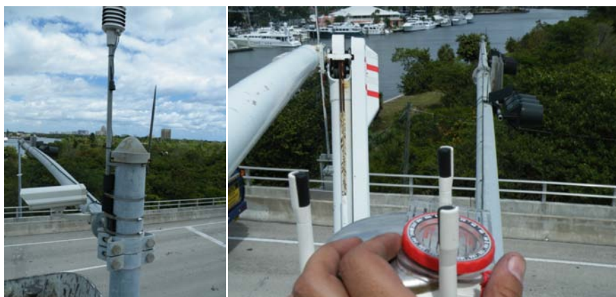
Figure 59: Setting of the Weather Station Direction with a Compass
