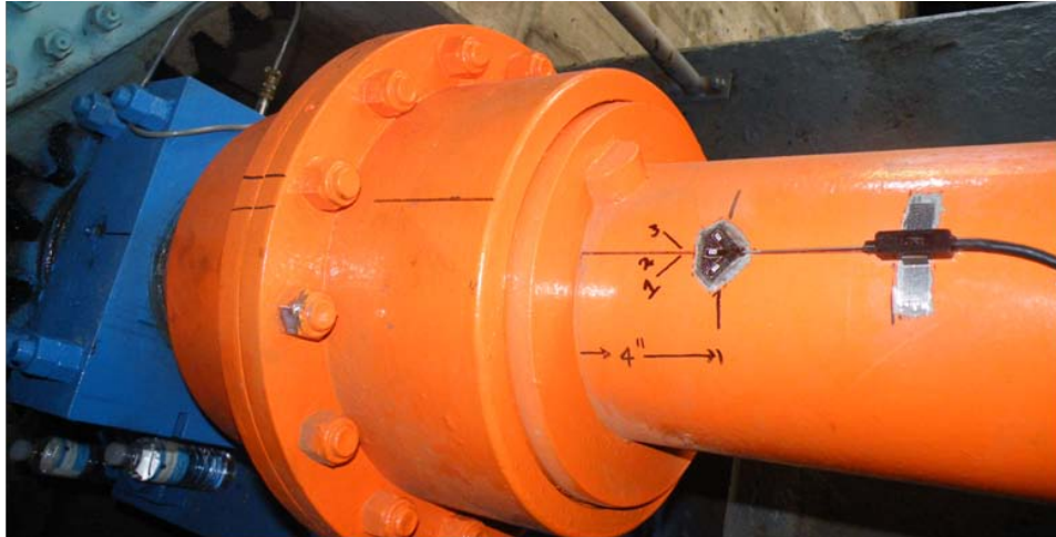
Figure 152: Strain Rosette on the Drive Shaft
