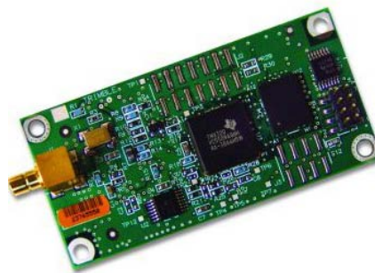
Figure 26: Trimble Resolution T GPS Timing Receiver
