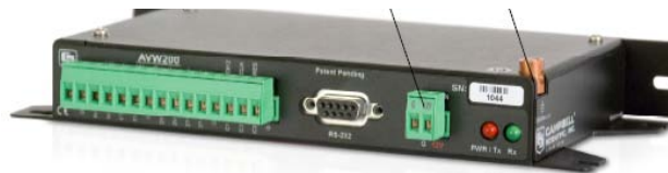
Figure 22: Vibrating Wire Interface of CR1000
