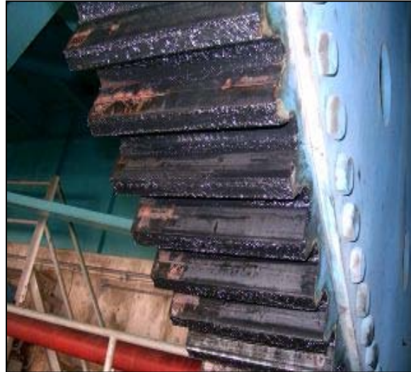
c) Open Gear without Grease
