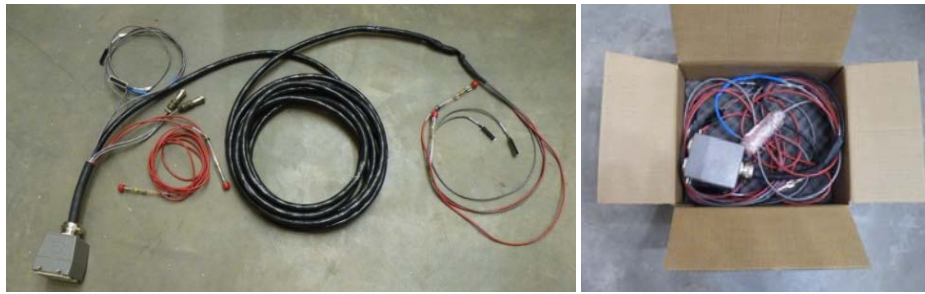
Figure 33: Sensor Group Ready for Bridge Installation
