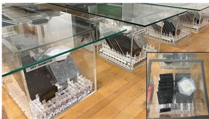
Photo 3.2. Photos of corrosion test setup.
