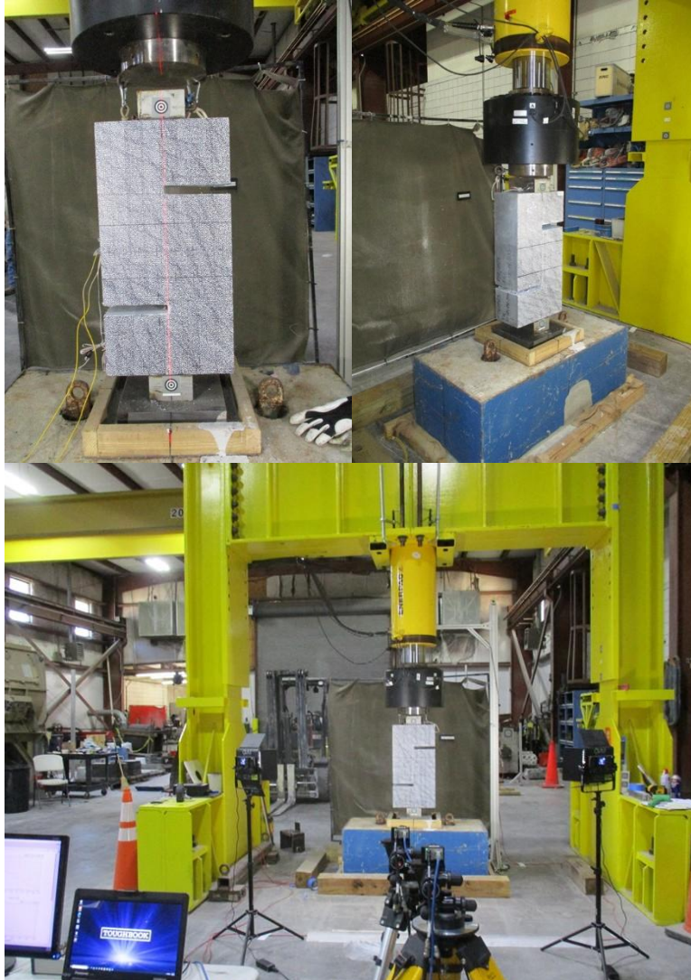
Photo 2.13. Sophisticated shear pushoff testing including test frame, mechanical actuators, sensors, data acquisitions, DIC high speed cameras and lighting.
