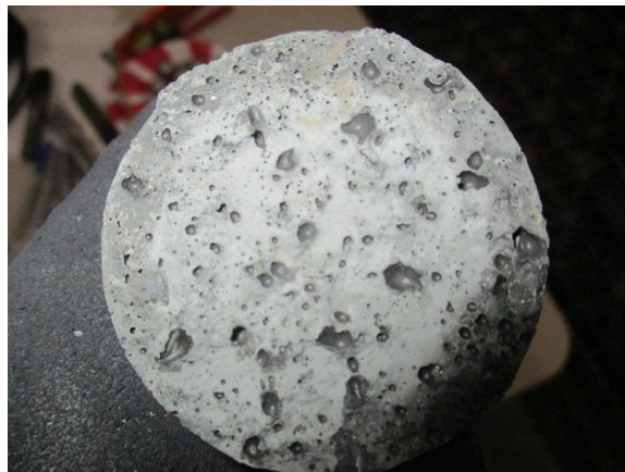
Photo 7.3. Concrete surface deficiency.
