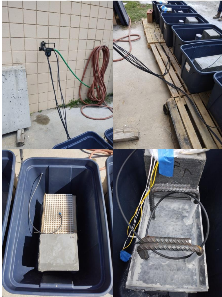
Photo 2.11. Development of irrigation system to maintain moisture or prolonged wet burlap and bonding wetting conditions and corrosion conditions for exposed steel fibers.
