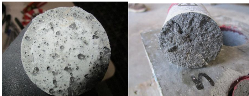
Photo 4.4. Comparison of porous interface (left) to typical interface appearance (right).
