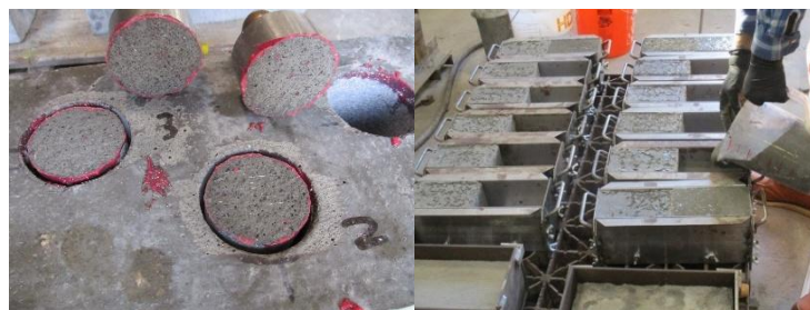
Photo 5.1. Porous friable UHPC skin material.
