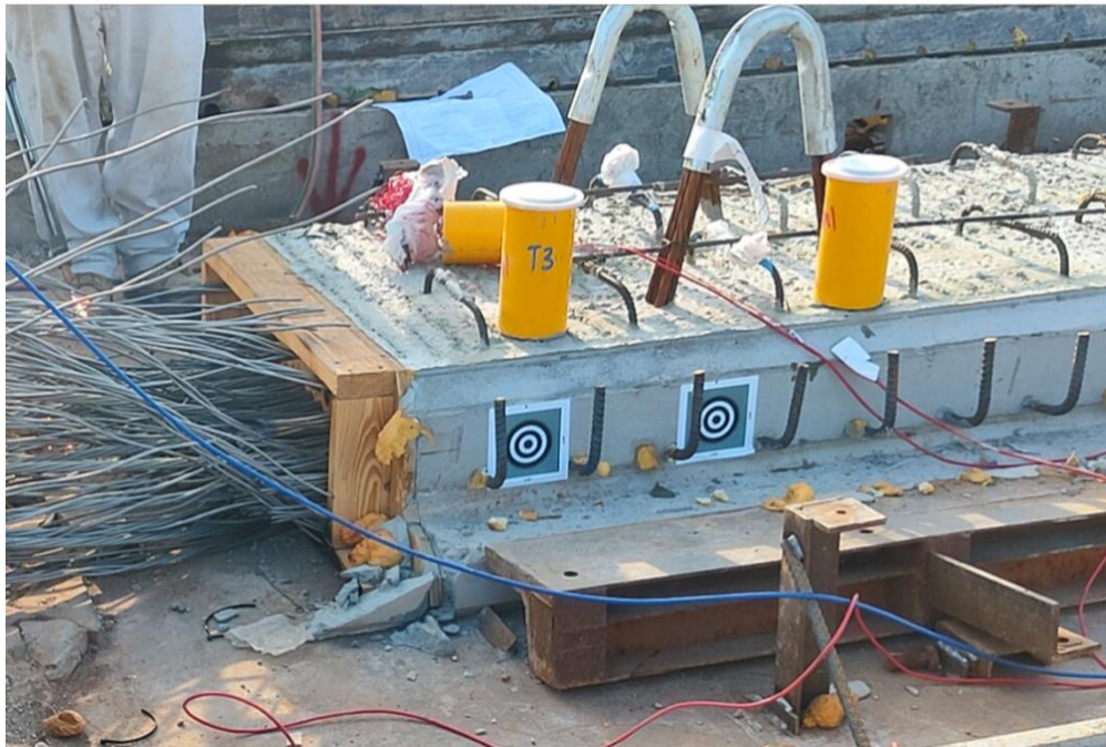
Figure 10-36. End 1 in FSB-1 immediately after strands release
