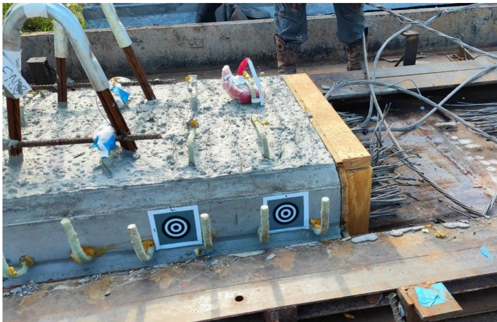
Figure 10-37. End 8 in FSB-4 immediately after strands release
