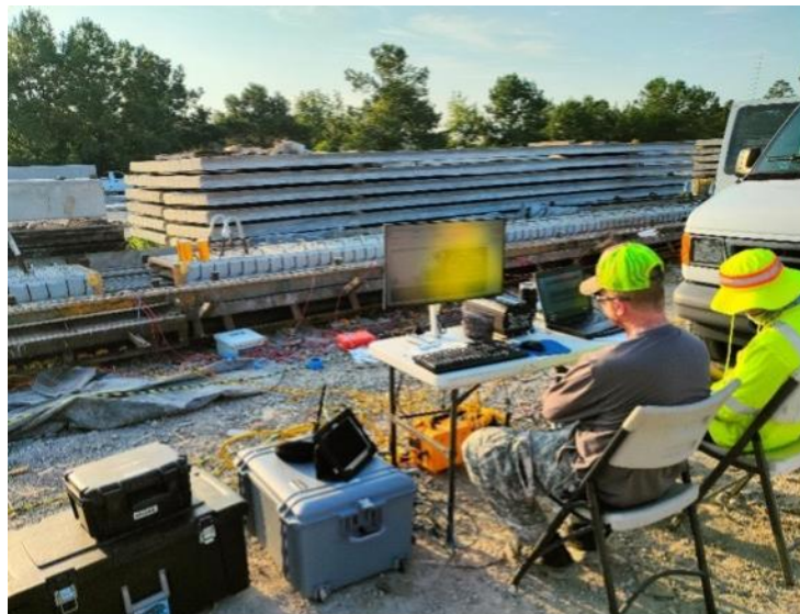
Figure 3-27. Acquisition system connected to the gauges to monitor the data
