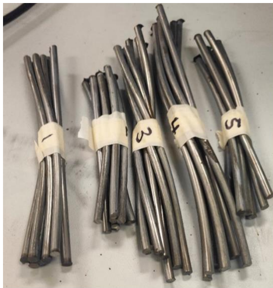
Figure 4-4. Wires taken from each specimen to determine diameter measurements
