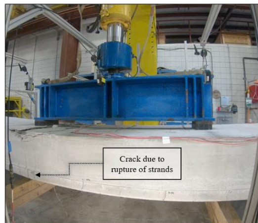
Figure 6-23. Failure sequence of FSB-3
