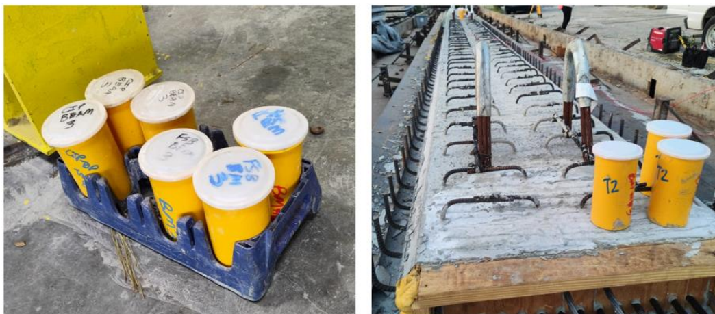
Figure 4-7. Concrete cylinders stored near the specimens
