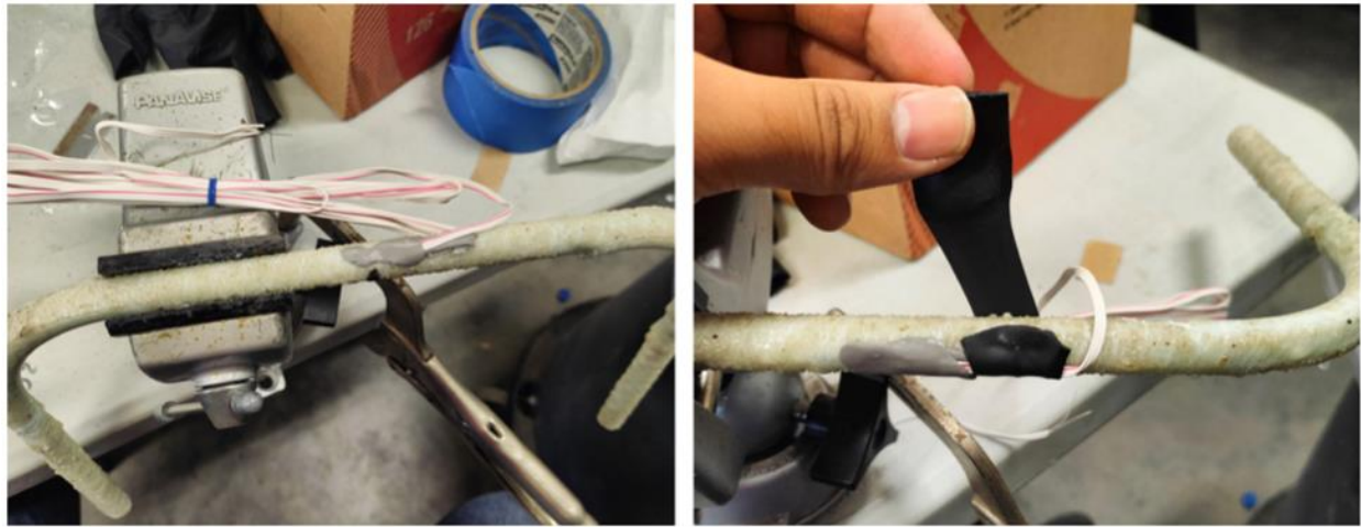
Figure 3-5. Gauge protection layers
