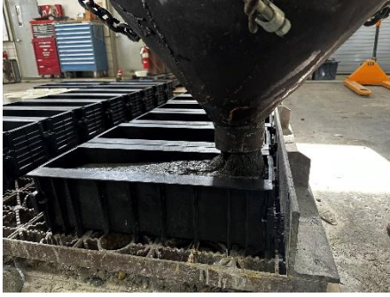
(a) Casting at end for parallel distribution of steel fiber
