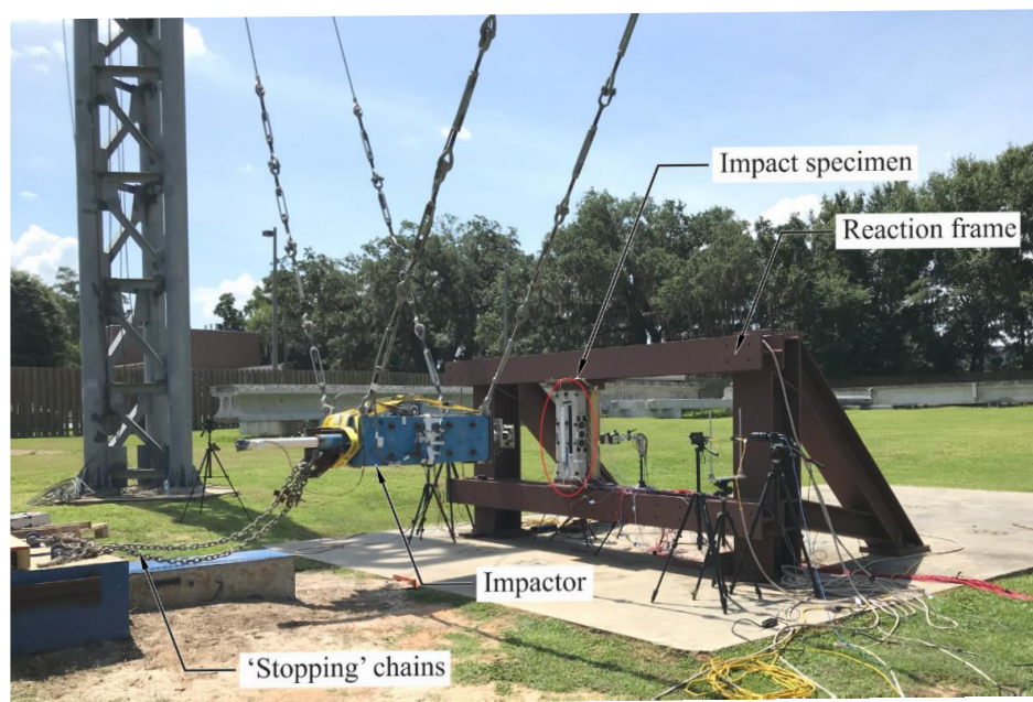
Figure 3.13 Pendulum impact test overview
