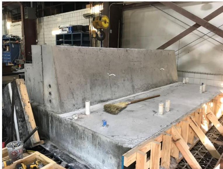
Figure 5.11 Completed (FRC) test specimen
