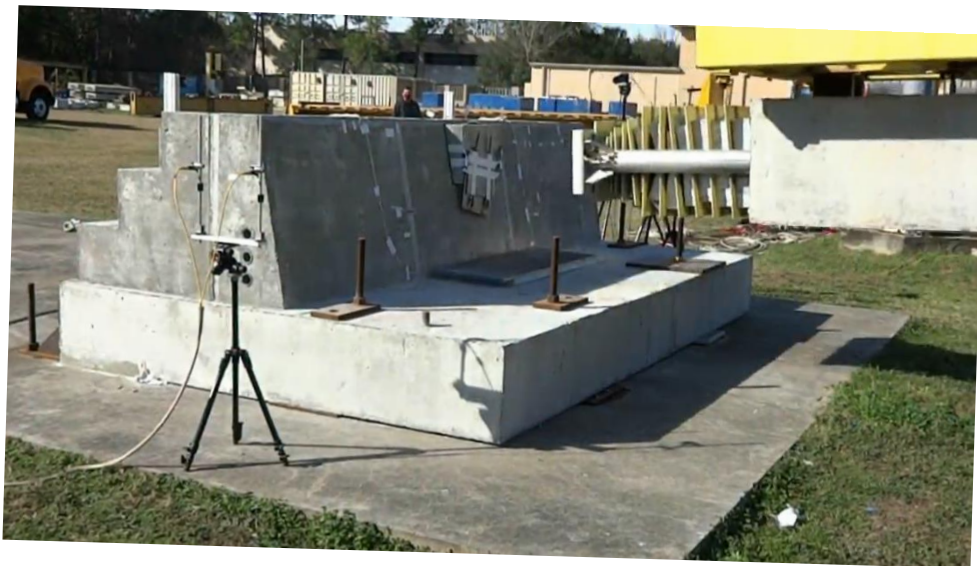
Figure 6.15 FRC COR test 2 specimen after completion of impact test
