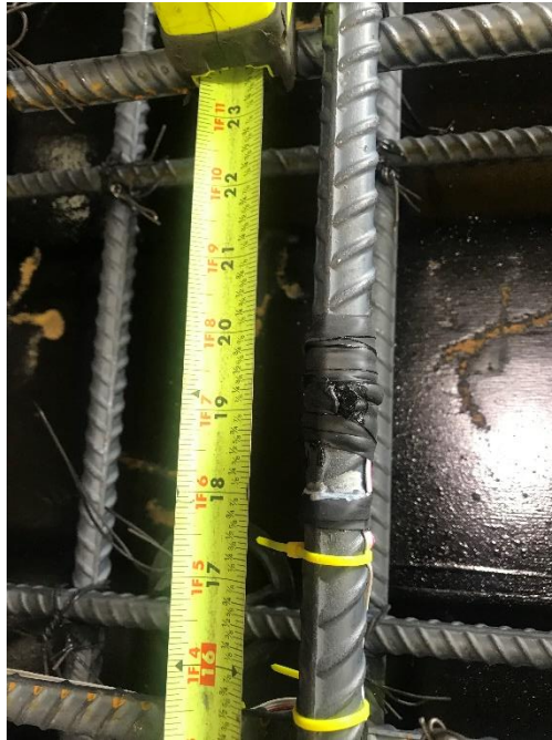
Figure 5.31 Strain gage attached to deck reinforcing bar and protected with waterproof tape
