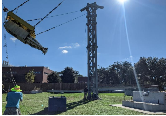
Figure 6.30 Impactor pulled back to 15-ft drop height (prior to release)
