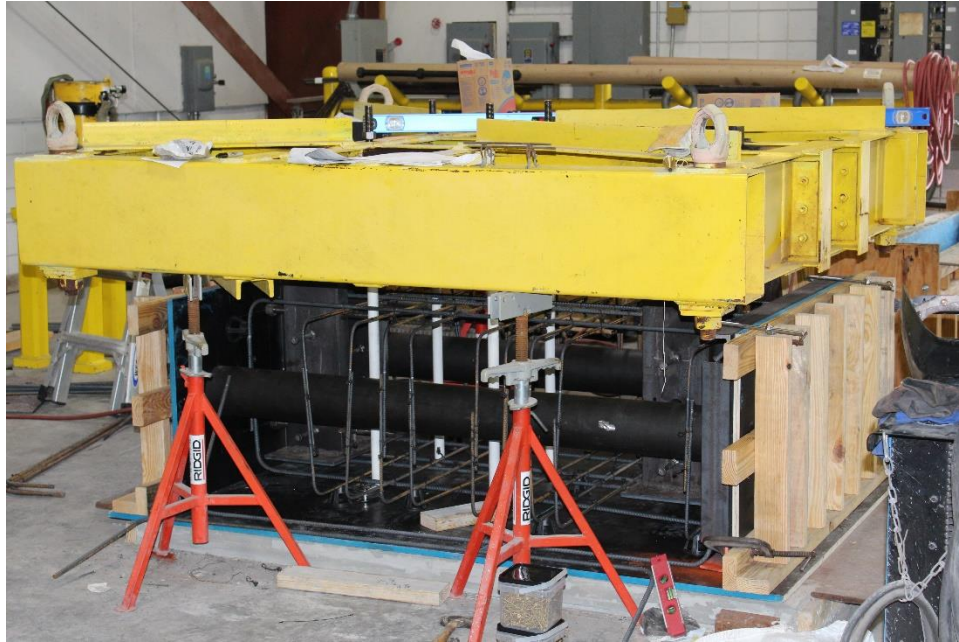
Figure 4.13 Steel hanger frame suspended above the concrete block formwork with embedded steel components correctly positioned
