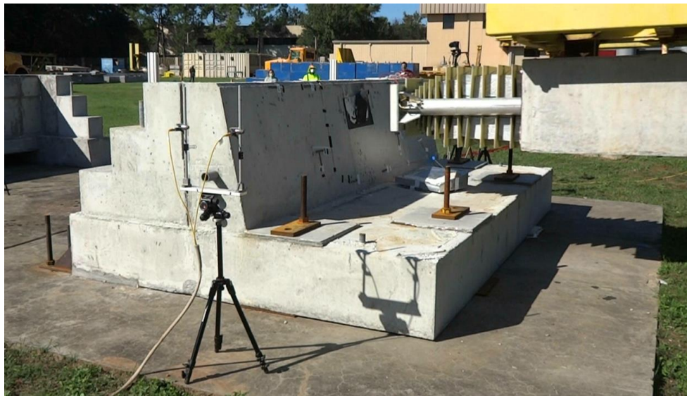
Figure 6.33 R/C COR 1 test specimen after completion of impact test
