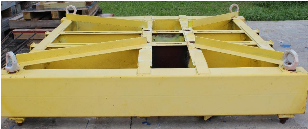
Figure 4.12 Repurposed steel hanger frame
