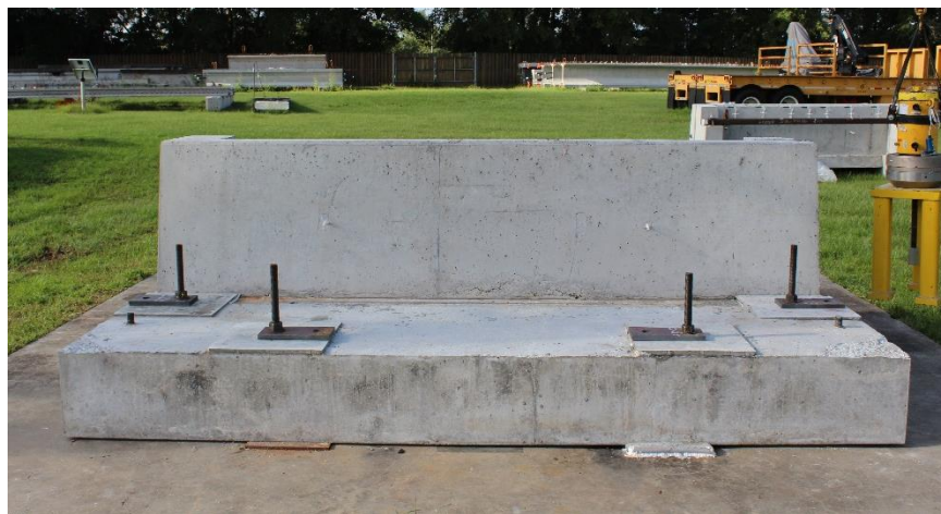
Figure 5.18 Anchored test specimen
