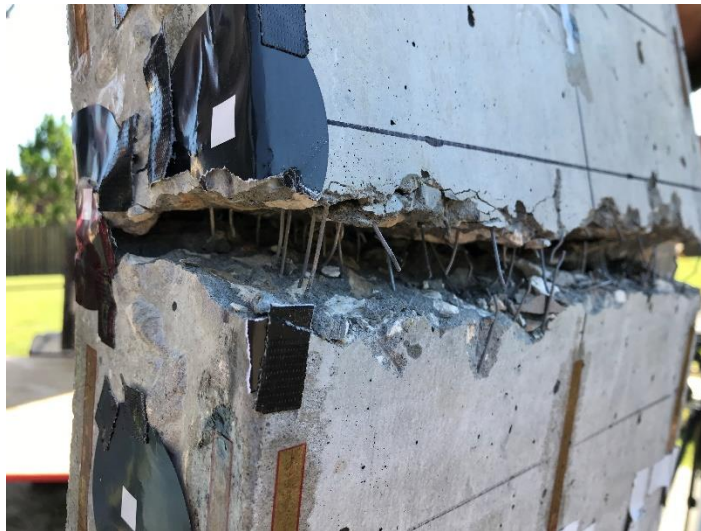
Figure 3.18 Final (preserved) state of FRC specimen-2
