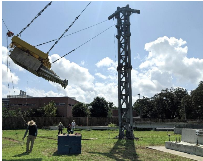
Figure 6.1 Impactor pulled back to 15-ft drop height (prior to release)
