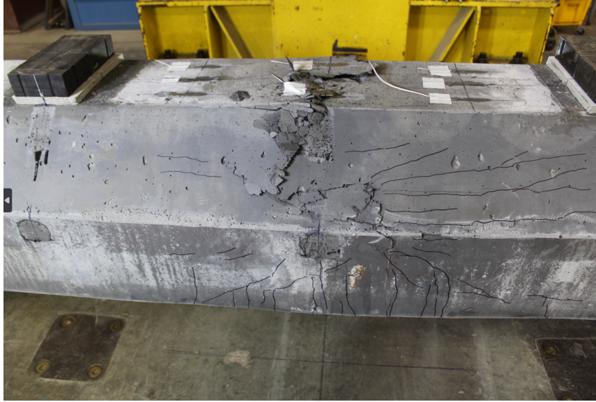
Figure 62: Failure of the 24-inch octagonal pile
