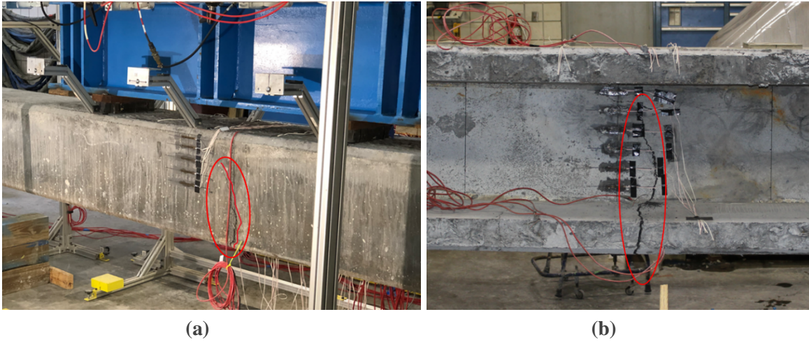
Figure 59: Strain localization failure in (a) 18-inch square and (b) 30-inch H (strong axis test)
