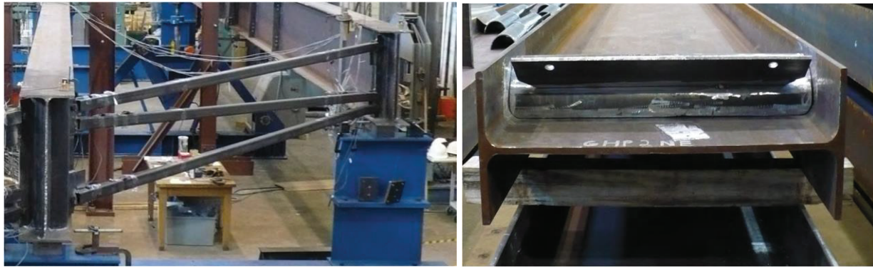
Figure 1.38 Large-scale test specimen with half-round bearing stiffener (left) and a single stiffener prepared for welding (right) Quadrato et al.[44]
