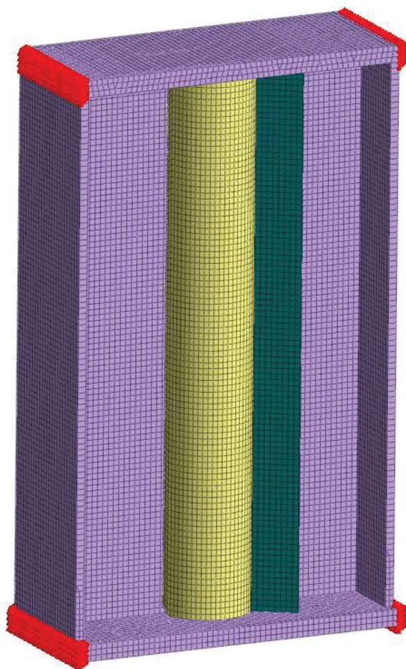
Figure 2.49- Boundry condition for FEM models defined in Midas FEA NX
