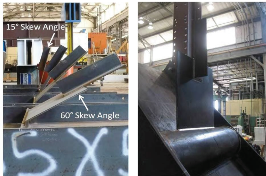
Figure 1.37 Small-scale connection test specimens by Quadrato et al.[44]
