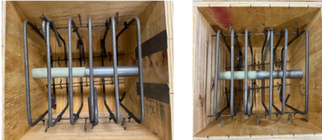
Figure 39. Concrete pullout bond specimen for Pultrall (left) and MST (right)
