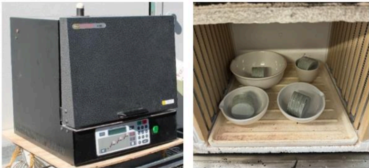
Figure 27. Fiber content furnace test setup
