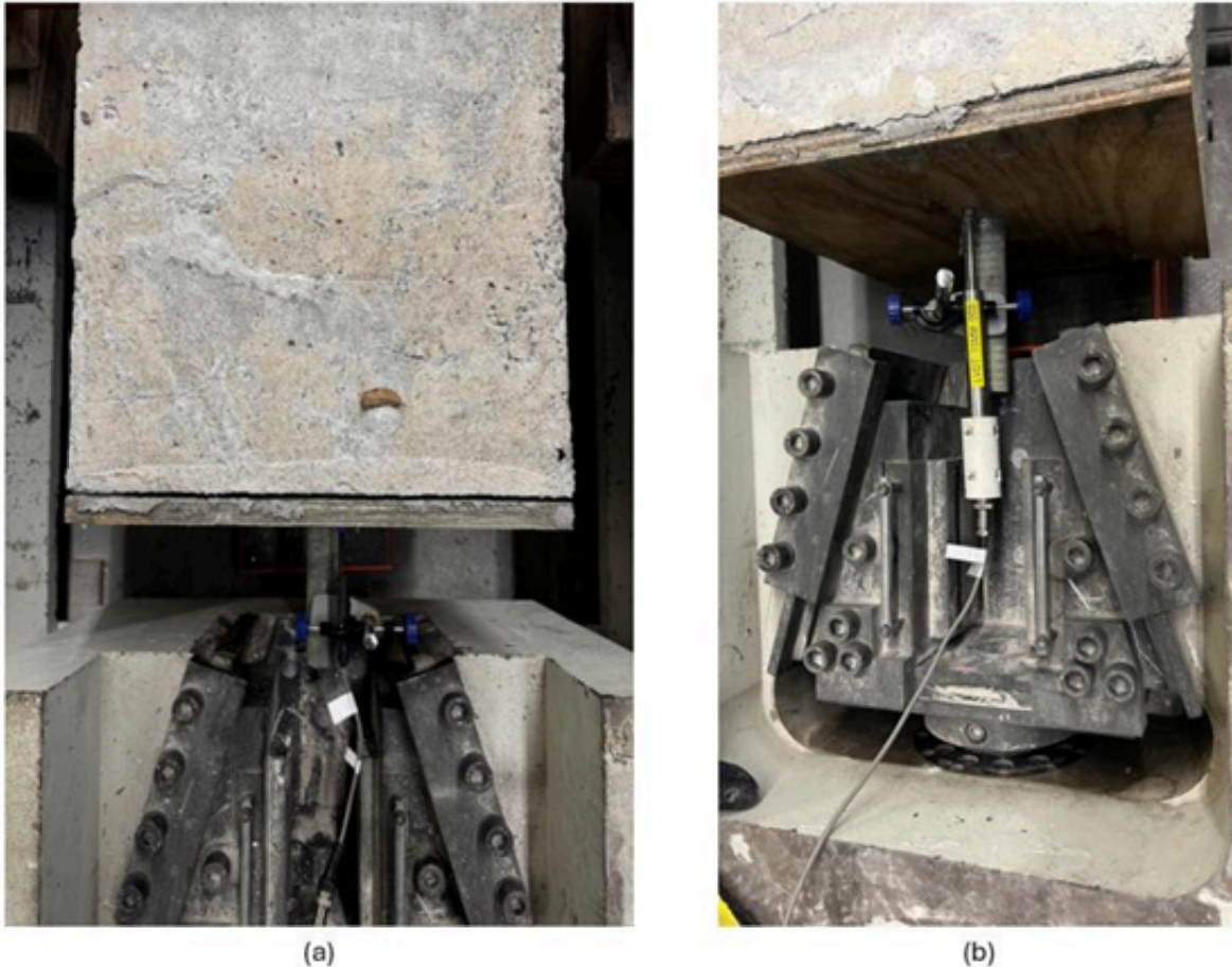
Figure 41. Bond strength representative slippage failure mode
