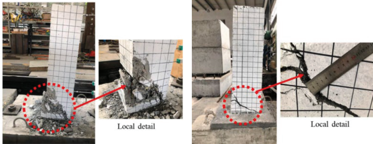
(a) Failure of RC column
