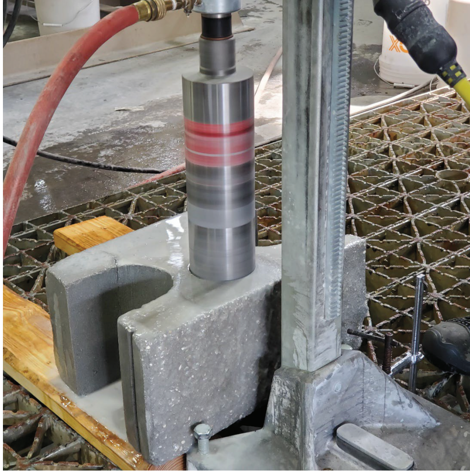
Figure 3-17. Drilling of the block cores.
