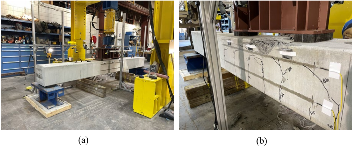
Figure 5.41: Flexure test pile setup.
