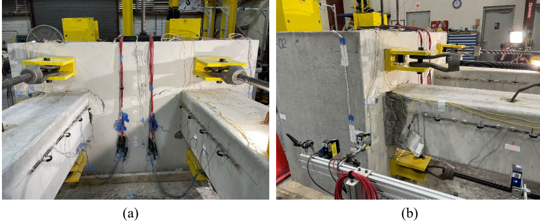
Figure 5.83: Photographs after failure of SP-02.
