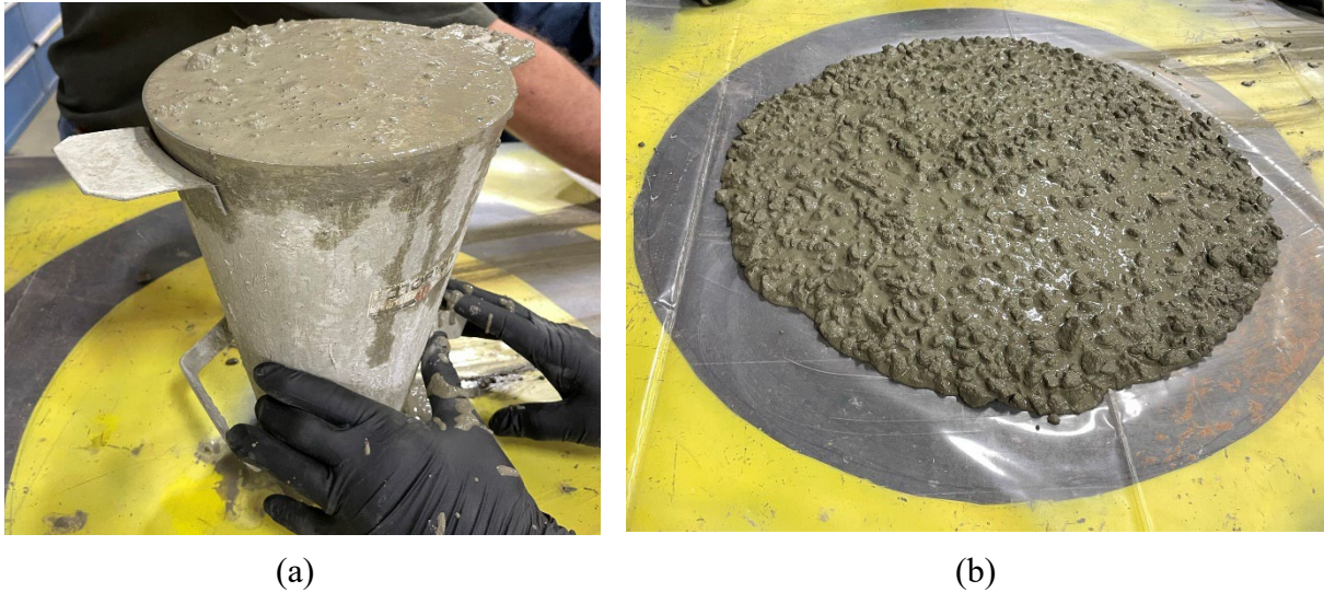
Figure 5.34: Standard slump flow test for SP-10: (a) inverted mold; (b) slump of 25 inches.
