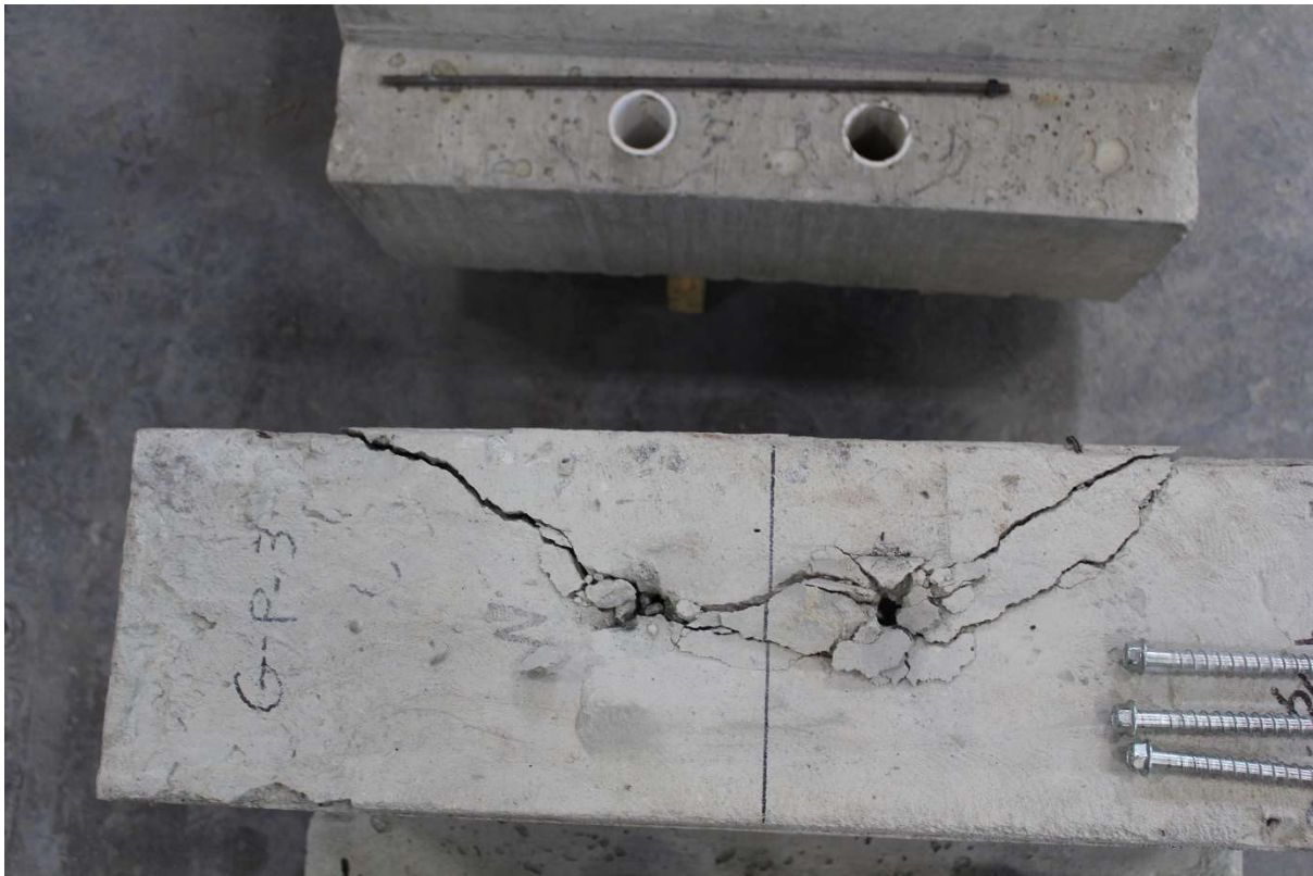
Figure A-126: G-G-312 specimen concrete after breakout
