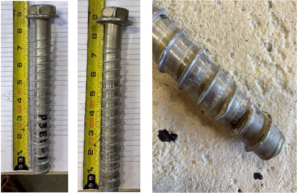
Figure A-5: P-SE1-1 specimen screw after loading
