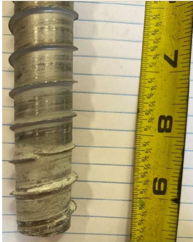
Figure A-47: G-SS-2 specimen south screw after loading
