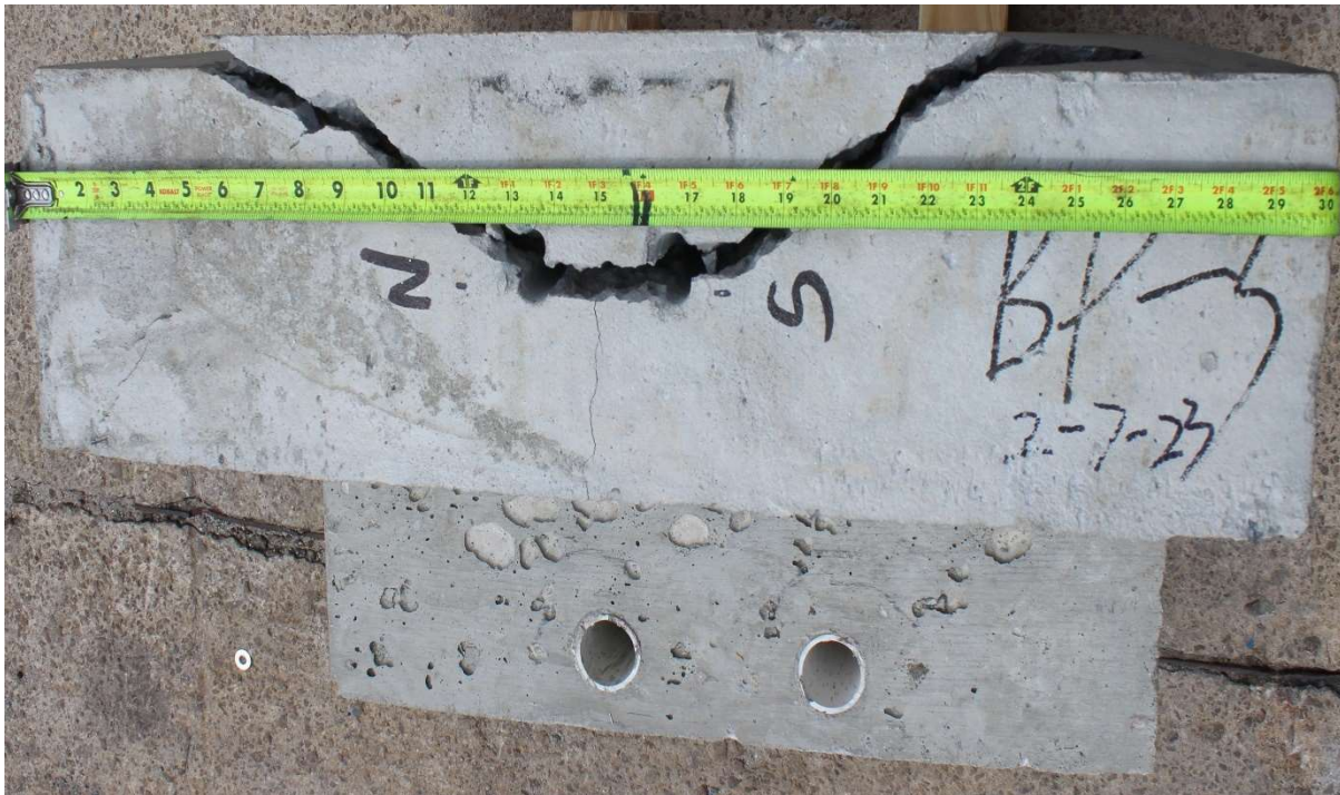
Figure A-101: B-P-3 specimen concrete after breakout
