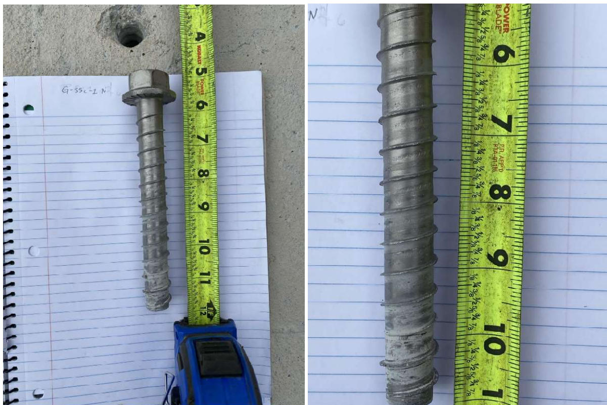
Figure A-56: G-SSc-1 specimen north screw after cyclic loading
