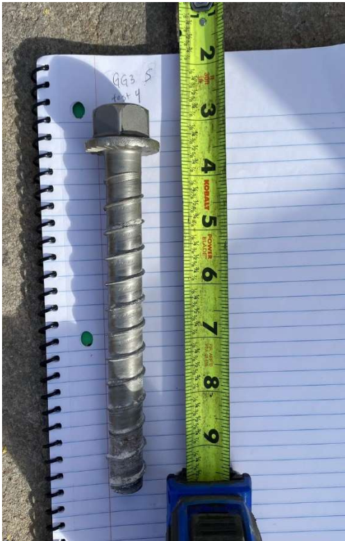
Figure A-82: G-G-3 specimen south screw after breakout
