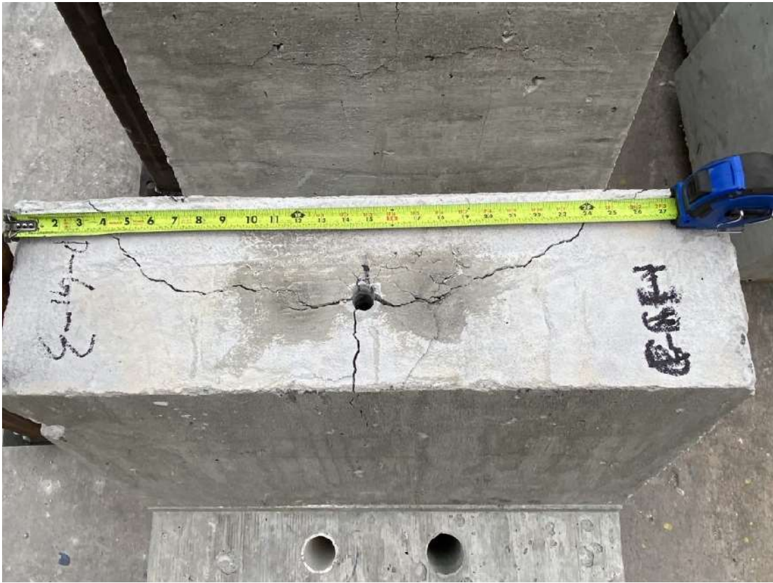
Figure A-34: P-G1-3 specimen concrete after anchor breakout
