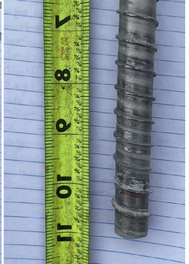
Figure A-66: G-SSc-4 specimen south screw after cyclic loading
