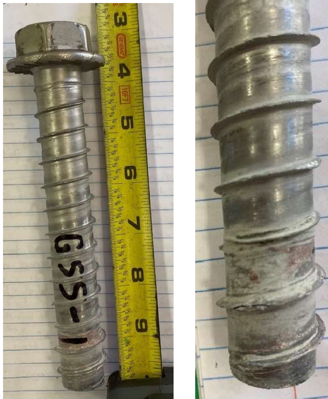
Figure A-45: G-SS-1 specimen screw after loading
