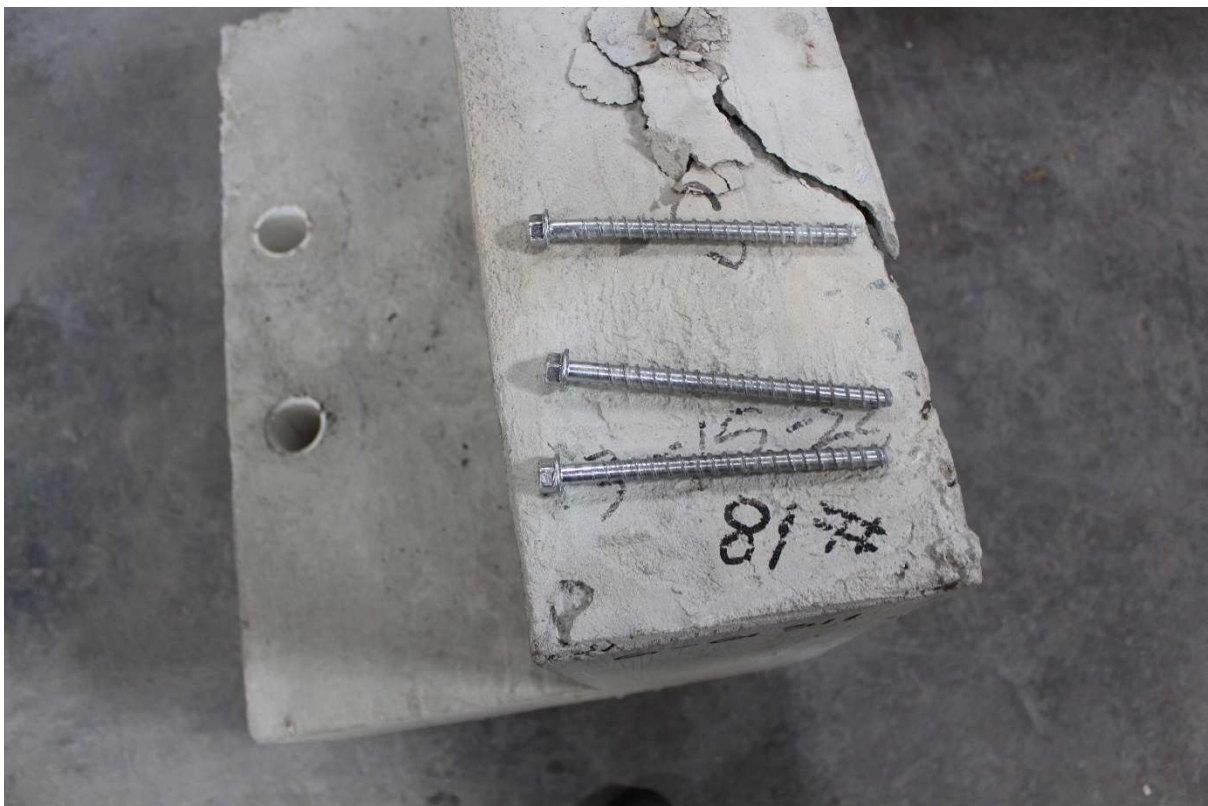
Figure A-125: G-G-311 specimen screw anchors after breakout
