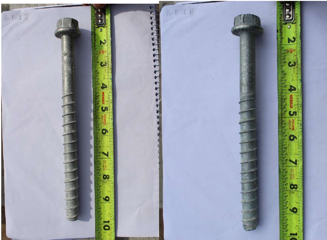
Figure A-96: B-P-1 south and north screw after breakout
