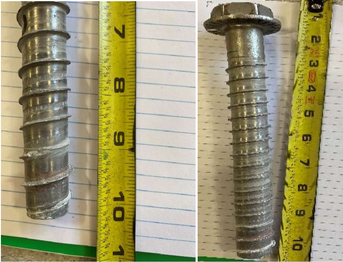
Figure A-9: P-SE1-3 specimen screw after loading
