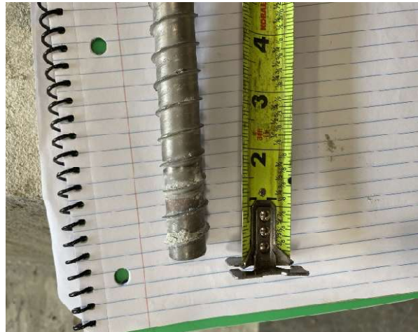
Figure A-79: G-G-2 specimen south screw after breakout
