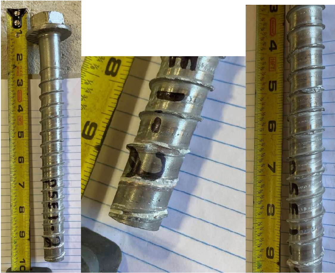
Figure A-7: P-SE1-2 specimen screw after loading
