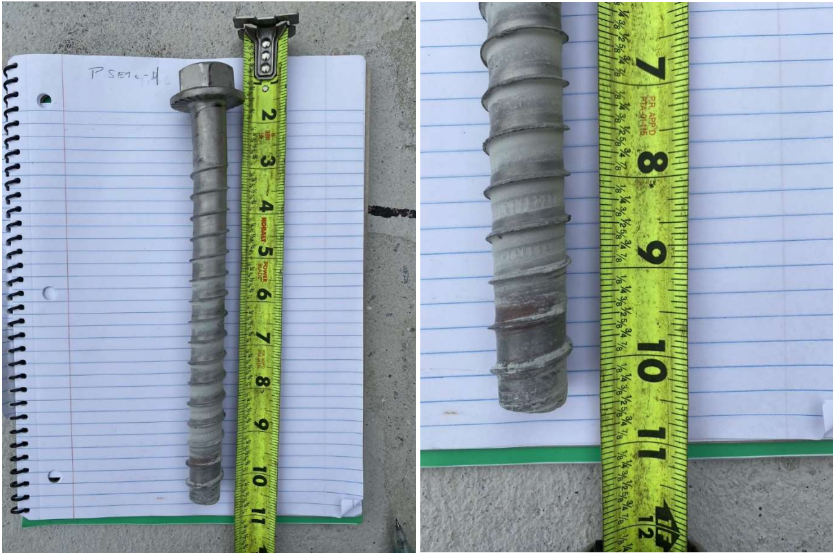
Figure A-23: P-SE1c-4 specimen screw after cyclic loading
