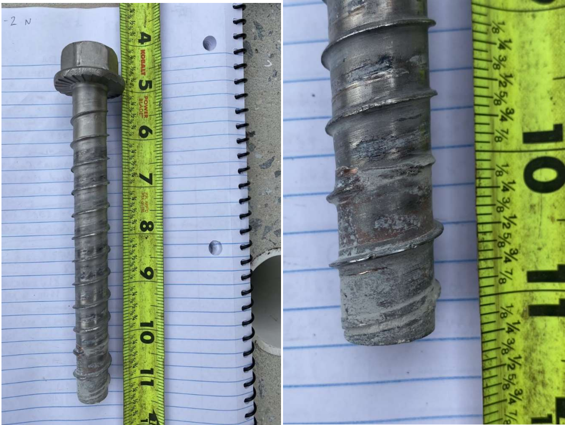
Figure A-59: G-SSc-2 specimen north screw after cyclic loading
