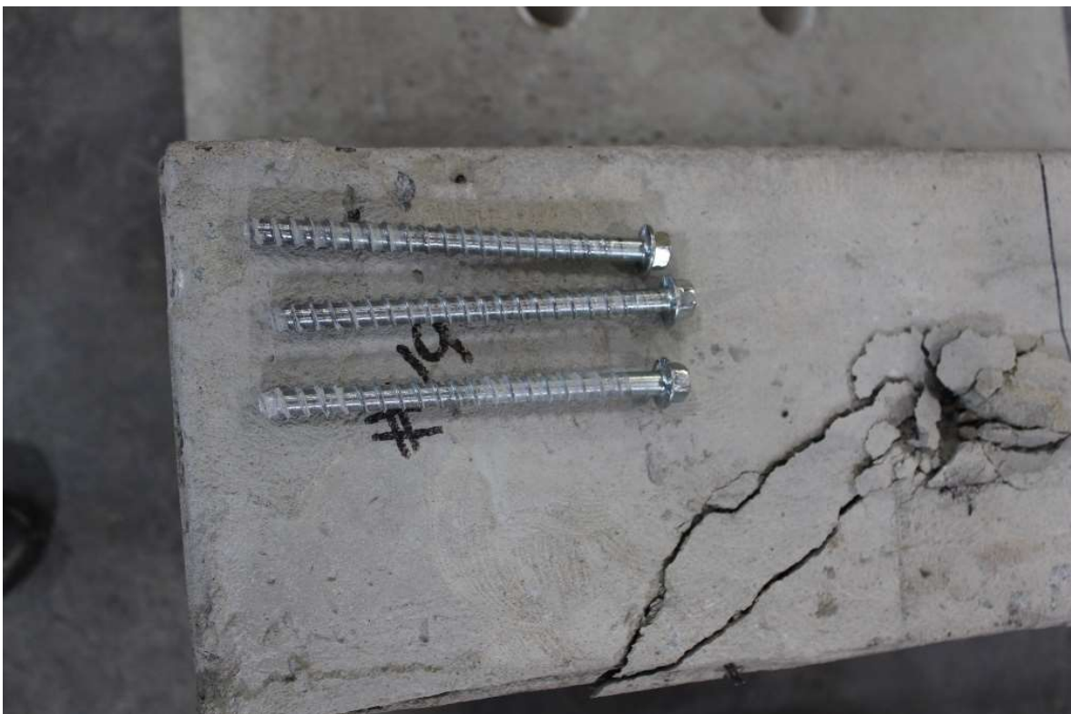
Figure A-127: G-G-312 specimen screw anchor breakout
