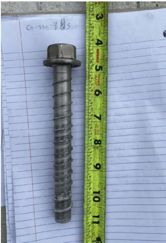
Figure A-66: G-SSc-4 specimen south screw after cyclic loading
