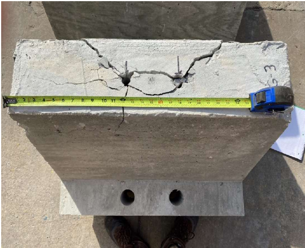
Figure A-83: G-G-3 specimen concrete after screw anchor breakout
