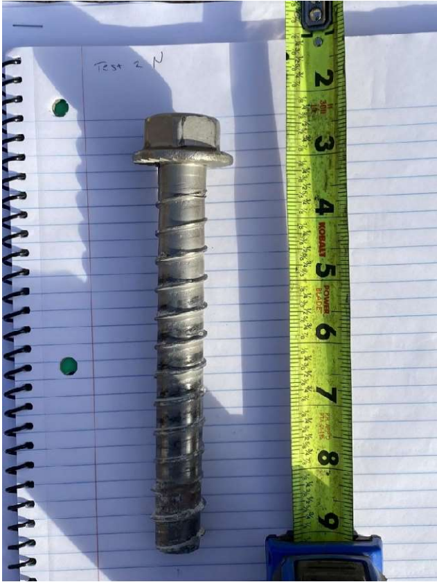
Figure A-75: G-G-1 specimen north screw after breakout
