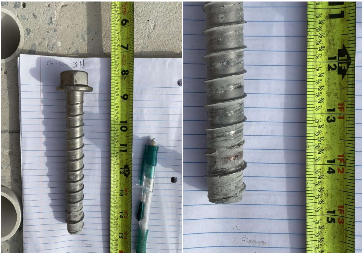
Figure A-62: G-SSc-3 specimen north screw after cyclic loading
