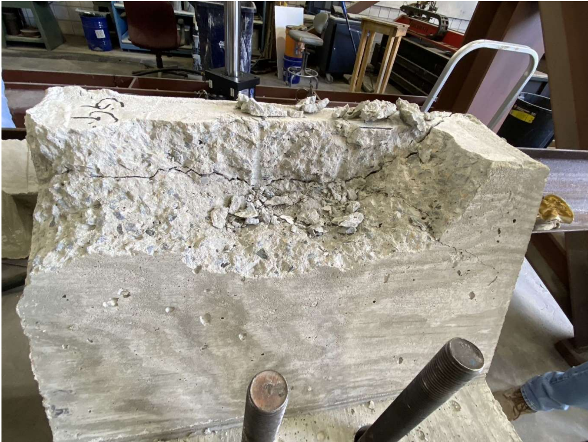
Figure A-77: G-G-1 specimen concrete after screw anchor breakout
