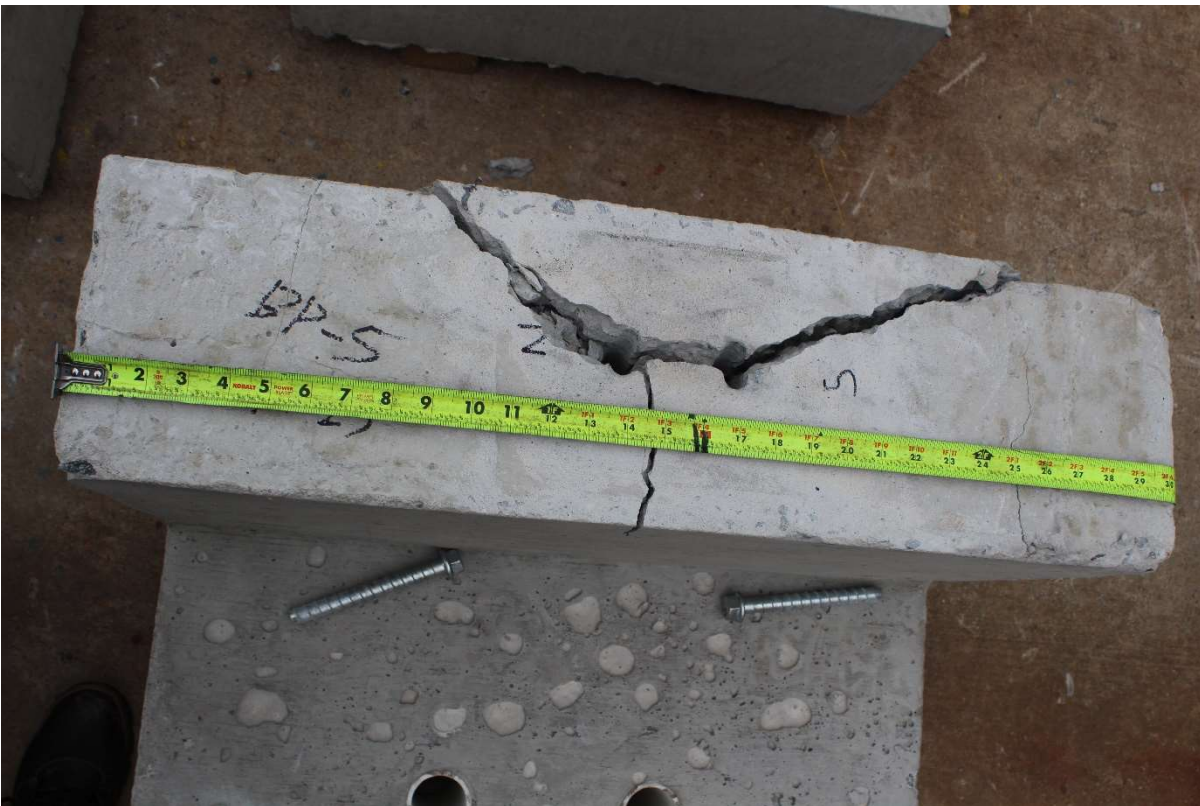
Figure A-105: B-P-5 specimen concrete after breakout
