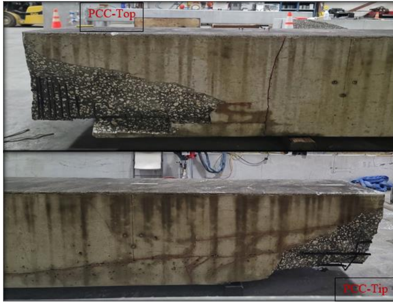
Figure 4.37: Failure at top and tip after final impact for PCC
