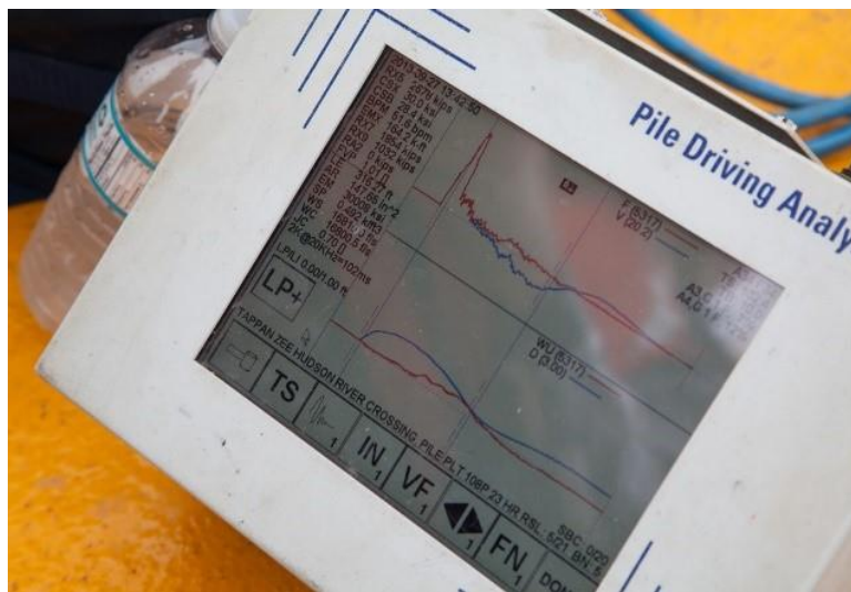
Figure 2.6: Pile driving analyzer (PDA)
