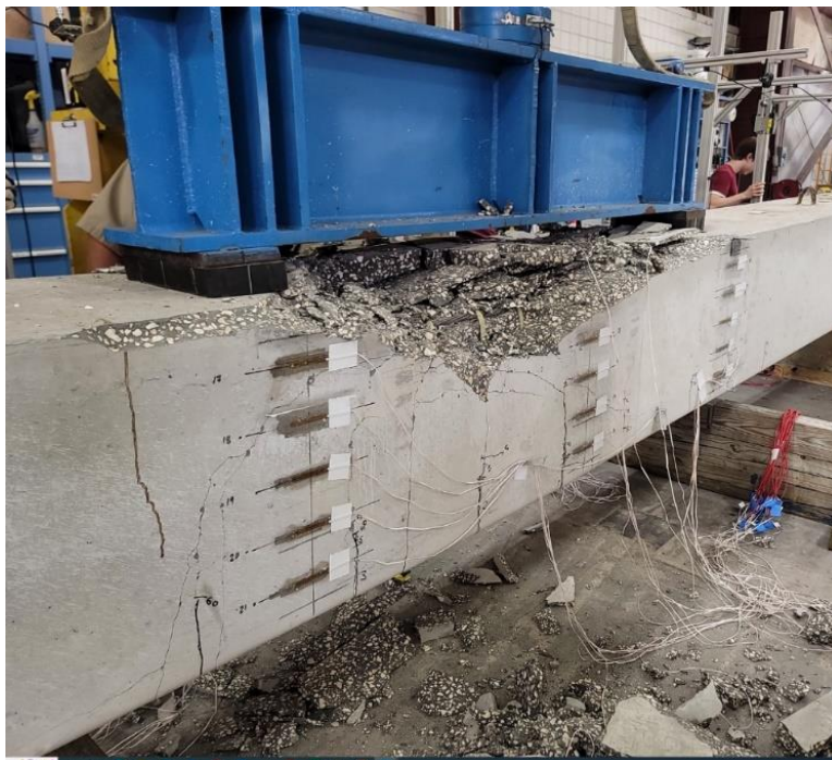
Figure 4.45: Concrete crushed in the compression zone
