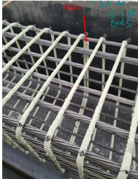
Figure 4.7: Spiral splicing: (a) PSG2, (b) PSG1
