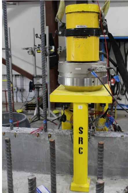
Figure 7: Testing equipment photograph with side view of UHPC strip
