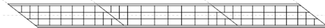
Figure 35. Bridge 2C3-47 ( L_s=152 ft, 195 ft, 152 ft; w_g=36 ft; \theta=50^\circ ; I_s=0.28, 0.22, 0.28 ; n_g=4 ; n_{CF}=8, 9, 8 ; O_{min.ext}/b_f=4.0 ; O_{min.int}/b_f=4.0 ).
