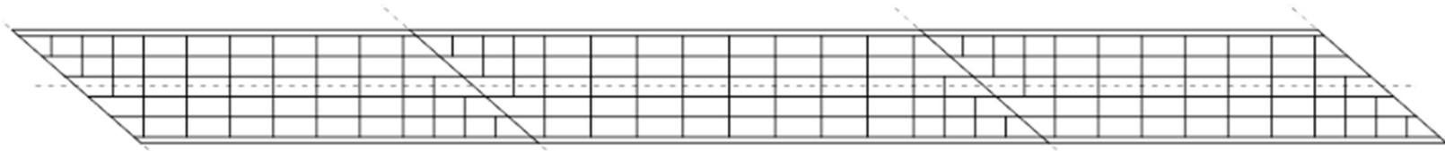
Figure 37. Bridge 2C3-51 ( L_s=222 ft, 285 ft, 222 ft; w_g=60 ft; \theta=47^\circ ; I_s=0.29, 0.23, 0.29 ; n_g=6 ; n_{CF}=10, 12, 10 ; O_{min.ext}/b_f=4.0 ; O_{min.int}/b_f=4.0 ).
