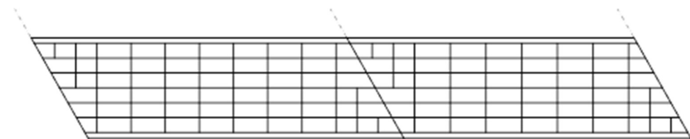
Figure 31. Bridge 2C2-46C ( L_s=228 ft, 207 ft; w_g=63.4 ft; \theta=35^\circ ; I_s=0.20, 0.21 ; n_g=7 ; n_{CF}=9, 8 ; O_{min.ext}/b_f=4.0 ; O_{min.int}/b_f=4.0 ).
