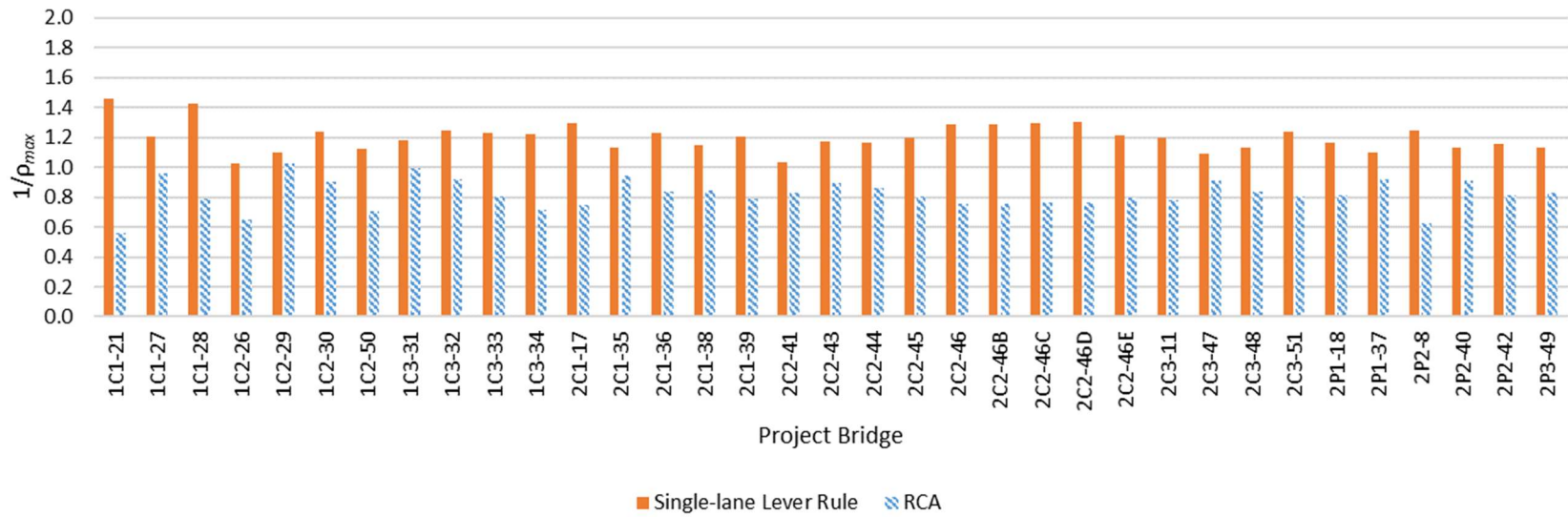
Figure 91. Ratios of the LGA moment LLDFs (single lane) to the 3D FEA-based AASHTO fatigue moment LLDF for the exterior girders.
