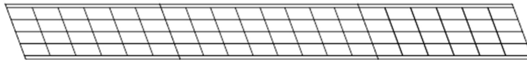
Figure 14. Bridge 1C3-32 ( L_s=152 ft, 195 ft, 152 ft; w_g=48 ft; \theta=20^\circ ; I_s=0.12, 0.09, 0.12 ; n_g=5 ; n_{CF}=5, 7, 5 ).
