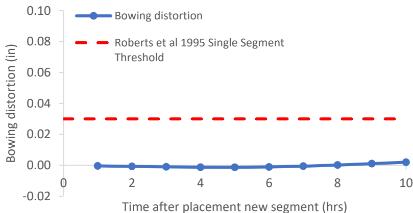
Figure B-83: Simulation 28 - Bowing distortion progression of match-cast segment from time of placement of new segment to 10 hours
