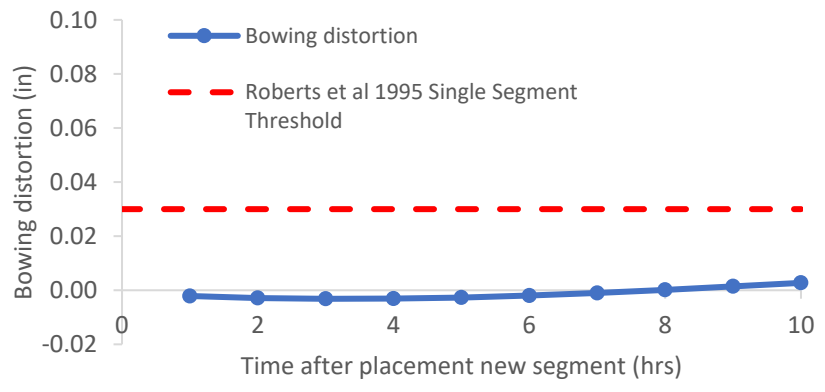
Figure B-389: Simulation 130 - Bowing distortion progression of match-cast segment from time of placement of new segment to 10 hours
