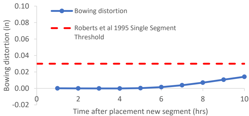
Figure B-449: Simulation 150 - Bowing distortion progression of match-cast segment from time of placement of new segment to 10 hours
