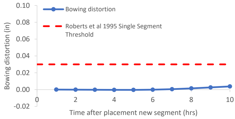
Figure B-110: Simulation 37 - Bowing distortion progression of match-cast segment from time of placement of new segment to 10 hours
