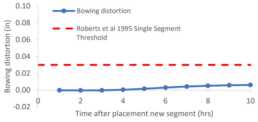
Figure B-338: Simulation 113 - Bowing distortion progression of match-cast segment from time of placement of new segment to 10 hours
