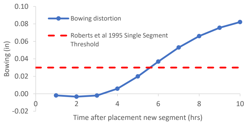
Figure B-107: Simulation 36 - Bowing distortion progression of match-cast segment from time of placement of new segment to 10 hours
