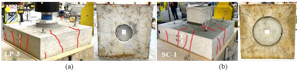
Figure 4.40: Crack patterns at failure for LP and SC specimens with corrugated interface (a) LP-3 and (b) SC-1
