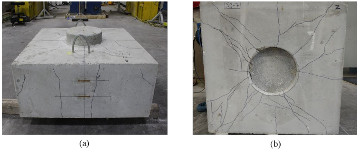
Figure A.183: Cracking on (a) cap and (b) bottom of Specimen S3-7
