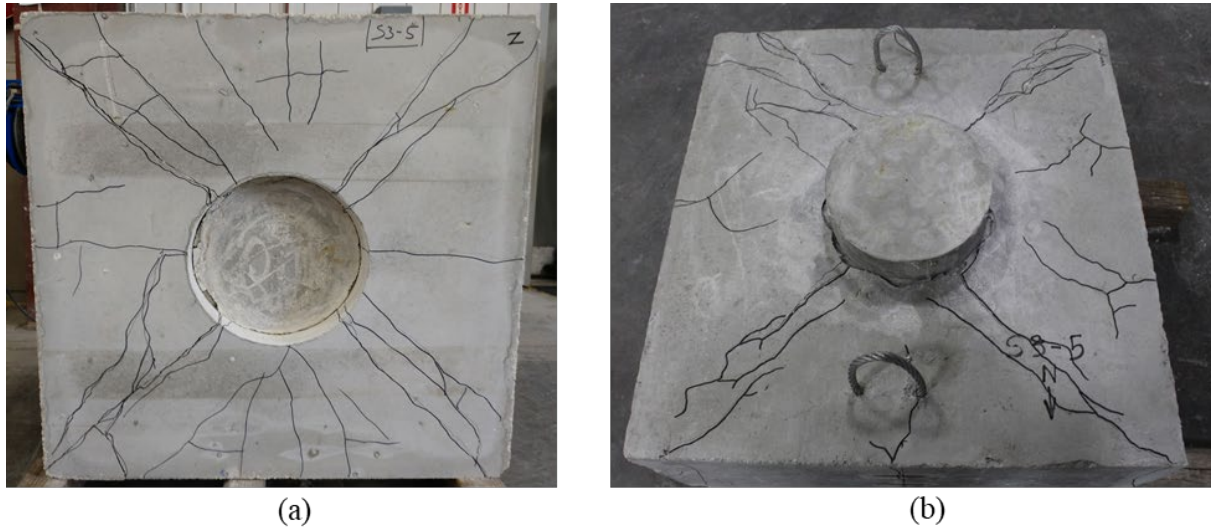
Figure A.170: Cracking on (a) cap and (b) bottom of Specimen S3-5
