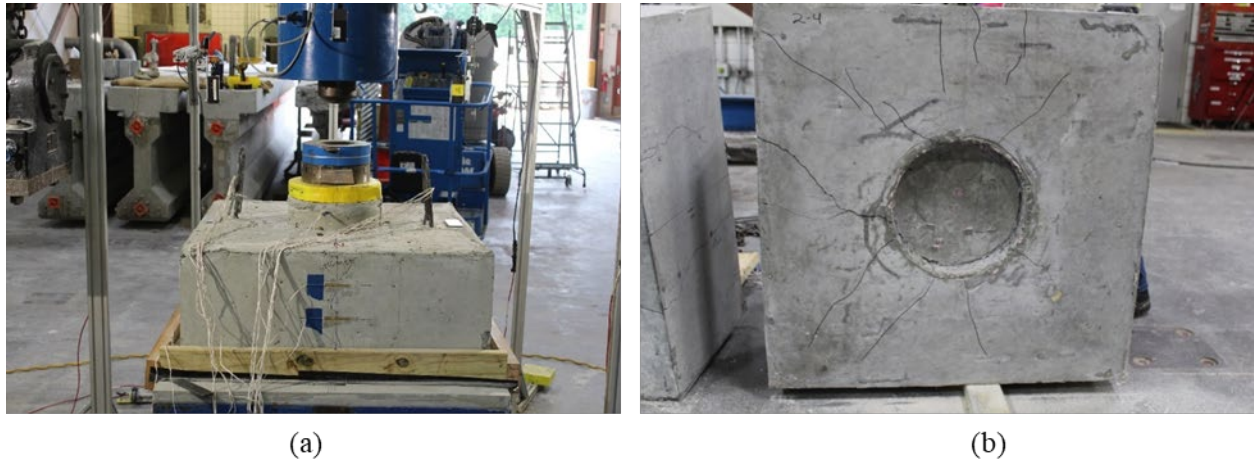
Figure A.45: Specimen S2-4 (a) elevation before testing and (b) bottom cracking after testing
