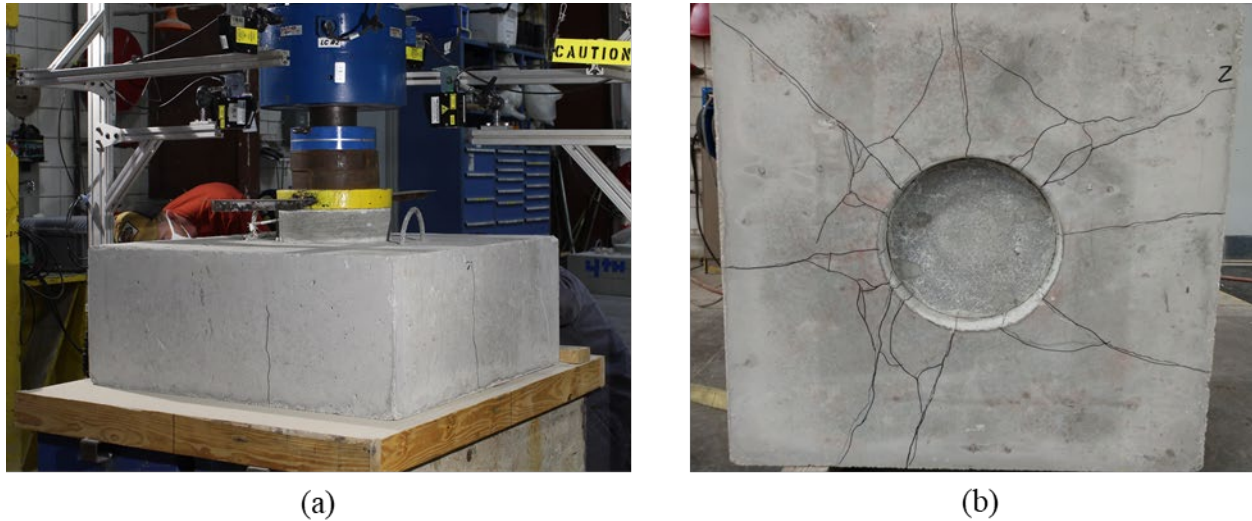
Figure A.144: Specimen S3-1 (a) elevation during testing and (b) bottom cracking after testing
