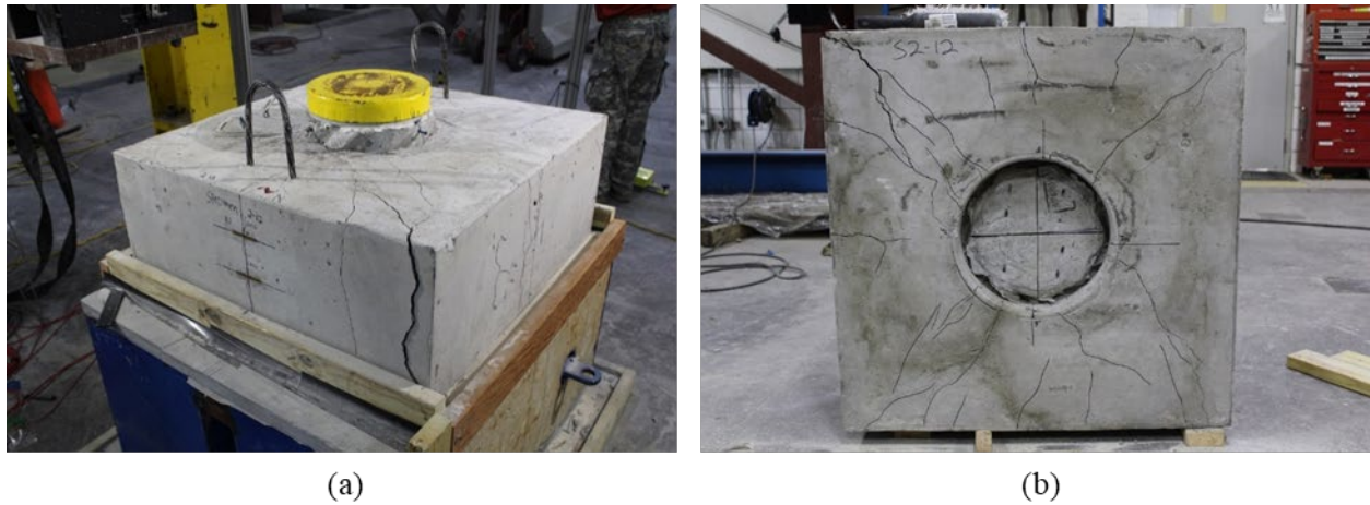
Figure A.102: Cracking on (a) cap and (b) bottom of Specimen S2-12
