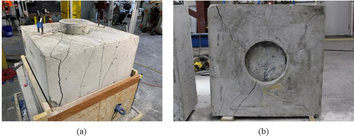
Figure A.66: Cracking on (a) cap and (b) bottom of Specimen S2-7
