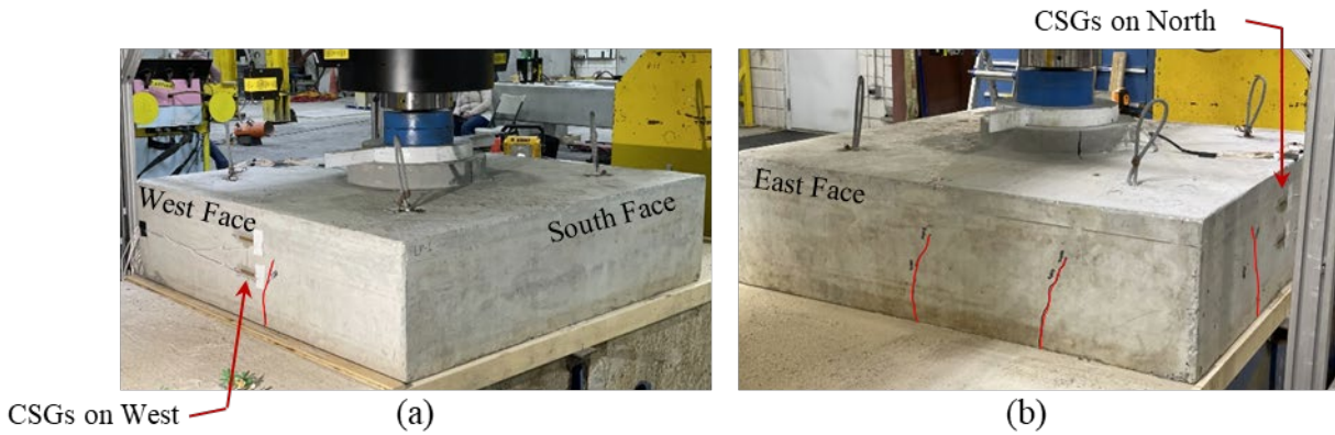
Figure B.3: Crack progression during testing at (a) 100 kips and (b) 200 kips
