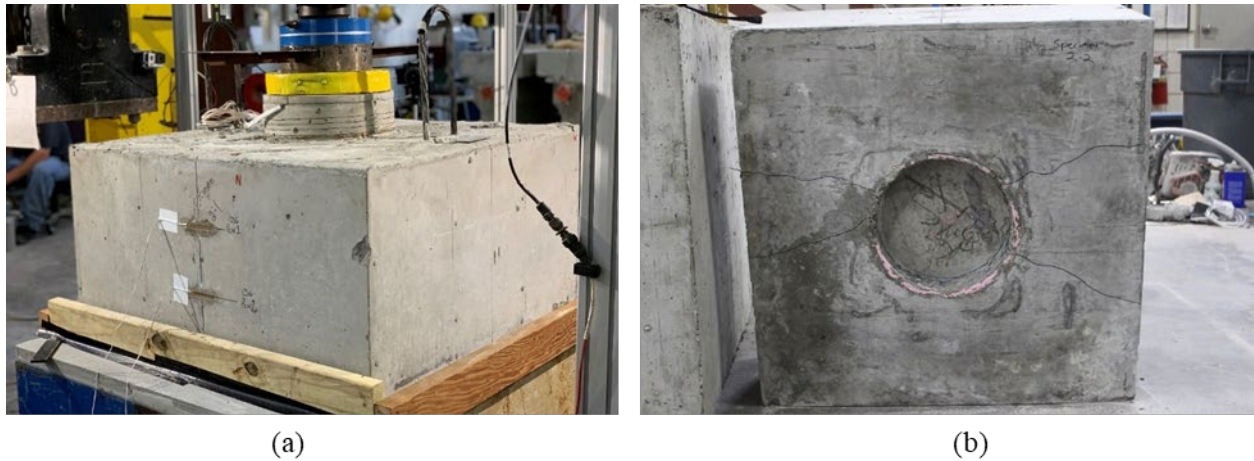
Figure A.31: Cracking on the (a) surface of the cap and (b) bottom of the specimen S2-2
