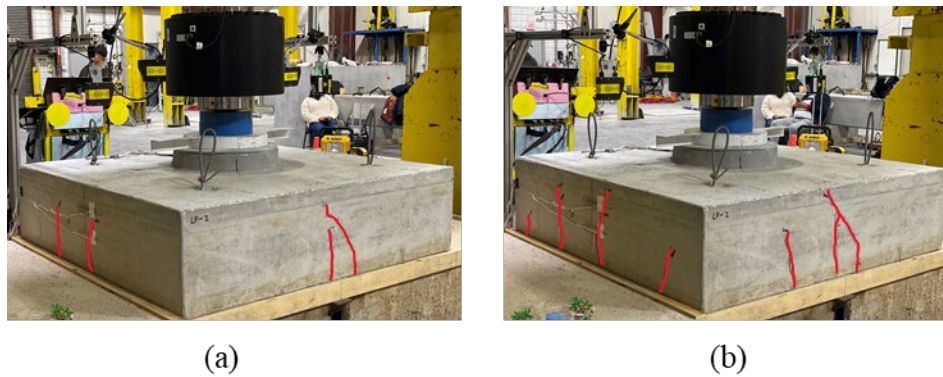
Figure B.10: Crack progression during testing at (a) 200 kips and (b) 300 kips
