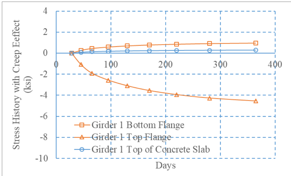
Figure 11-14. Time history for stress along longitudinal direction for girder #1 at midspan (creep effect, an 80 ft single span plate girder bridge with 10' spacing, five-girder system, shoring at 1/3 points)
