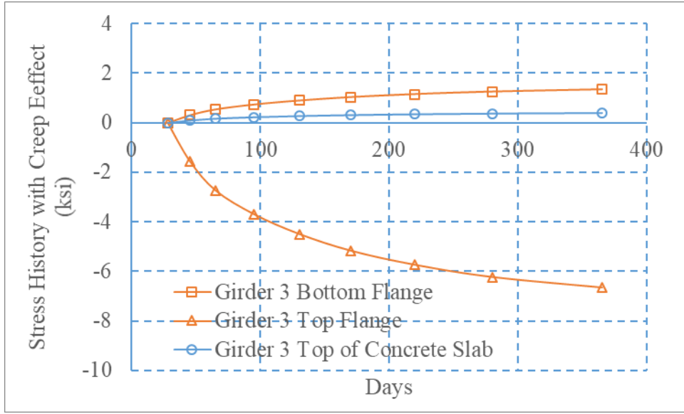
Figure 11-76. Time history for stress along longitudinal direction for girder #3 at midspan (creep effect, a 120 ft single span plate girder bridge with 10' spacing, five-girder system, shoring at 1/3 points)
