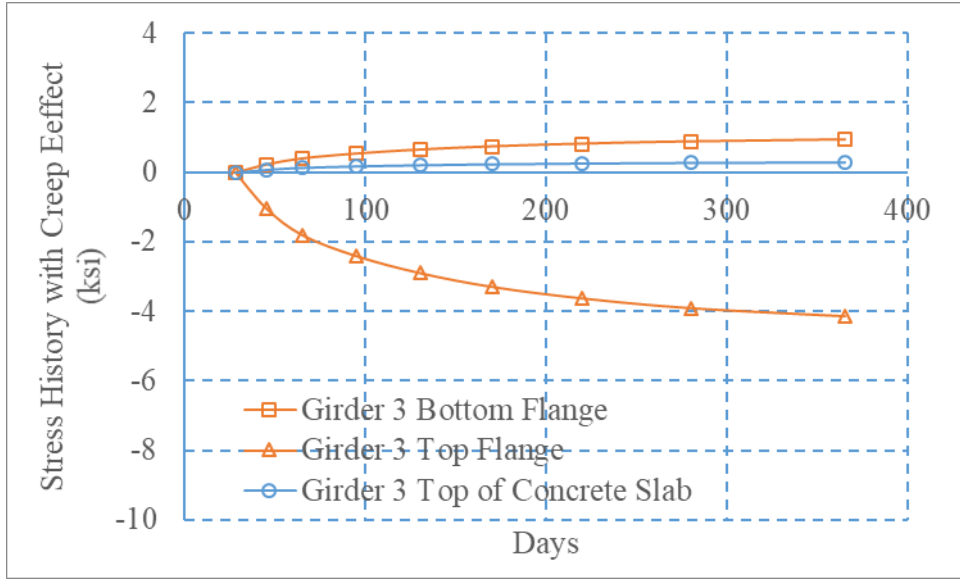
Figure 11-16. Time history for stress along longitudinal direction for girder #3 at midspan (creep effect, an 80 ft single span plate girder bridge with 10' spacing, five-girder system, shoring at 1/3 points)
