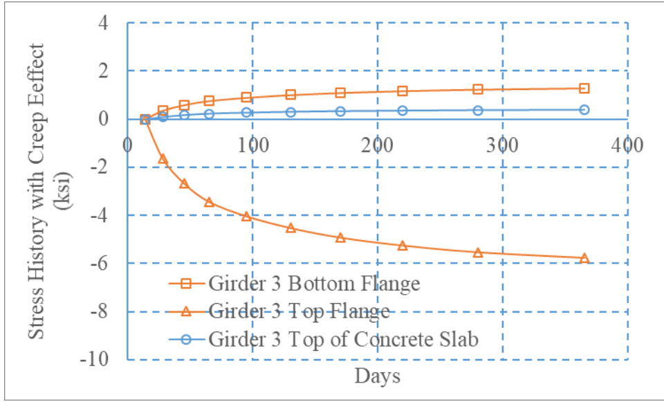
Figure 11-6. Time history for stress along longitudinal direction for girder #3 at midspan (creep effect, an 80 ft single span plate girder bridge with 10' spacing, five-girder system, unshored)
