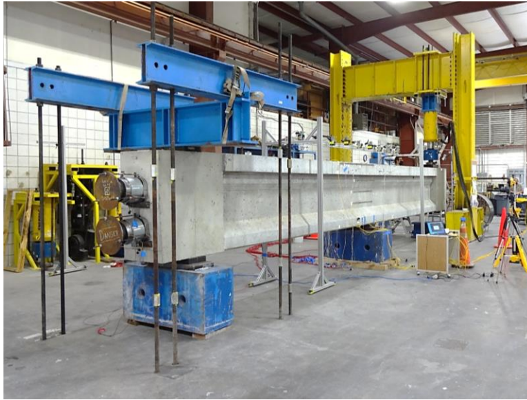
Figure E.23 Beam specimen NB-2 inside test frame and tie-down
