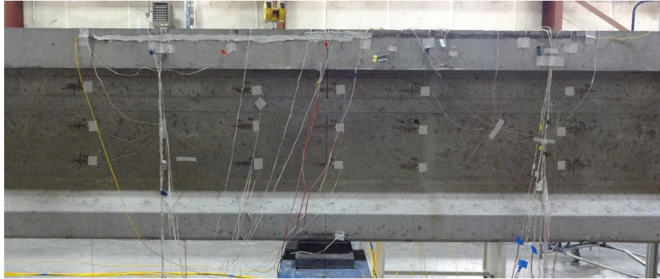
Figure 7.22 Typical 60-mm foil strain gages installed on NB precast specimens
