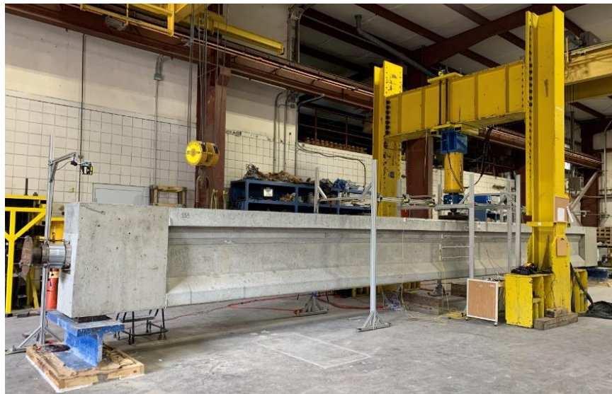
Figure C.27 Beam specimen SS-3 inside test frame
