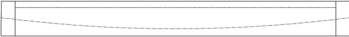
Figure 4.6 Parabolically draped tendon profile (F5) for precast simply-supported specimens (not to scale)
