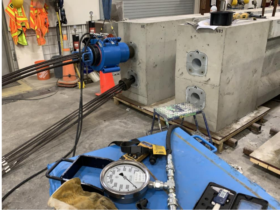
Figure 7.16 Post-tensioning of NB specimens
