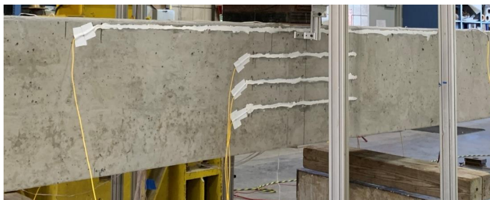
Figure 6.10 Fiber optic sensors installed on CIP beam specimen SS-5
