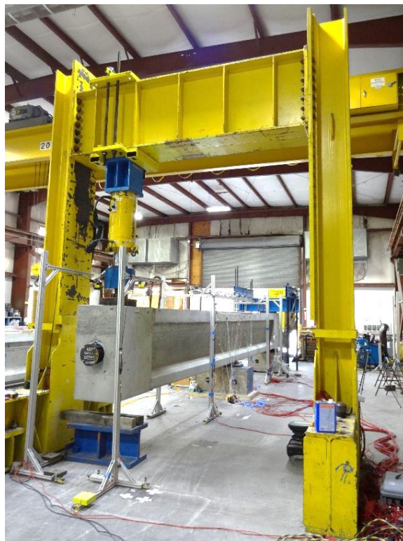
Figure E.5 Beam specimen NB-1 inside test frame
