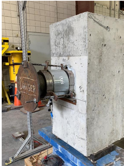
Figure 5.27 Geokon hollow-core load cell installed at dead end of beam specimen SS-3
