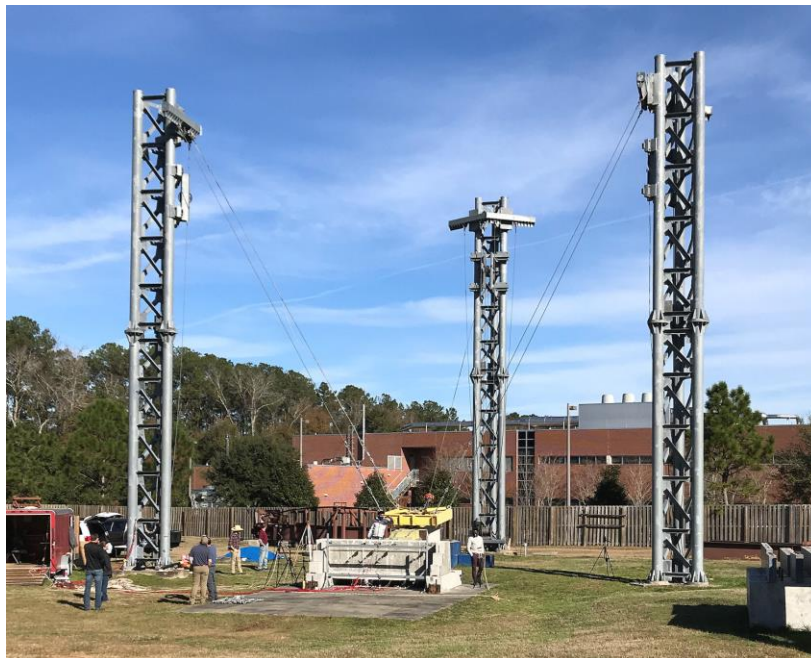
Figure 4.1 Pendulum at FDOT Structures Research Center (Tallahassee, FL)
