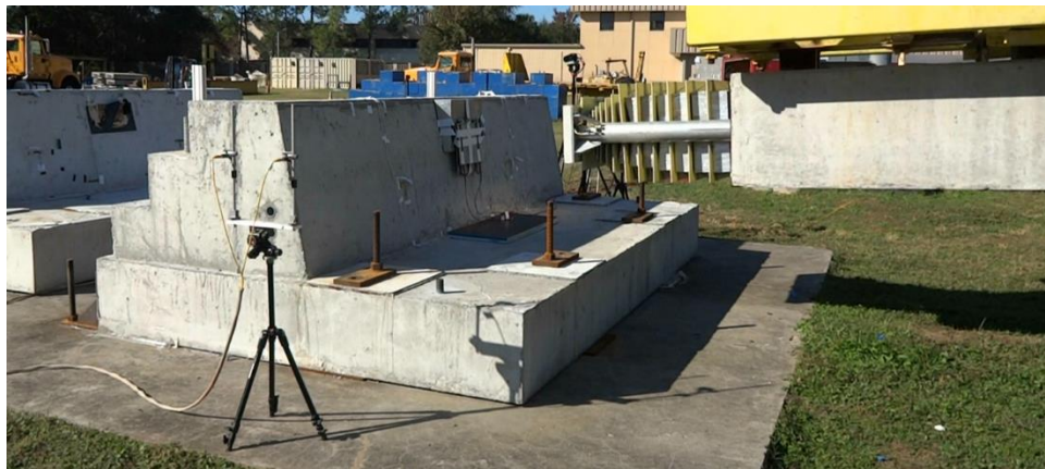
Figure 6.50 R/C COR test 2 specimen after completion of impact test
