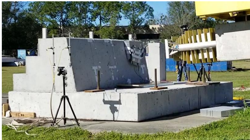
Figure 7.6 FRC EOR test 1 specimen after completion of impact test
