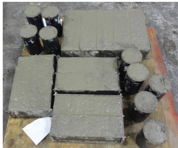
Figure 3.25 Additional trial FRC production specimens (4-in. x 4-in. x 14-in. flexural beams and 4-in. x 8-in. cylinders)
