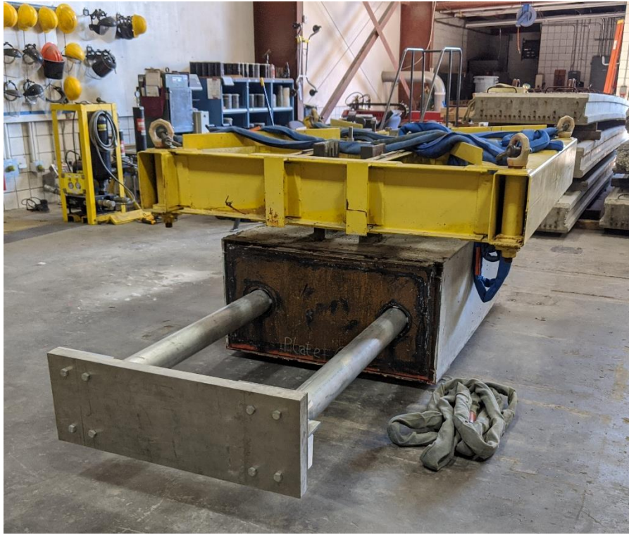
Figure 4.20 Complete pendulum impactor: Fabricated aluminum front nose placed inside the concrete block
