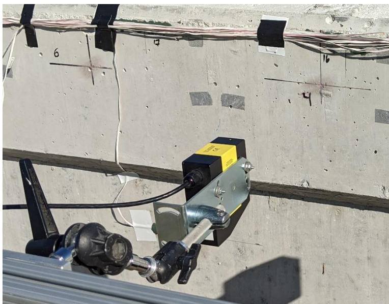
Figure 5.29 Laser displacement sensor mounted behind a test specimen
