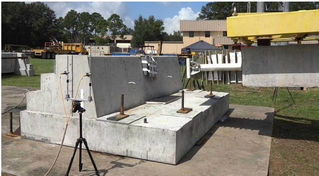
Figure 6.4 FRC COR test 1 specimen after completion of impact test
