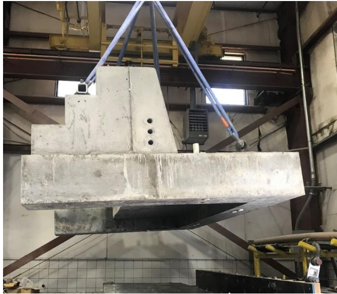
Figure 5.12 Test specimen lifted out of the formwork by crane
