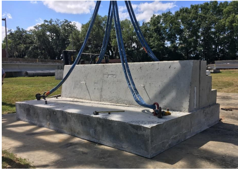
Figure 5.14 Impact test specimen in position on pendulum foundation
