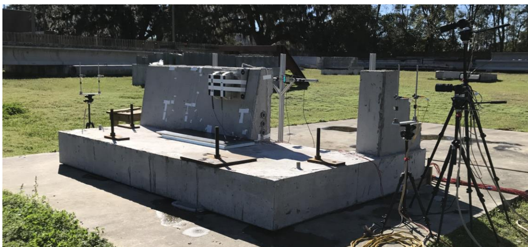
Figure 7.3 FRC EOR specimen prepared and ready for pendulum impact testing (with instrumentation in place)
