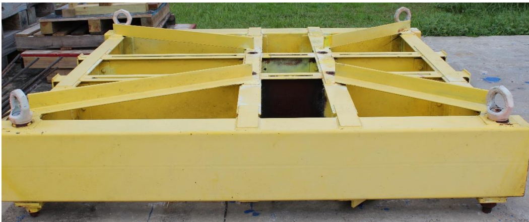
Figure 4.12 Repurposed steel hanger frame
