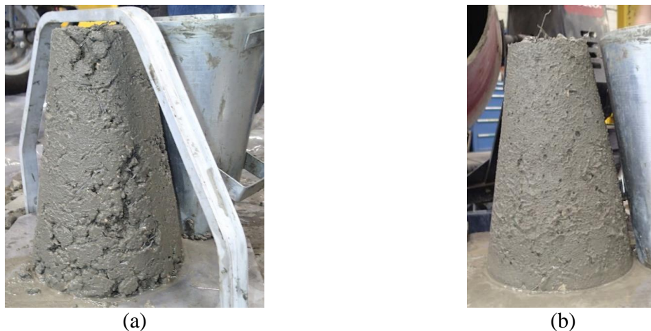
Figure 3.1 Slump tests for trial FRC production: (a) Standard (hand rodded) slump (measured 0.25-in. slump); (b) Slump with vibration (measured 0.0-in. slump)
