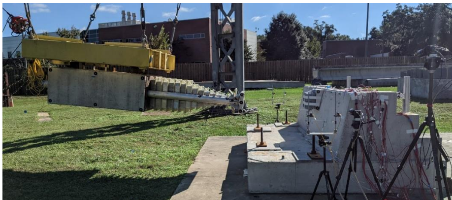
Figure 5.21 Pendulum impactor and impact test specimen prepared and ready for testing (with instrumentation in place)
