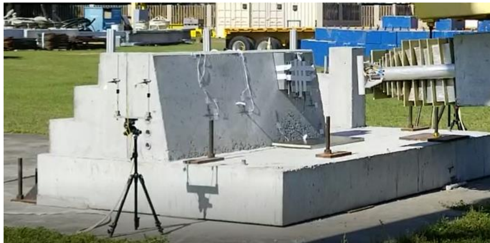
Figure 7.24 R/C EOR test 1 specimen after completion of impact test
