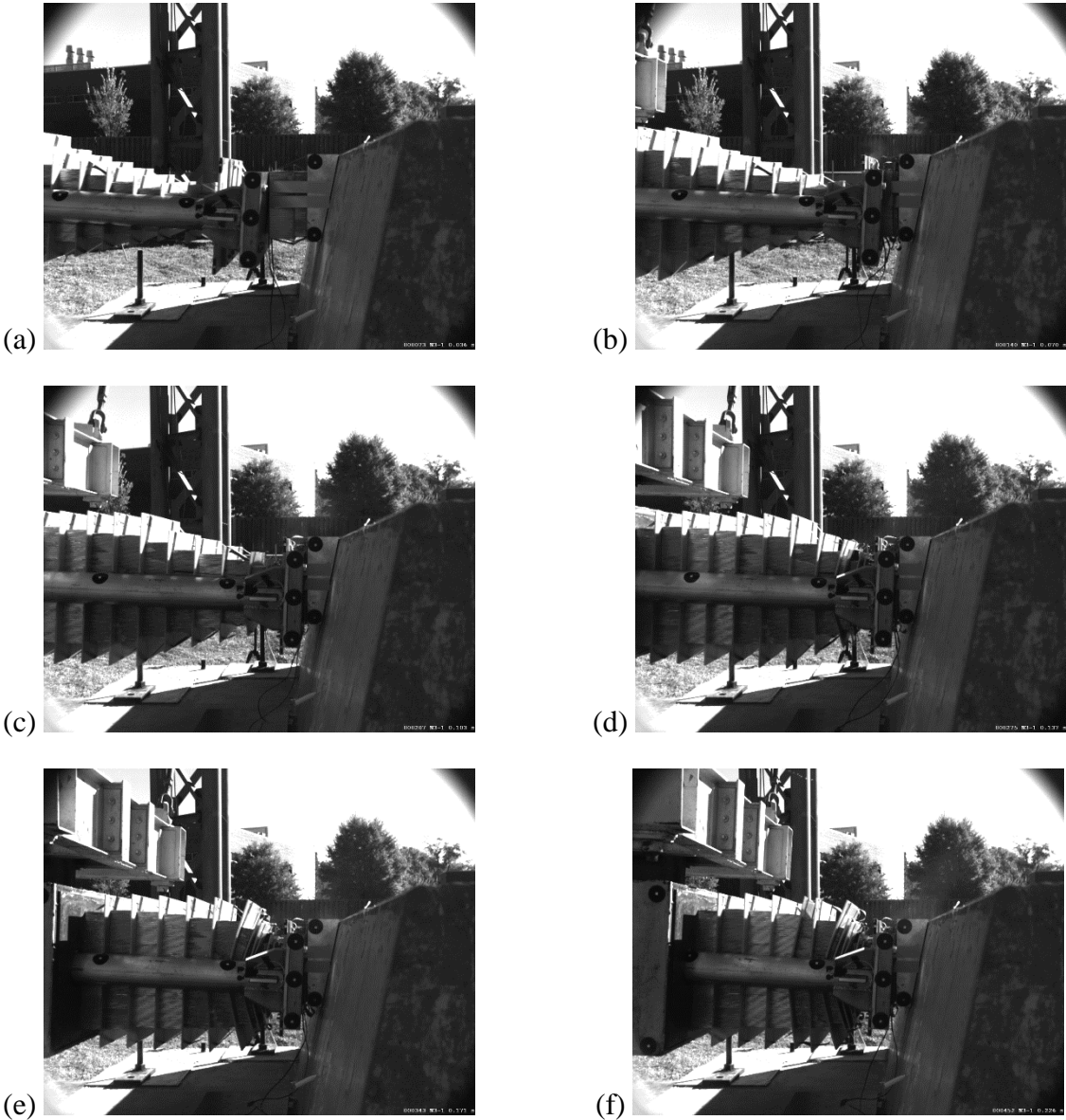
Figure 6.48 High-speed video frames from HSC-1 (R/C COR test 2) showing crush deformation of aluminum honeycomb: (a) At initial impact; (b) – (e) Intermediate frames; (f) At peak impact force
