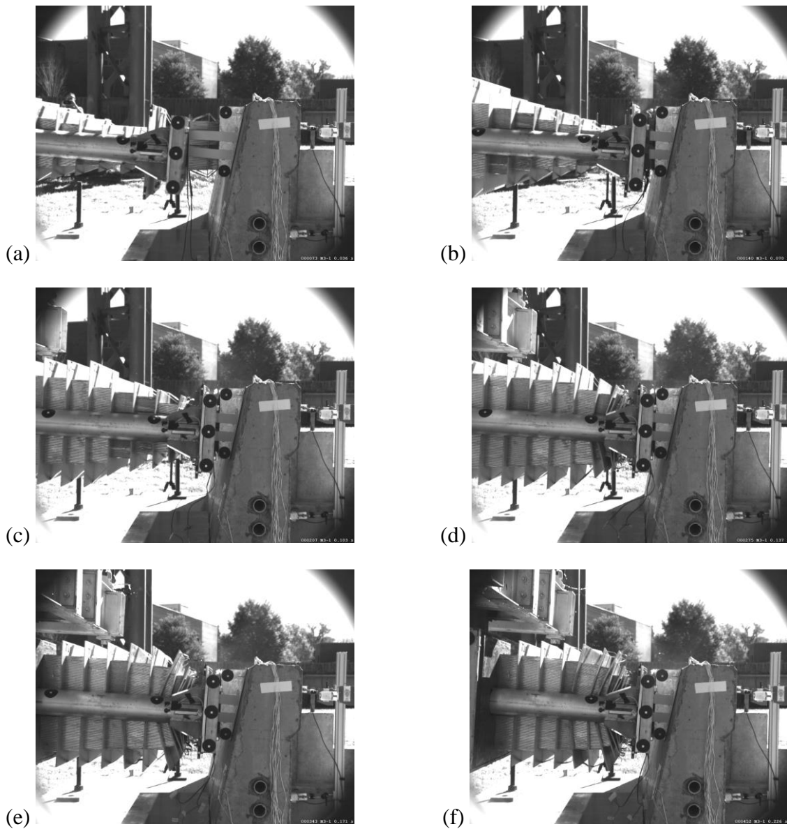
Figure 7.4 High-speed video frames from HSC-1 (FRC EOR test 1) showing crush deformation of aluminum honeycomb: (a) At initial impact; (b) – (e) Intermediate frames; (f) At peak impact force
