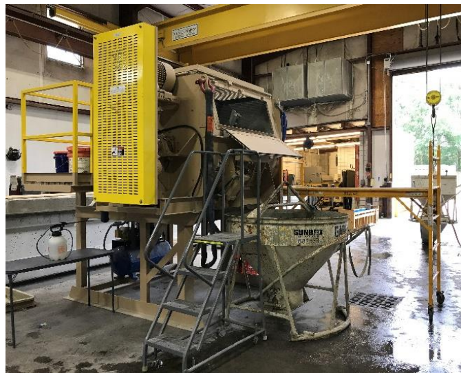
Figure 3.21 FDOT UHPC mixer used to introduce fibers into the concrete delivery truck mixture
