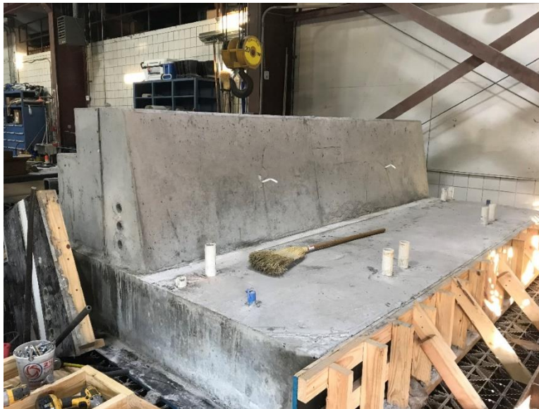
Figure 5.11 Completed (FRC) test specimen
