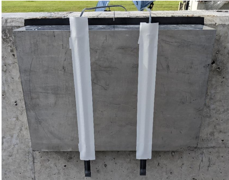
Figure 5.24 Tape switches adhered to the impact face of the aluminum loading wedge
