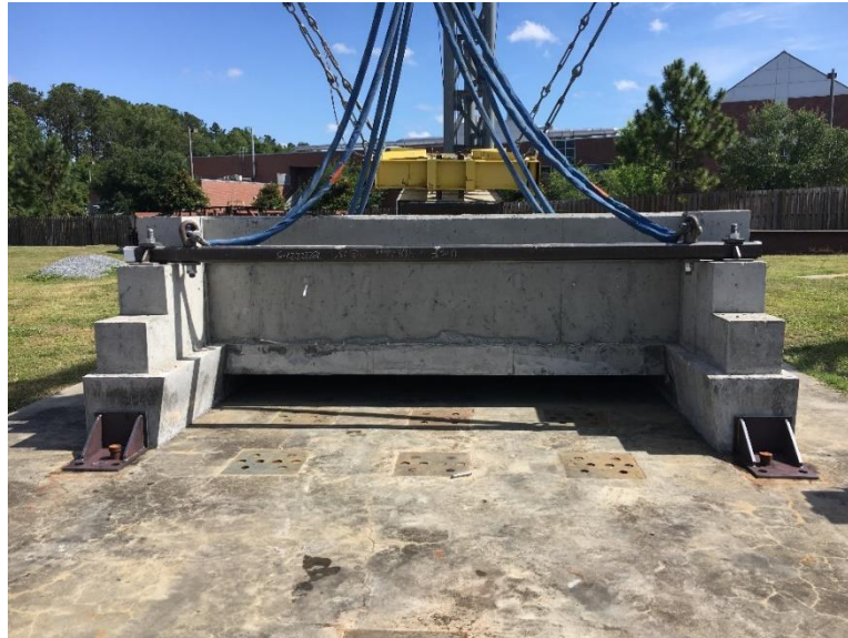
Figure 5.15 Backside of impact specimen after being positioned onto the pendulum foundation (with temporary HSS lifting element still connected)
