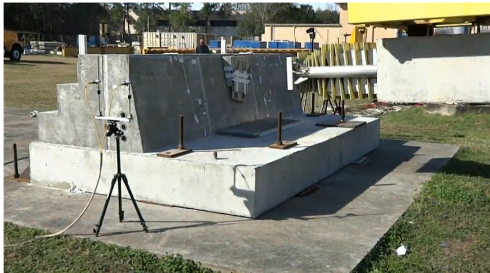
Figure 6.15 FRC COR test 2 specimen after completion of impact test
