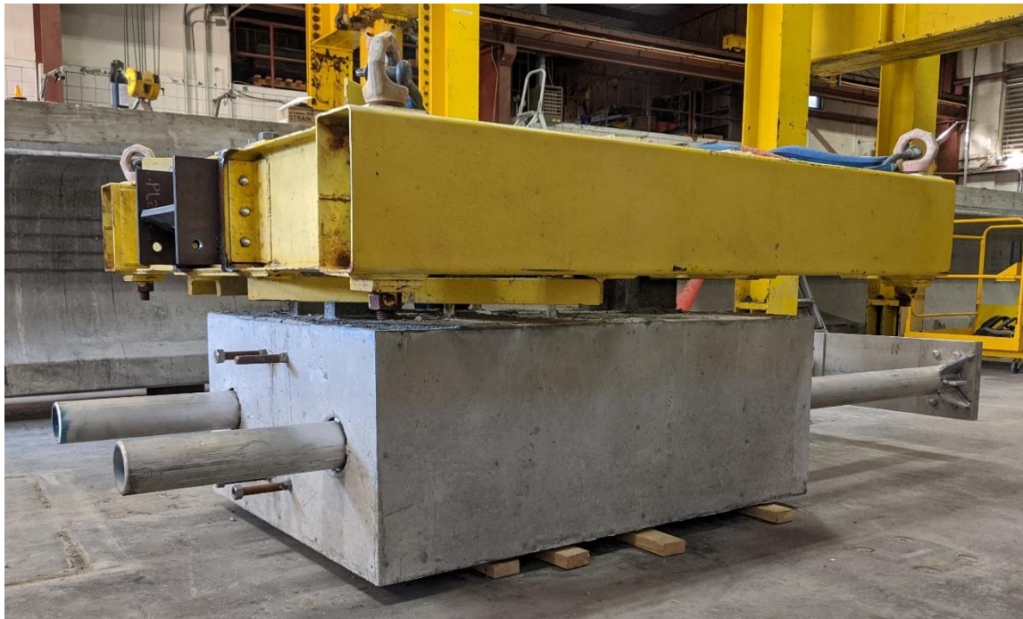
Figure 4.21 Complete pendulum impactor: Aluminum front nose placed inside the concrete block and the front nose tubes protruding out the back of the block
