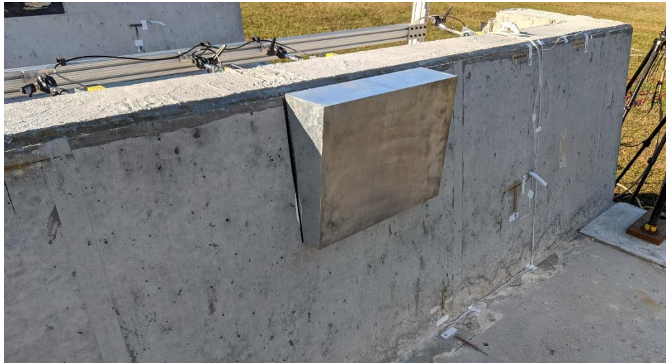
Figure 5.20 Aluminum loading wedge adhered to front face of railing
