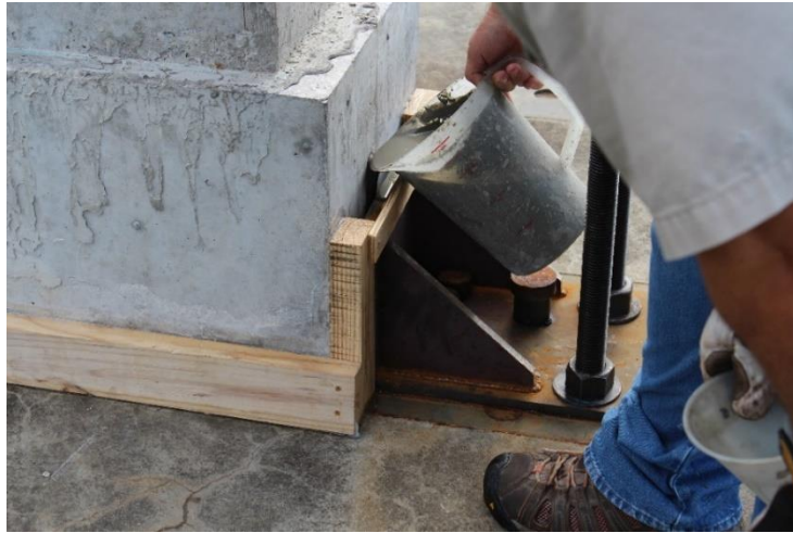
Figure 5.19 Placing grout between test specimen and small reaction element (steel slide stopper) as a secondary reaction system to prevent specimen from sliding during impact testing
