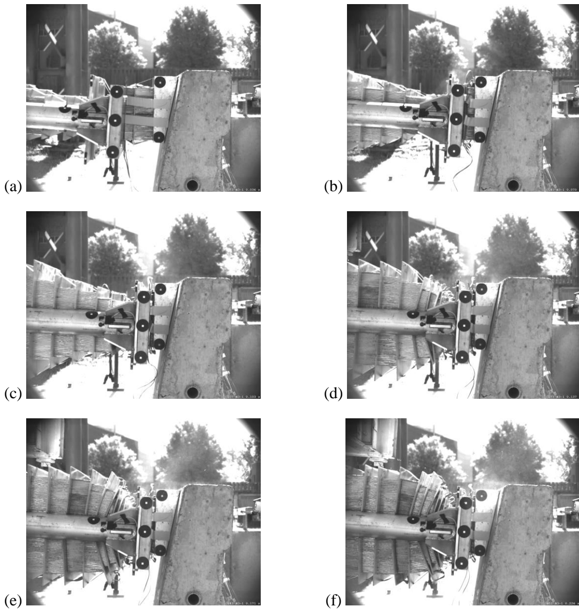
Figure 7.22 High-speed video frames from HSC-1 (R/C EOR test 1) showing crush deformation of aluminum honeycomb: (a) At initial impact; (b) – (e) Intermediate frames; (f) At peak impact force
