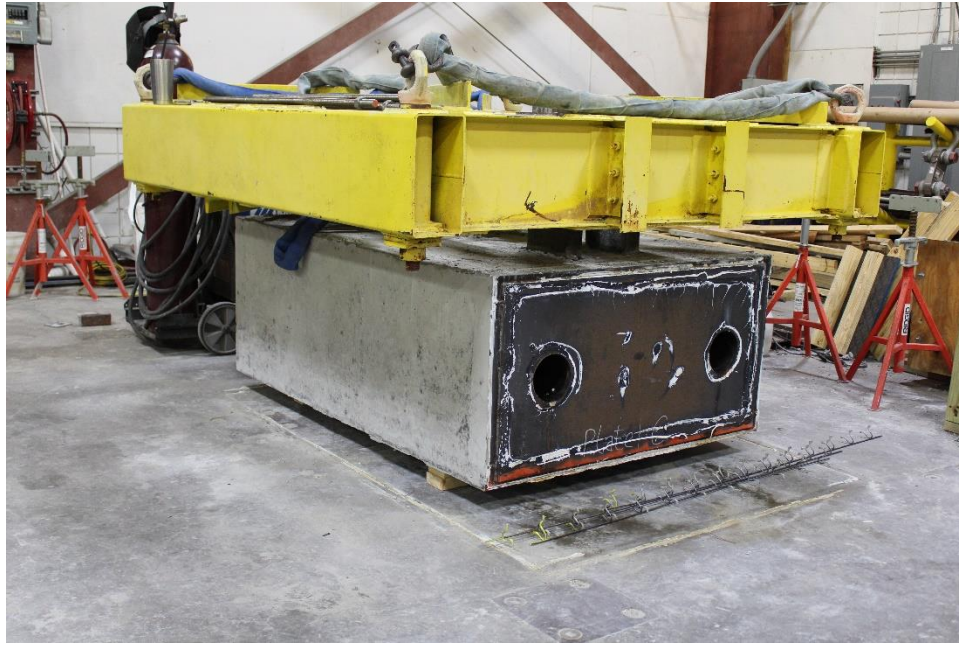
Figure 4.17 Formed concrete block connected to the steel hanger frame
