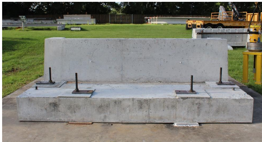
Figure 5.18 Anchored test specimen
