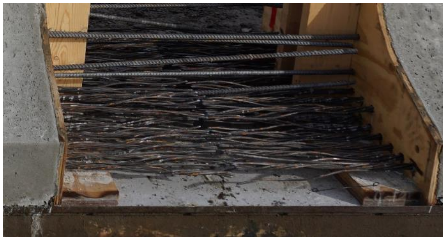
Figure 5-31 Fully cut strands
