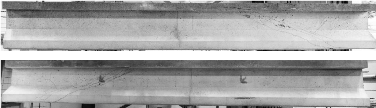
Figure 4-45 Specimen SS2 at end of destructive testing
