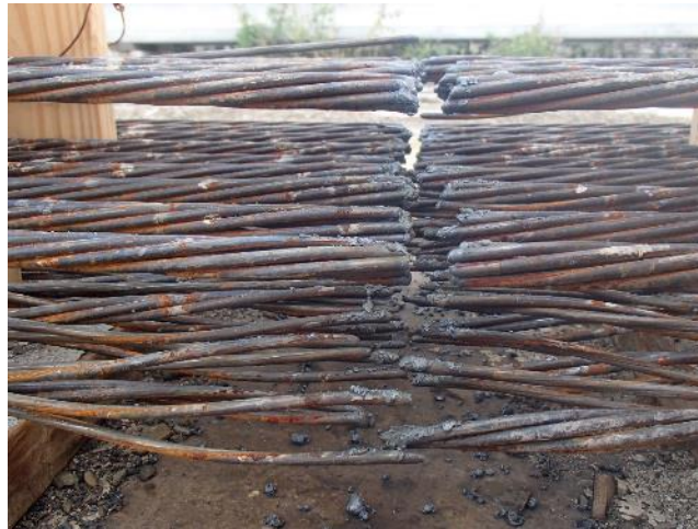
Figure 4-31 Fully cut strands
