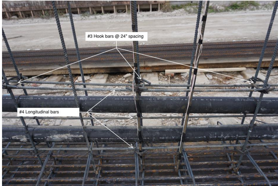
Figure 6-11 Specimen P50R SDG duct reinforcement.
