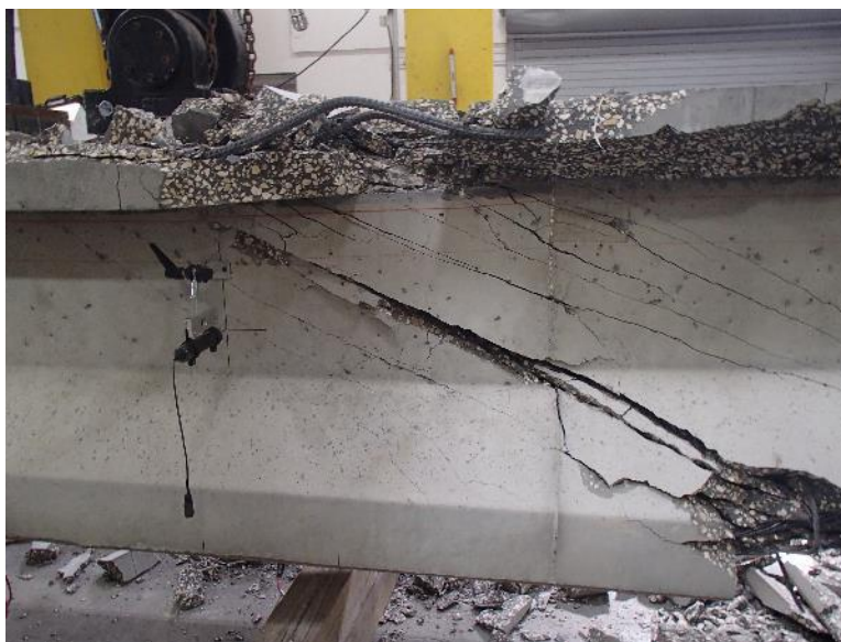
Figure 4-52 Shear failure of specimen SS4
