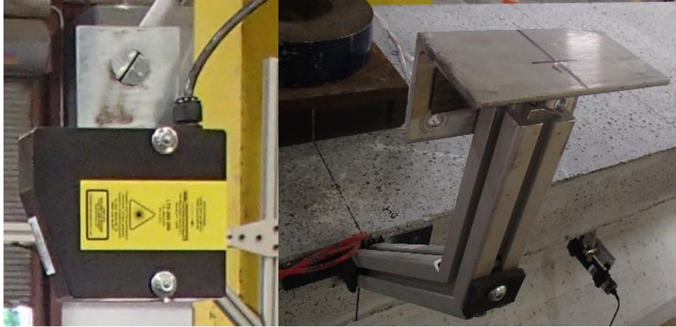
Figure 4-36 Laser displacement transducer
