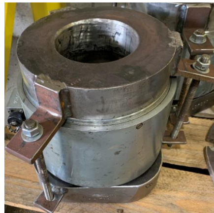
Figure 5-52 Load cell assembly with square bottom plate.
