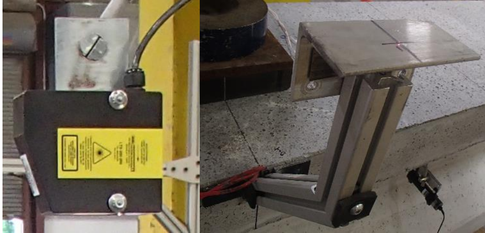
Figure 5-41 Laser displacement transducer
