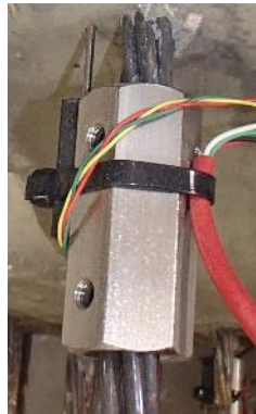
Figure 4-35 Linear potentiometer measuring strand slip
