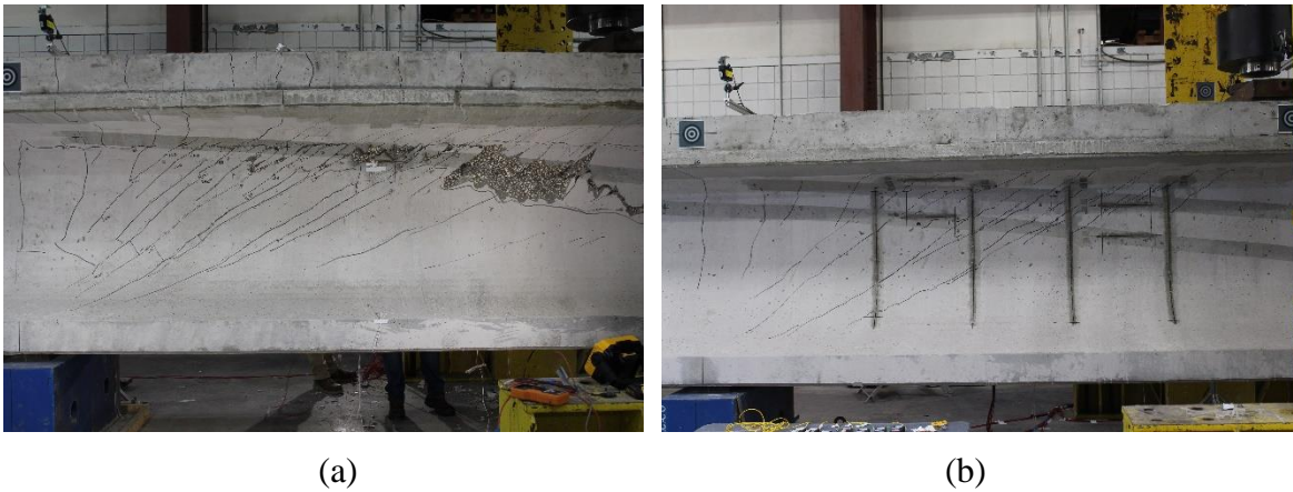
Figure 5-74 Concrete spalling at web after peak shear force and unloading (a) N50-1 (b) N50-2.
