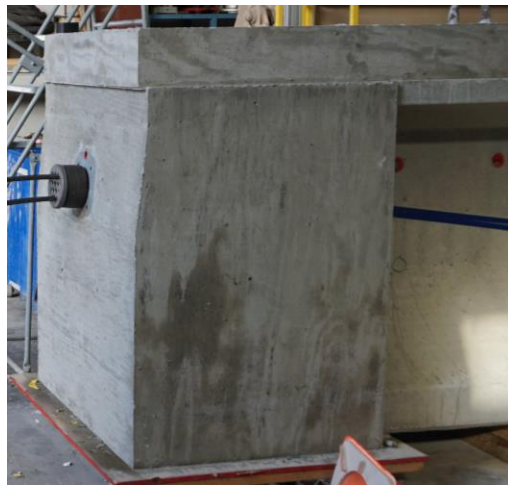
Figure 5-44 Anchor block and wedge plate at live end
