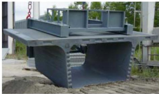
Figure 2.10 (a) General view of PS34 overpass (Resplendino 2008); (b) full-scale mock-up of a precast segment, with the scheme of extracted samples (AFGC recommendation 2013).
