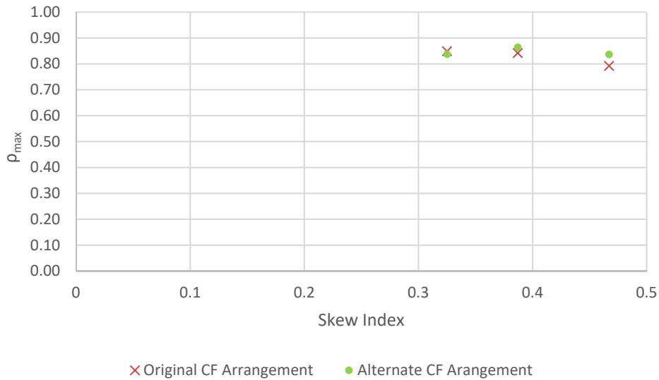
Figure 61. Comparison of \rho_{\max} values for STR I negative bending moments for central interior girders in bridges with original and alternate cross-frame arrangements.
