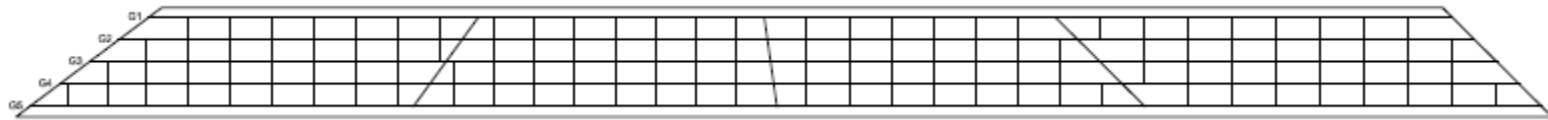
Figure 30. Bridge 15 (F57) ( L_s = 188 ft, 156 ft, 159 ft, 226 ft; w_g = 49.2 ft; \theta = 53.4^\circ, 36.2^\circ, 8^\circ, 45.3^\circ, 45.3^\circ ; I_s = 0.32 ; O_{min}/b_f = 1.45 ).
