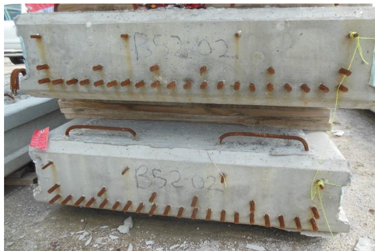
Figure 7 Slab Storage at the Precast Yard, End View
