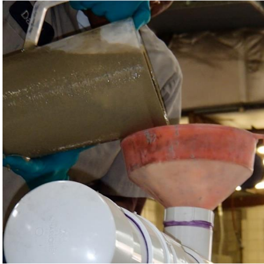
Figure 6-6. Grout mixture placed into specimen through funnel and PVC tee
