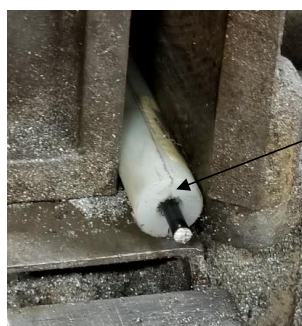
Figure 12-2. RE clamped in horizontal saw
