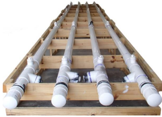
Figure 6-1. Fully assembled specimens with downward angle of PVC tee
