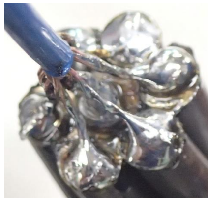
Figure 12-4. Wire soldered to end of 7-wire prestressing strand.
