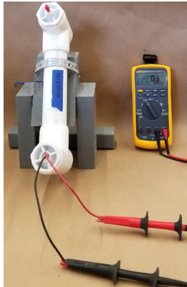
Figure 15-1. Corrosion potential measurement during drying
