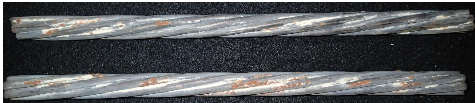
Figure 8-14. Corroded strands near port C dried ISG specimen
