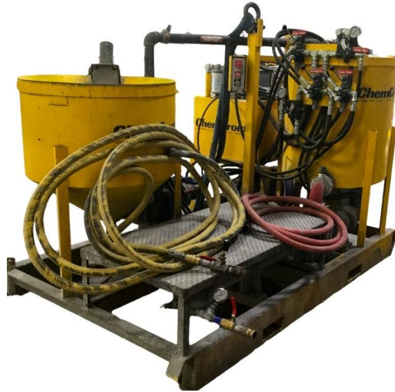
Figure A.3-3. Grout Plant
