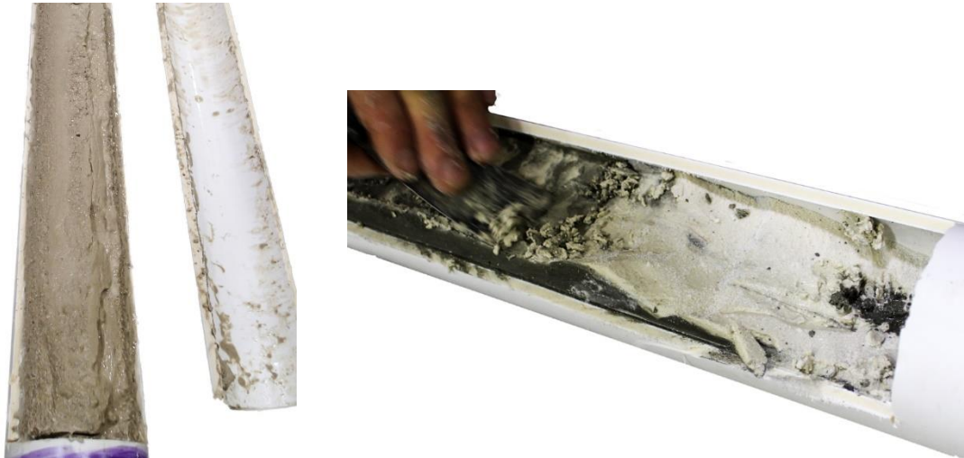
Figure A.3-9. Verification of soft grout
