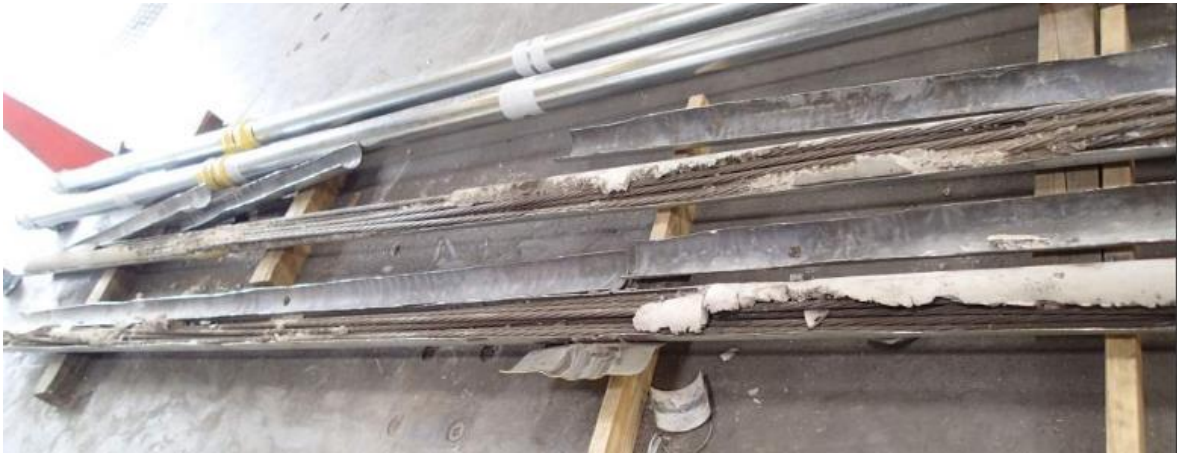
Figure A.3-15. EMT1 and EMT2 after hydrodemolition
