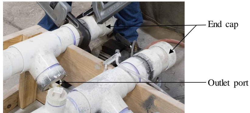
Figure 8-9. End caps and outlet port on specimens
