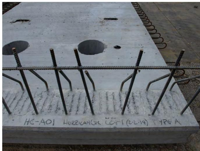
**Fig. 3-33. Markings of Precast Panel Number and Casting Date**
