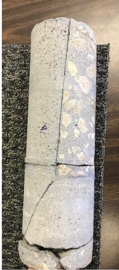
Fig. 6-29. Core 7, Showing Core through Panel and Shear Pocket and into Girder Top Flange
