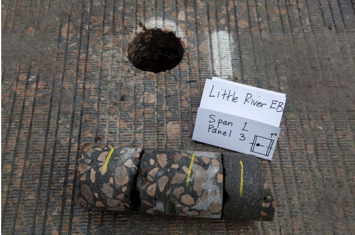
Fig. 6-3. Core 1, Little River EB, Span 1, Panel 3 (in Panel) (1)
