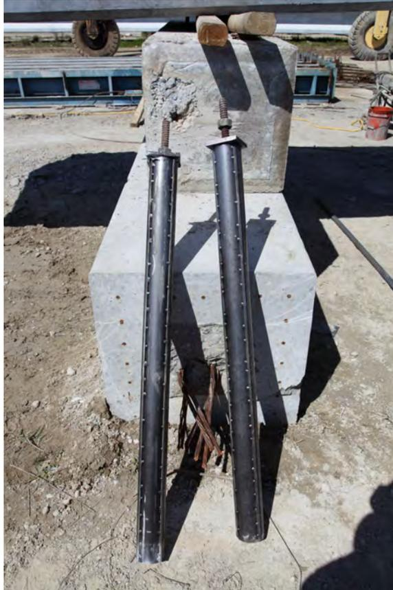
Fig. 6-14. Precast Bent Cap, Pipes for Stabilizing Dowel Bar Duct Forms (Two Shown)
