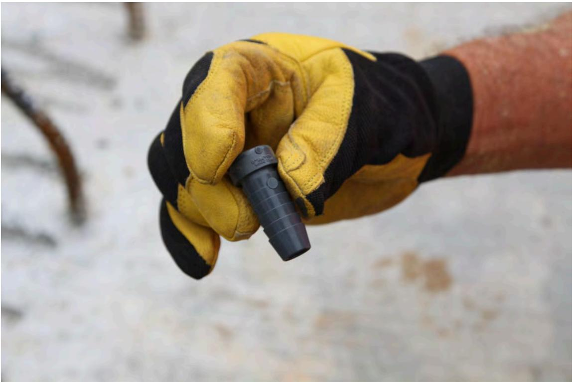
Fig. 4-18. Plug for Grout Port
