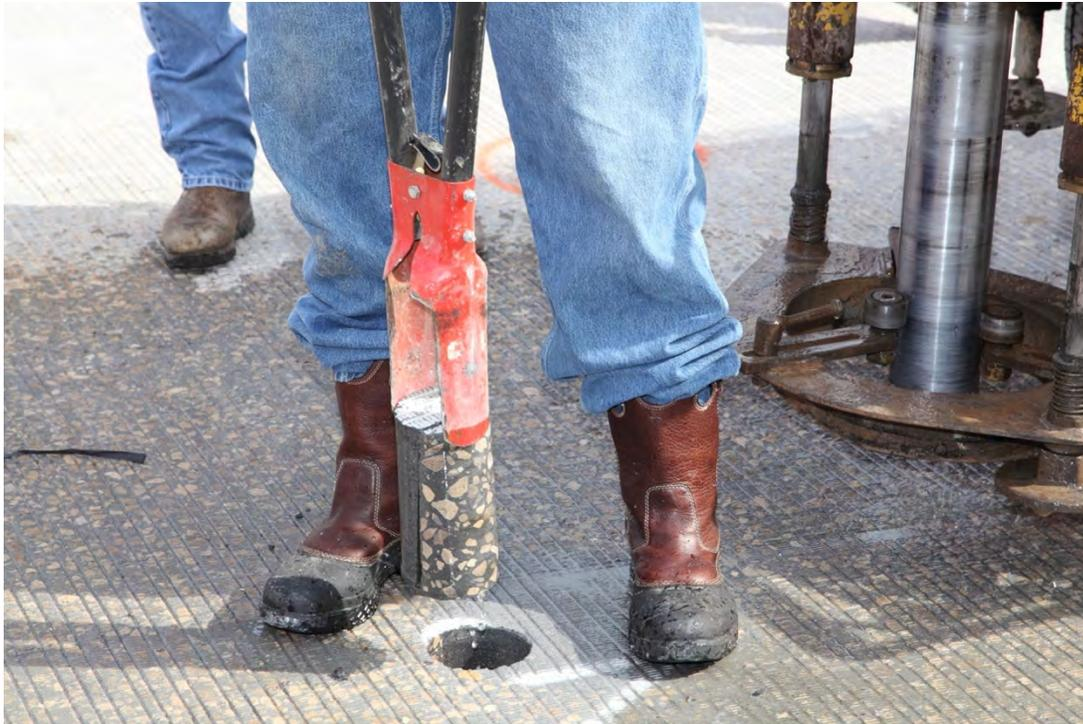
**Fig. 6-2. Core Being Pulled from Deck Panel**
