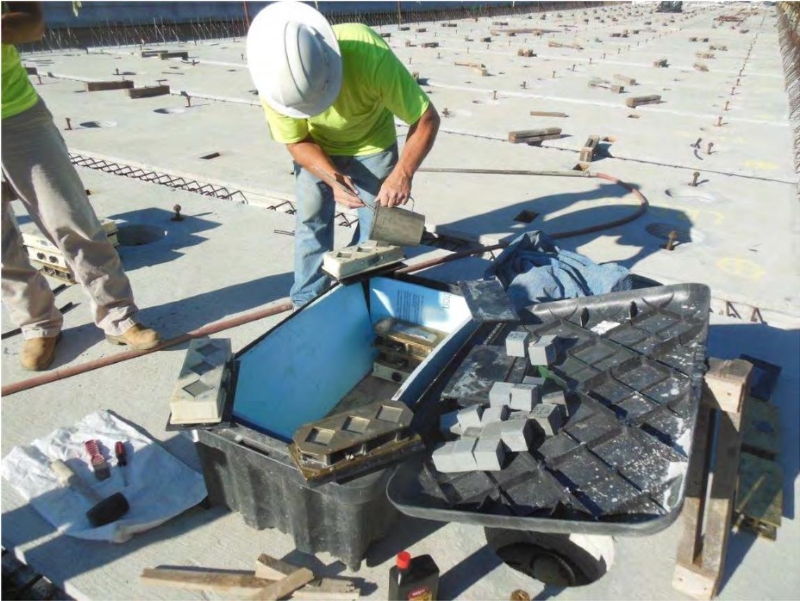
**Fig. 4-32. Making Grout Cubes for Testing**
