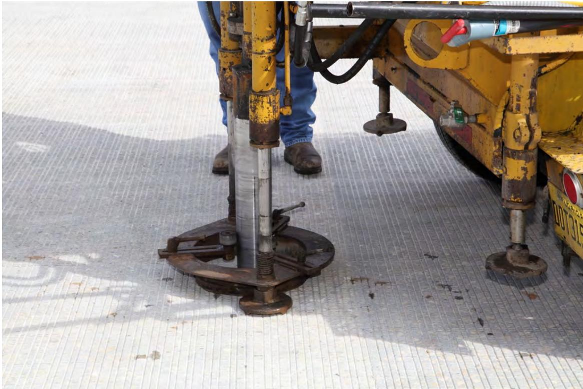
**Fig. 6-1. Coring Machine for Extracting Concrete Samples**
