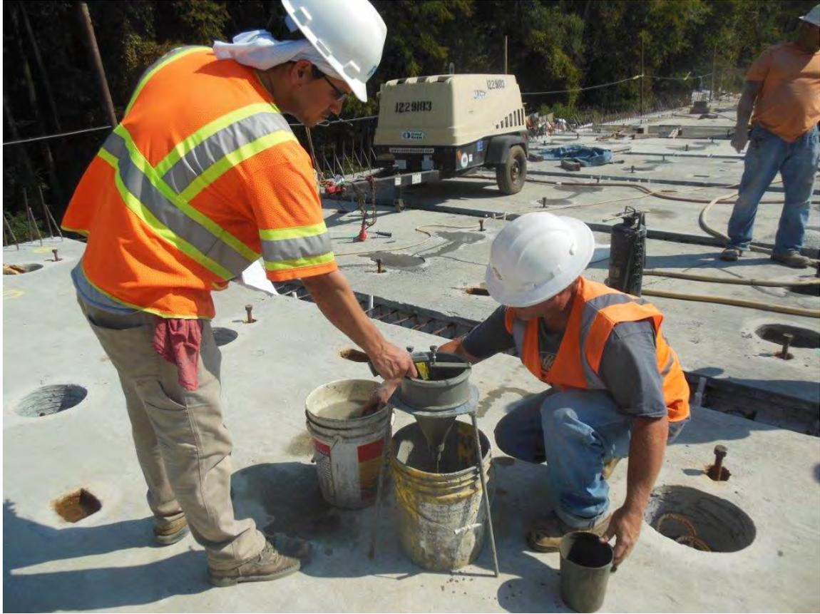
Fig. 4-30. Measuring Efflux of Grout
