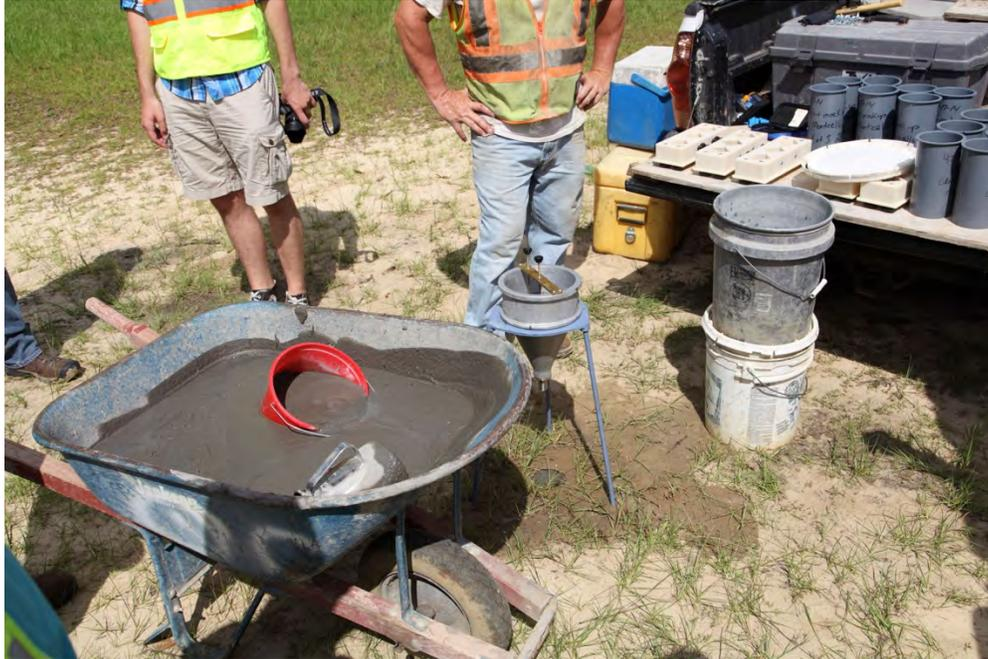
Fig. 5-9. Grout Testing Setup
