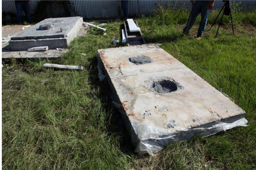
**Fig. 5-19. Grout Mock-up for Precast Deck Panel, “Panel” Removed for Grout Inspection (“Panel” Is Flipped Over in Foreground; “FIB” and Grouted “Haunch” Are in Background)**
