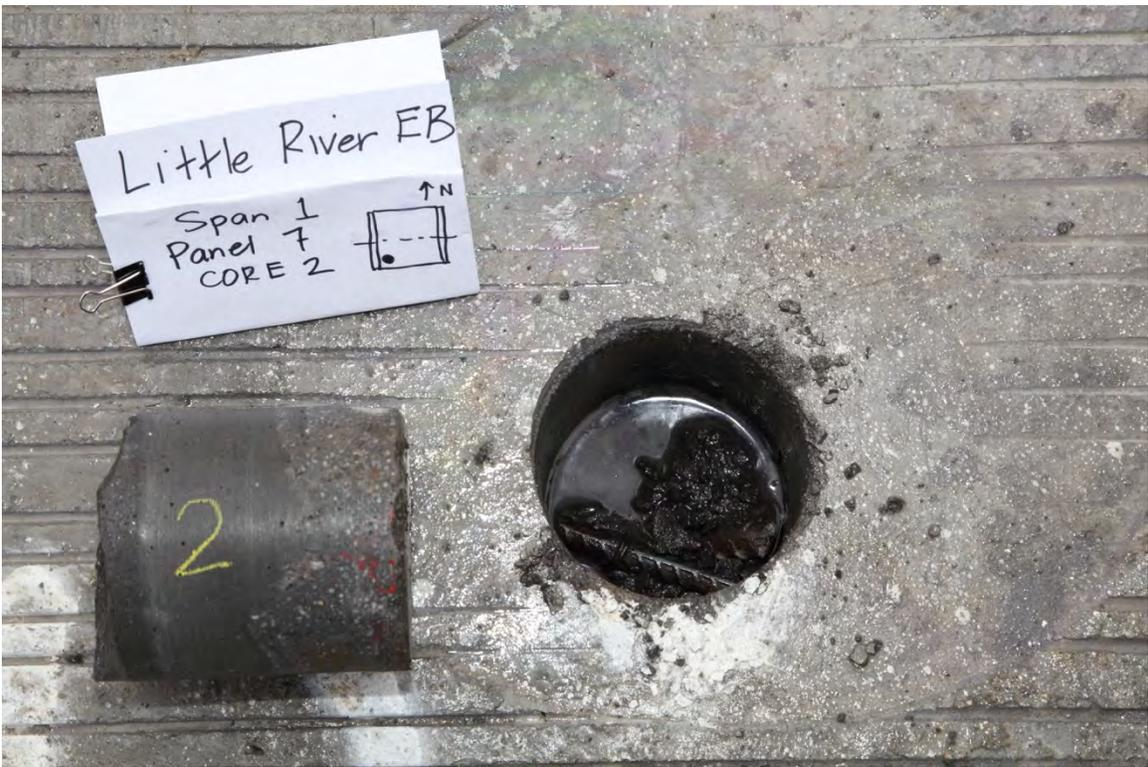
Fig. 6-6. Core 2, Little River EB, Span 1, Panel 7 (Shear Pocket-to-Panel Interface) (1)
