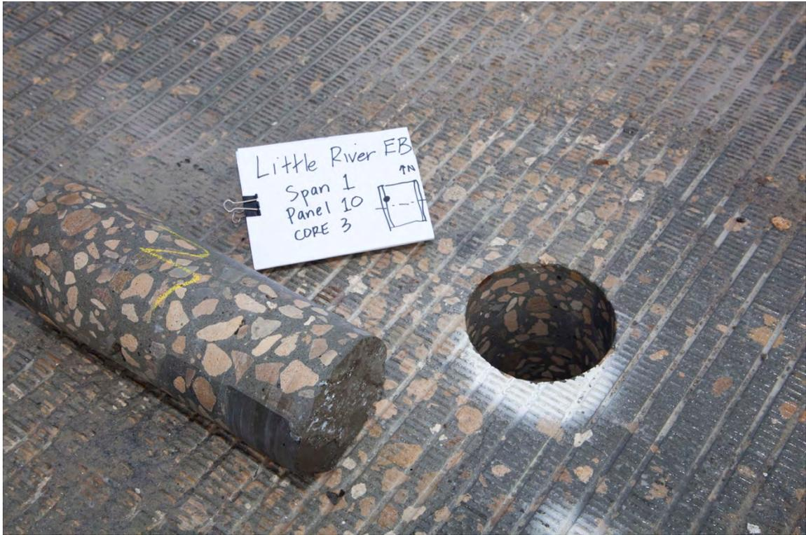
Fig. 6-9. Core 3, Little River EB, Span 1, Panel 10 (Closure Joint-to-Panel Interface) (1)
