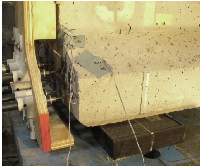
Figure 10–Specimen on bearing pad
