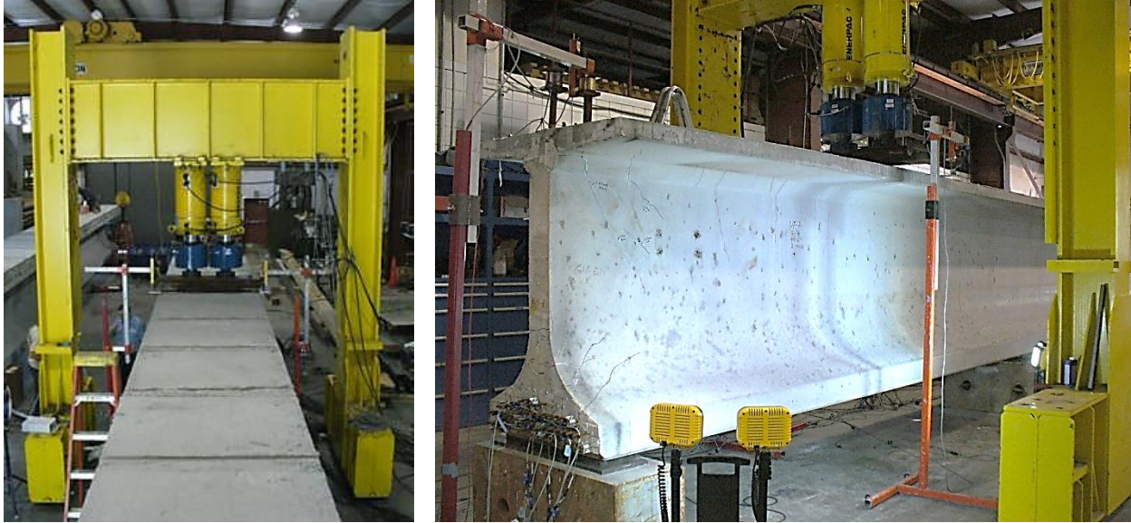
Figure 32–View of test specimen and load frame from above (left) and side view of specimen (right)
