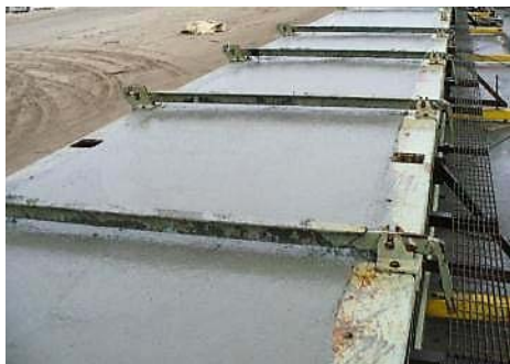
Figure 23–Top flange finish (left) and tarp covers (right)
