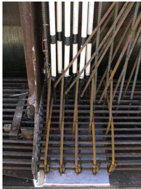
Figure 18—Top (left) and bottom (right) of post-tension rods in specimen PT
