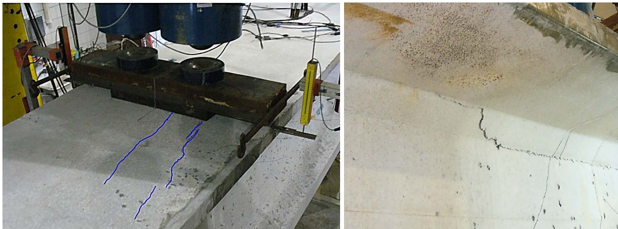
Figure 77–Punching failure from above (left) and below (right)
