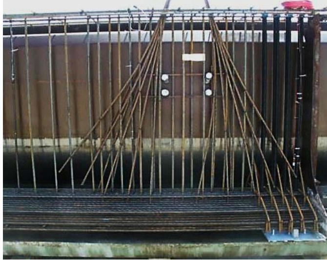
Figure 17—Specimen LB reinforcement
