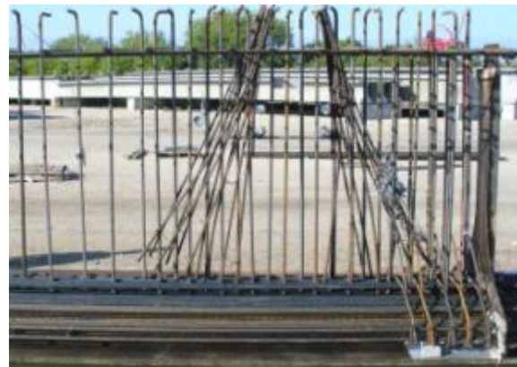
Figure 22–Girder F reinforcement A) Specimen FN and B) Specimen FB
