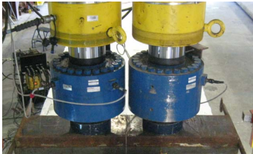
Figure 50–Load cells below hydraulic actuators
