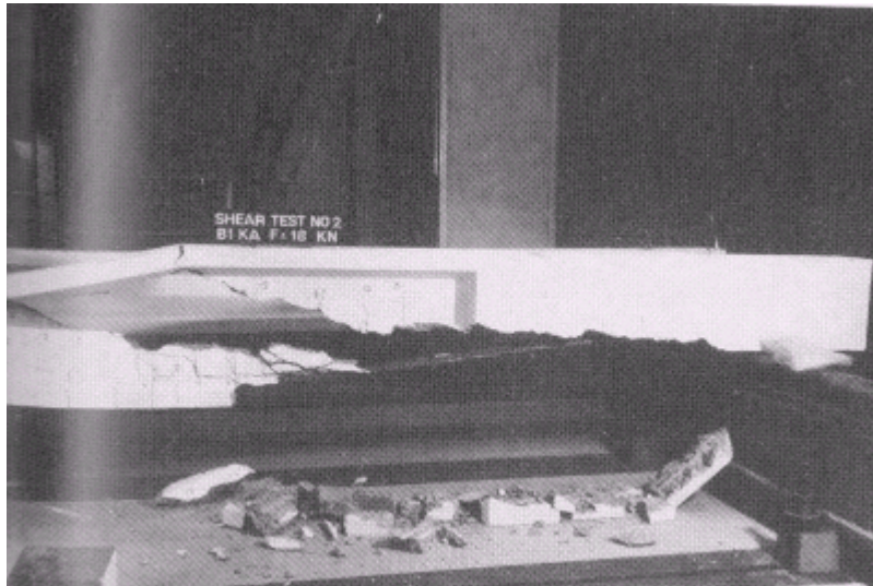
Figure 22–T-beam failure after tied-arch behavior
