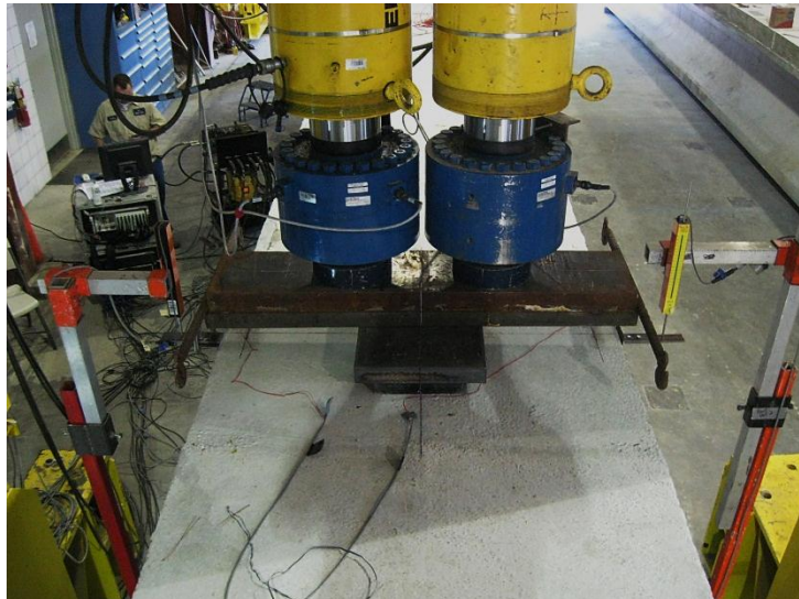
Figure 31–Support conditions at load point for specimens CT, SL, and PT
