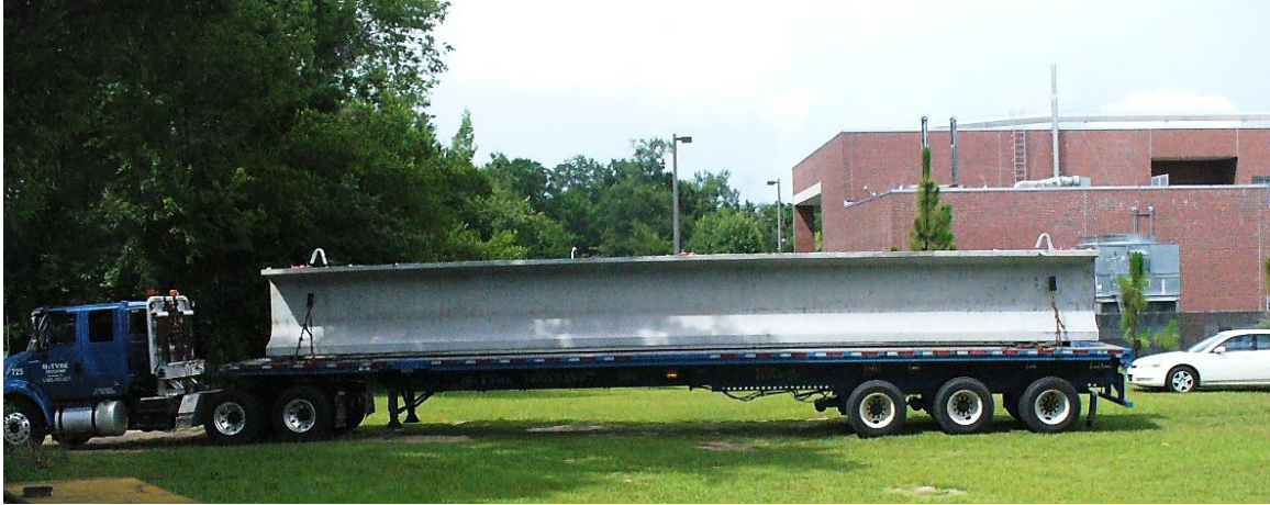
Figure 27–Test girder transported by truck
