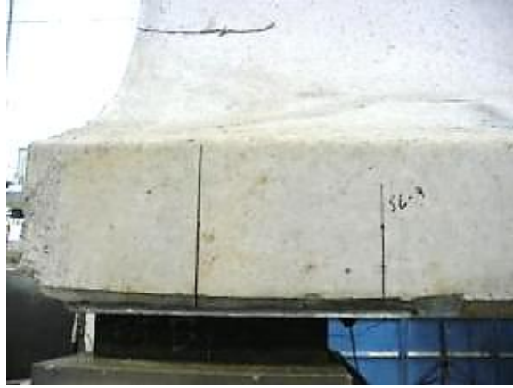
Figure 29–Support conditions at bearing
