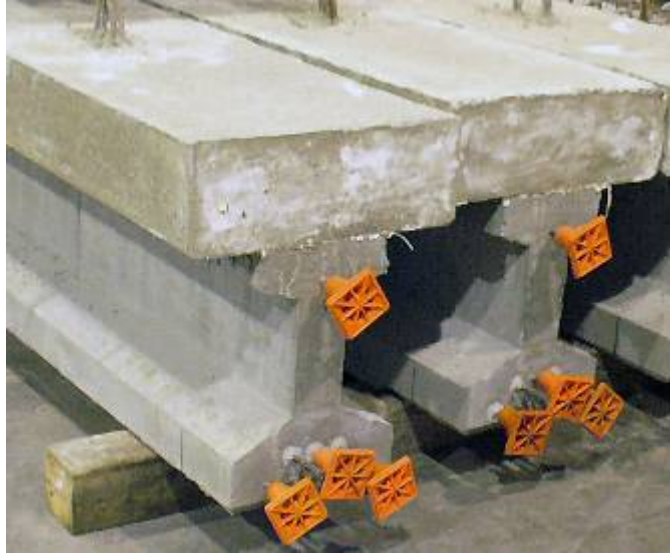
Figure 7–Finished beam specimens ready for testing
