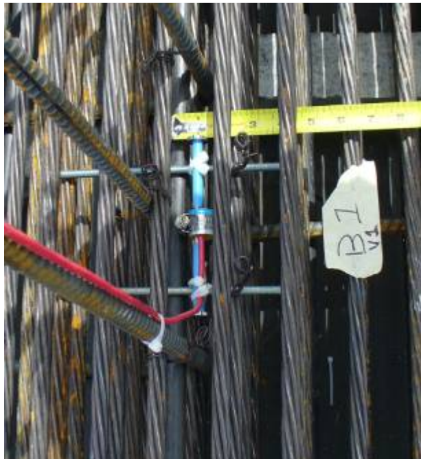
Figure 37–V gage installation (view from above)
