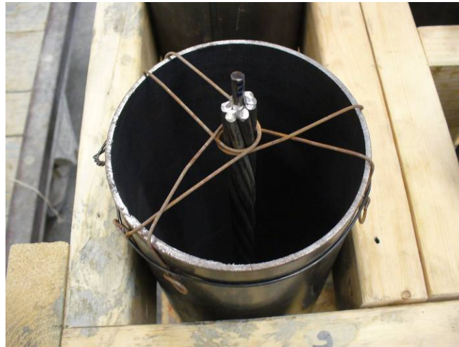
Figure 29–Stand lateral support at top of tube
