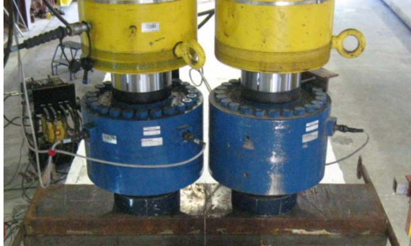
Figure 43–Load cells below hydraulic actuators
