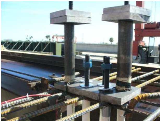
Figure 18—Top (left) and bottom (right) of post-tension rods in specimen PT
