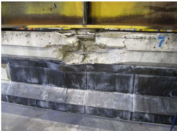
Figure 4-45: Failure of full-scale PSC girder by static testing
