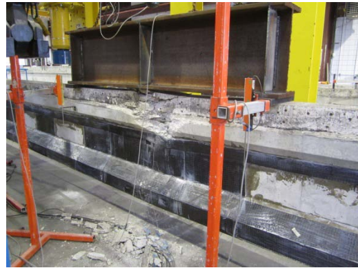
Figure 9-6: Girder failure under loading
