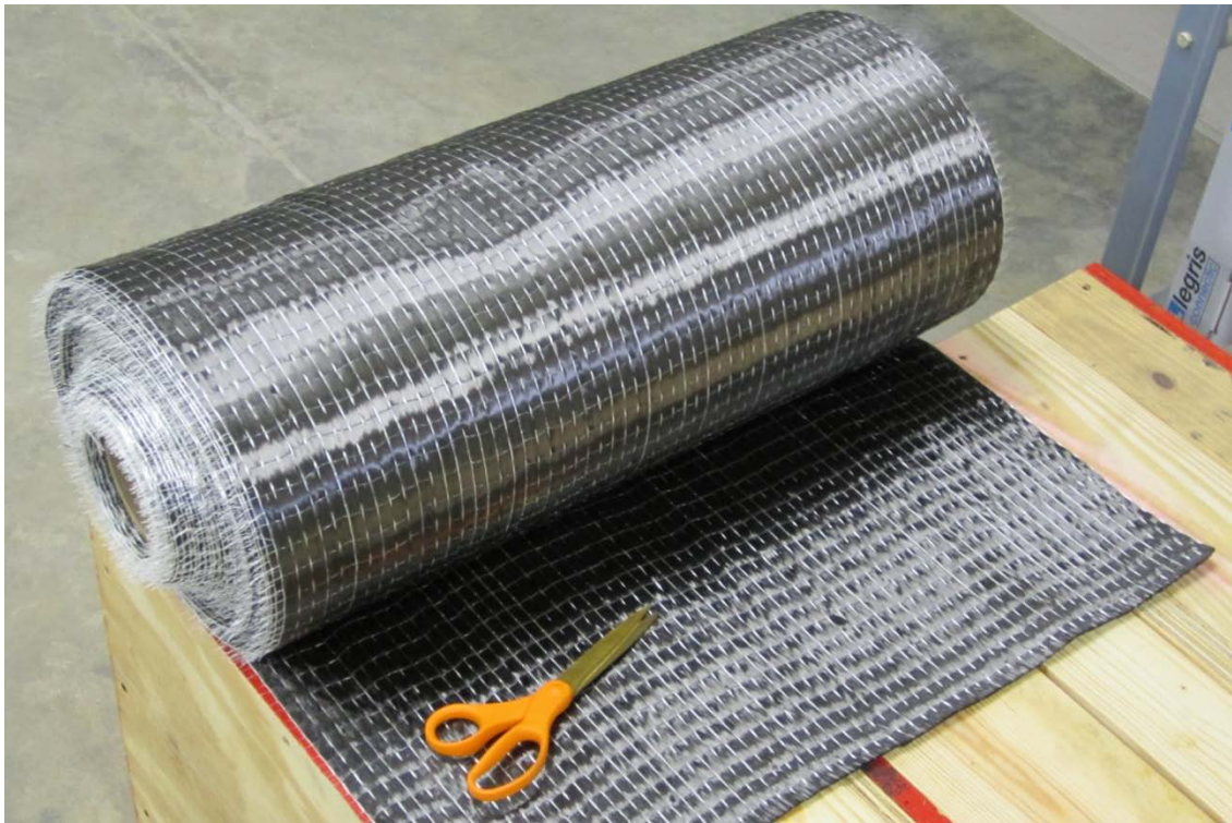
Figure 3-1: Picture of carbon fiber fabric material used in test specimen
