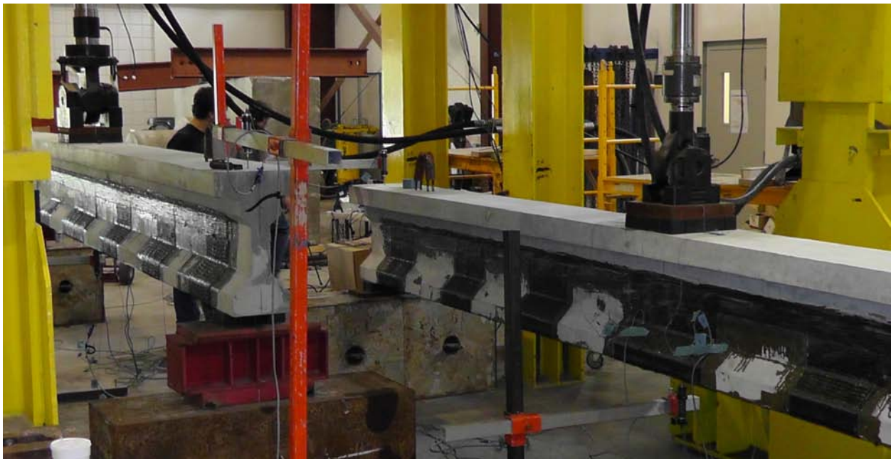
Figure 3-23: Fatigue loading setup arrangement for half-scale PS girders
