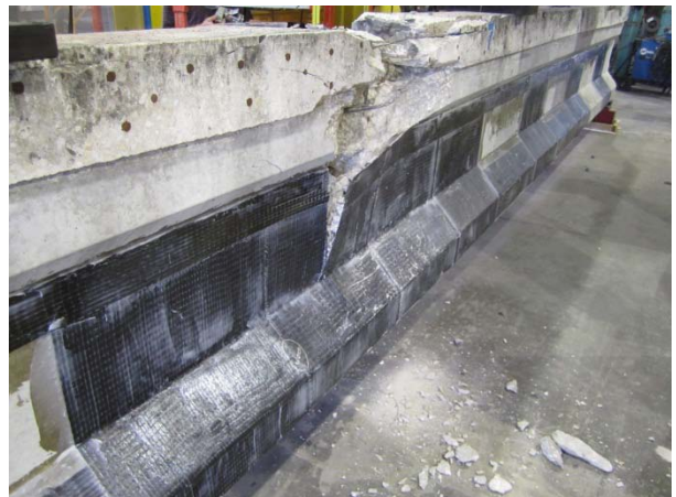
Figure 4-44: Failure of full-scale PSC girder by static testing
