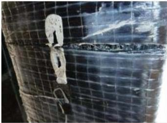
Figure 4-24:(left) Rupture of longitudinal CFRP, (right) Debonding of CFRP U-wrapping
