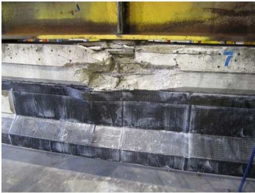
Figure 9-6: Girder failure under loading
