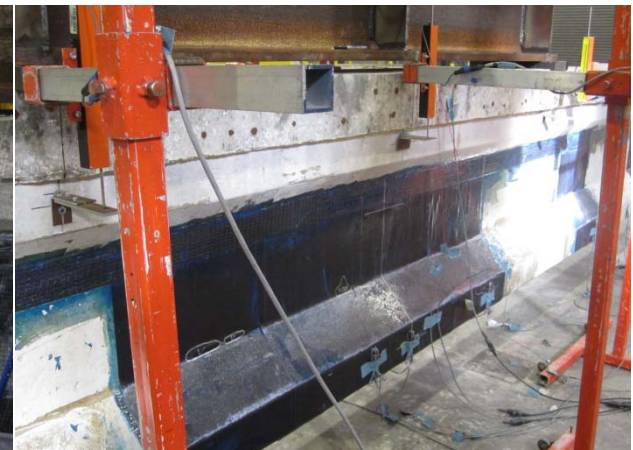
Figure 4-45: Failure of full-scale PSC girder by static testing
