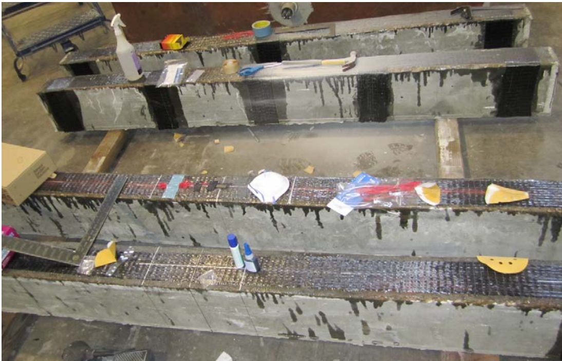
Figure 3-14: Picture of CFRP repairs applied to RC beam specimens
