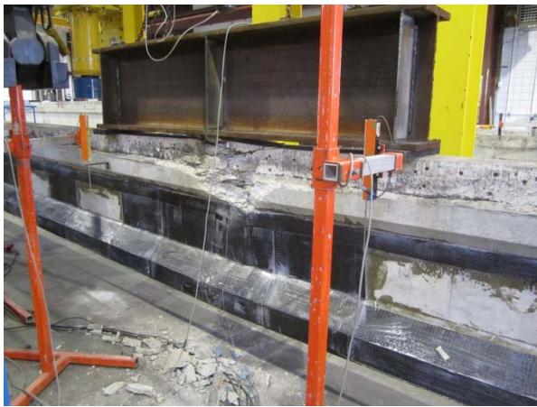
Figure 4-44: Failure of full-scale PSC girder by static testing
