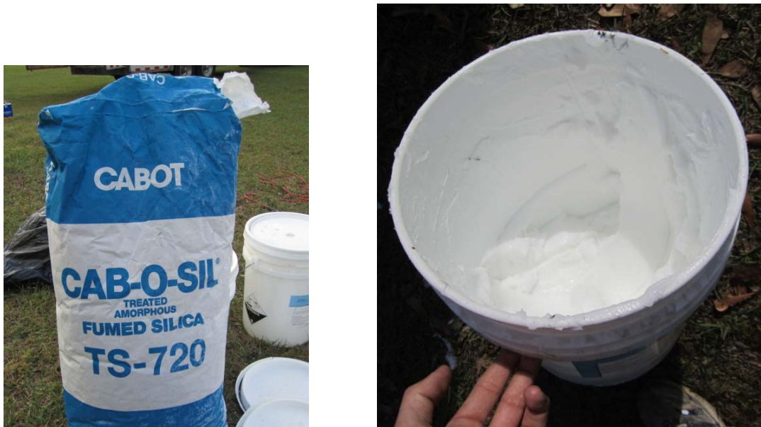
Figure 3-15: (left) Fumed silica used to thicken epoxy; (right) Thickened epoxy
