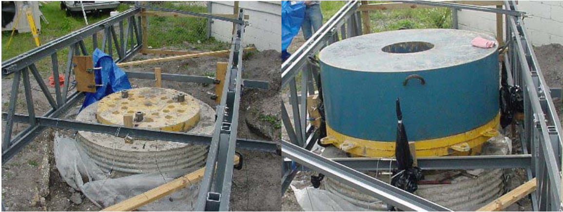
Figure 141 Load cells, LVDTs, steel plates (bottom and top), and seating weight
