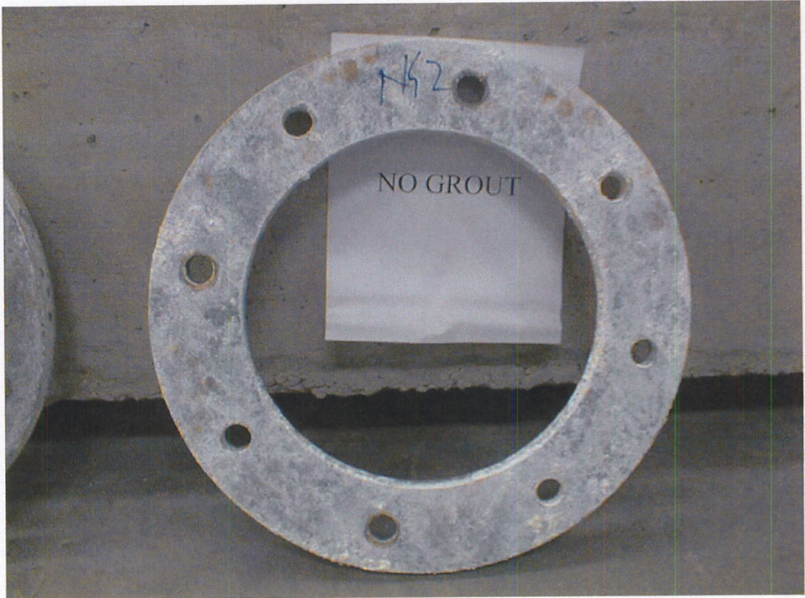
Figure 5.14 : Picture Of Galvanized Plate From Base Plate Arrangement With Out Grout Pad After 14 Weeks
