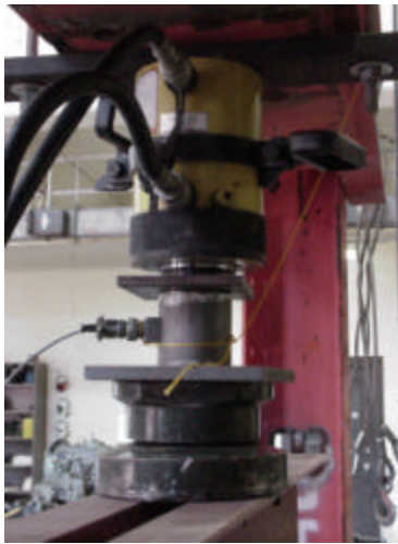
Figure 3.12 Ram and load cell on doubly symmetric channel
