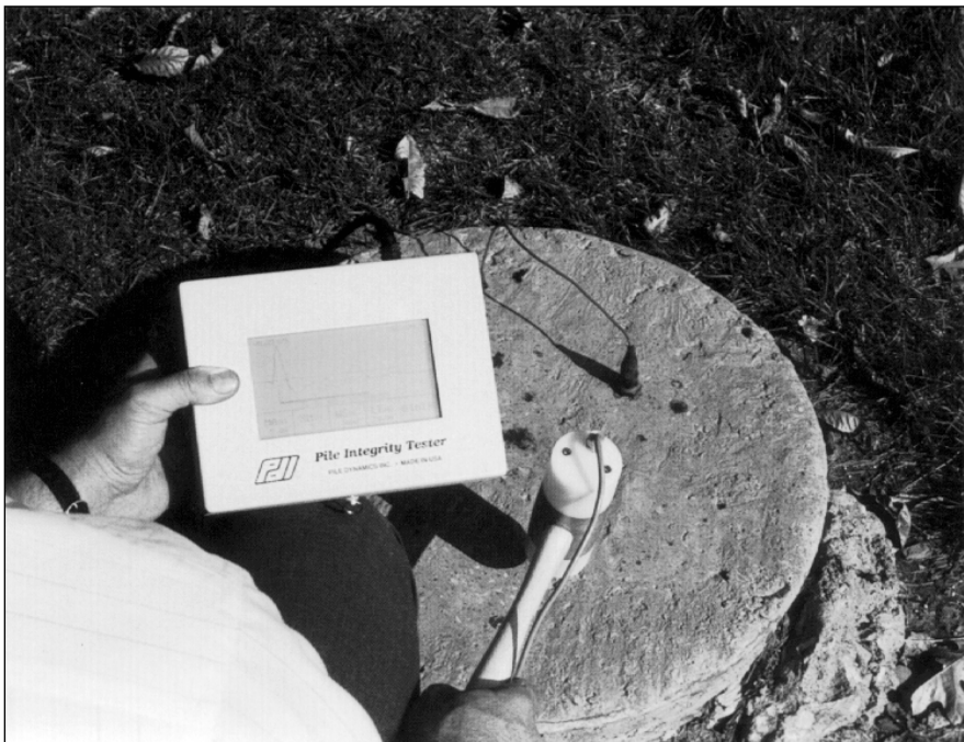
Figure 39, Pile Integrity Tester (After PDI, 1993)
