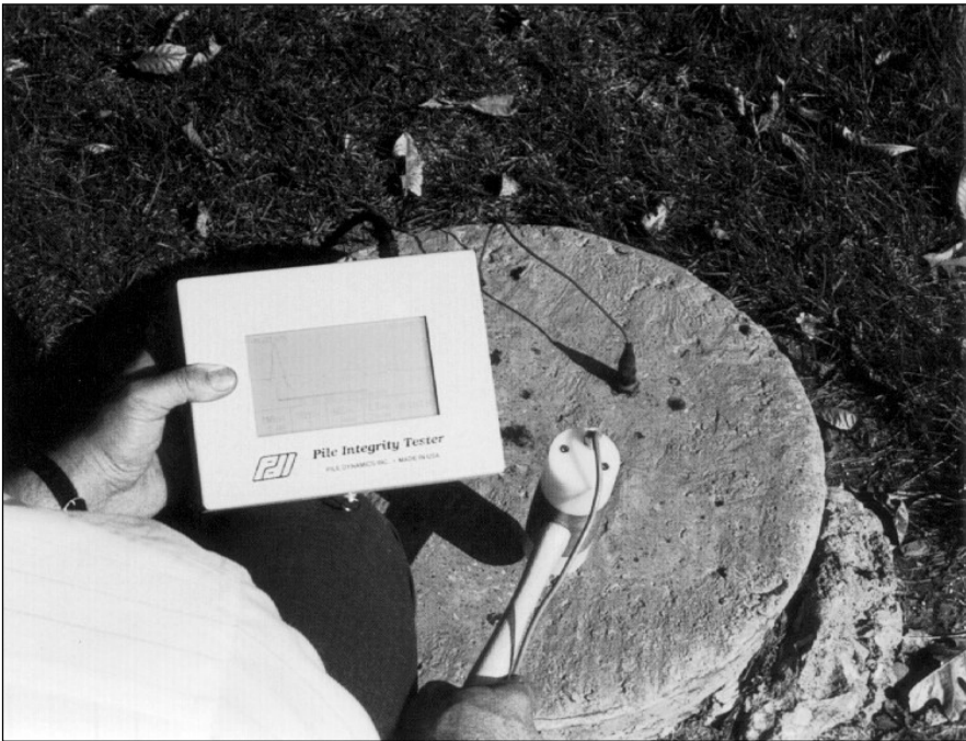
Figure 39, Pile Integrity Tester (After PDI, 1993)
